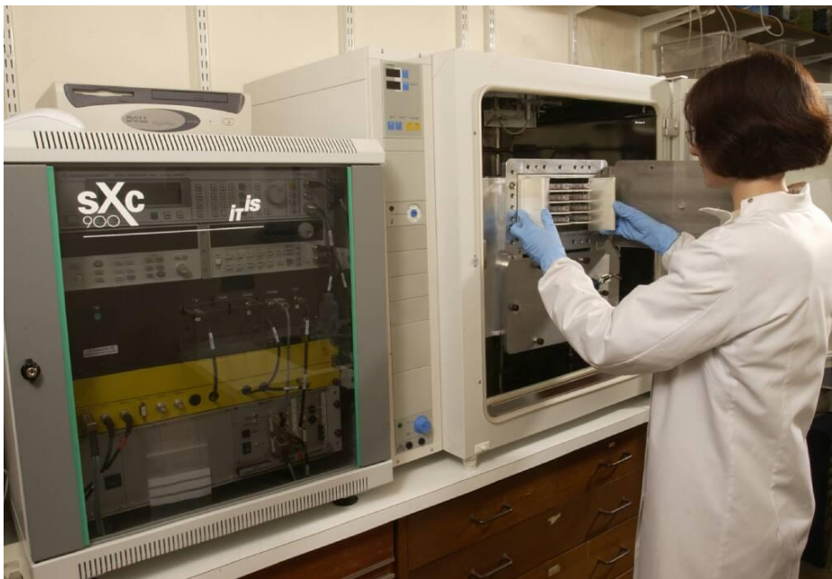
Figure 2.1. The sXc900 exposure system showing the waveguides inside the incubator and the controlling computer.
