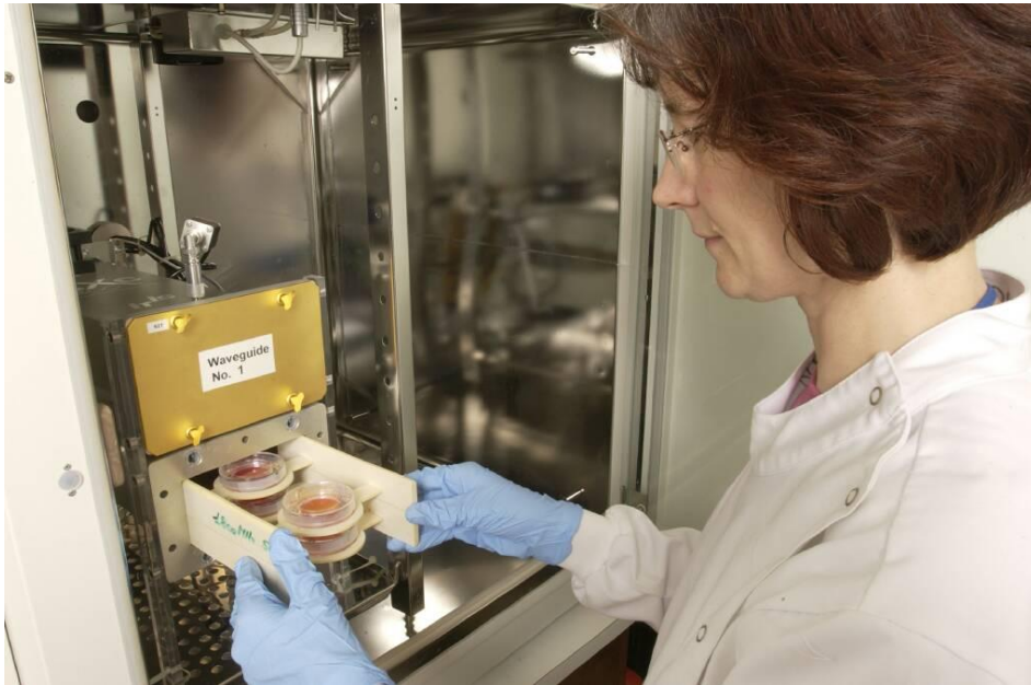
Figure 2.2. The sXc1800 exposure system showing the waveguides inside the incubator.
