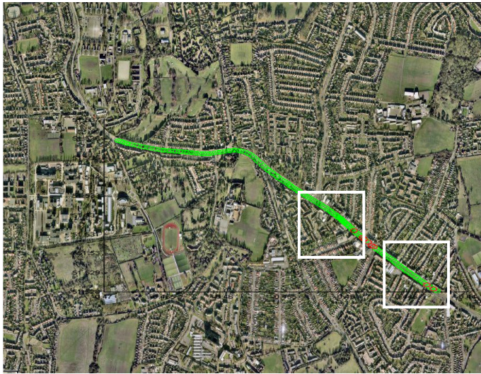
Figure 5-20: Uncorrectable (red marks) and corrected received tables (green marks) tables for MISO reception along Route B.
