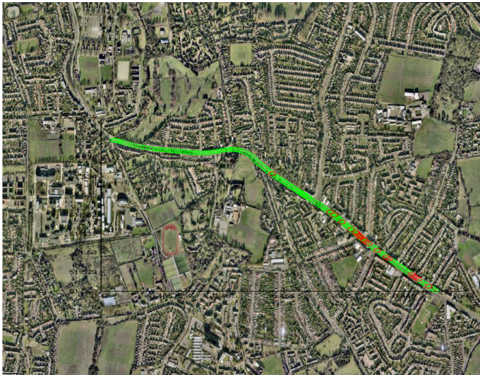
Figure 5-19: Uncorrectable (red marks) and corrected received tables (green marks) tables for SISO reception along Route B.
