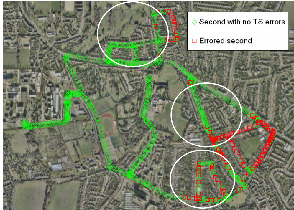
Figure 5-14: Errored and error free seconds vs. geographical position for MISO reception along Route A. It the reduction of errored seconds (marked as red squares) is clear if the zone within the white circles are compared with Figure 5-13
