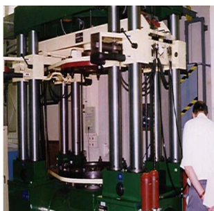
Figure 2.32 LNE torque machine (Davis, 2002).
