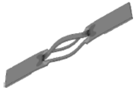
Figure 1b Stress contour plot for the resonator in mode 3.
