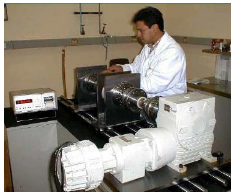
Figure 2.34 2 kNm Torque Transfer Machines (CENAM, 2006).
