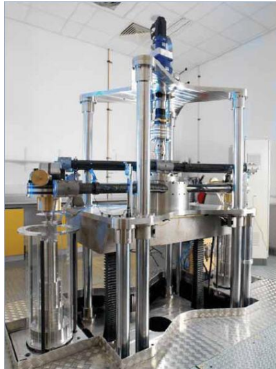
Figure 2.31 NPL torque standard machine (Robinson, 2007).
