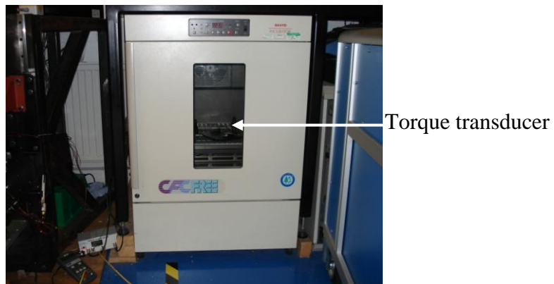
Figure 5.43 Temperature test for torque transducer based on SL20 resonant sensors.
