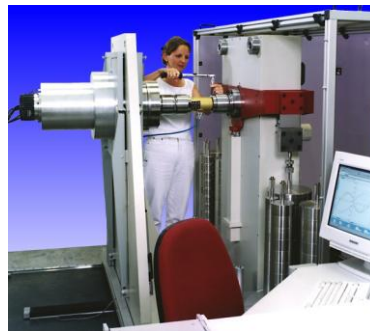
Figure 2.30 PTB 1kNm torque standard machine (PTB, 2009).
