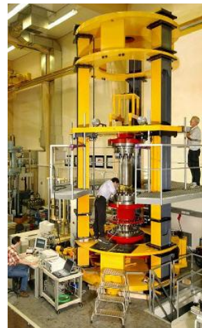
Figure 2.33 The 1.1 MNm torque standard machine of PTB (PTB, 2005).
