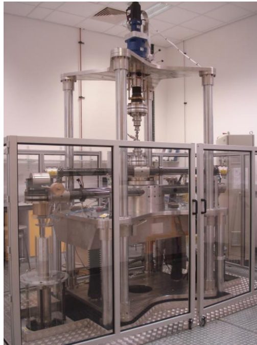
Figure 5.46 NPL Torque Standard Machine (Deadweight Lever-beam).
