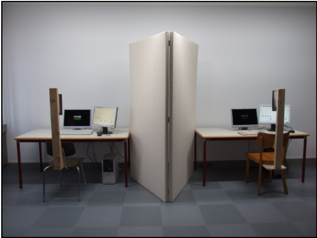
Figure 8-6: Viewing conditions on-site according to ITU-R BT.1788 (Rec. ITU-R BT.1788, 2007).
