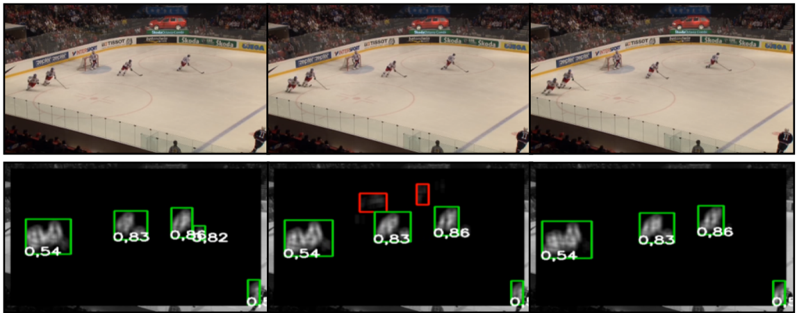
Figure 7-31: Example of filtering ROIs over time by clustering. Red rectangles represent ROIs which cannot be allocated to any cluster and are hence removed from further processing. Green rectangles represent ROIs which are consistent over time. The numbers on each filtered rectangle are the weighting factor w_{total} computed by the classification module (cf. Section 7.3.3).
