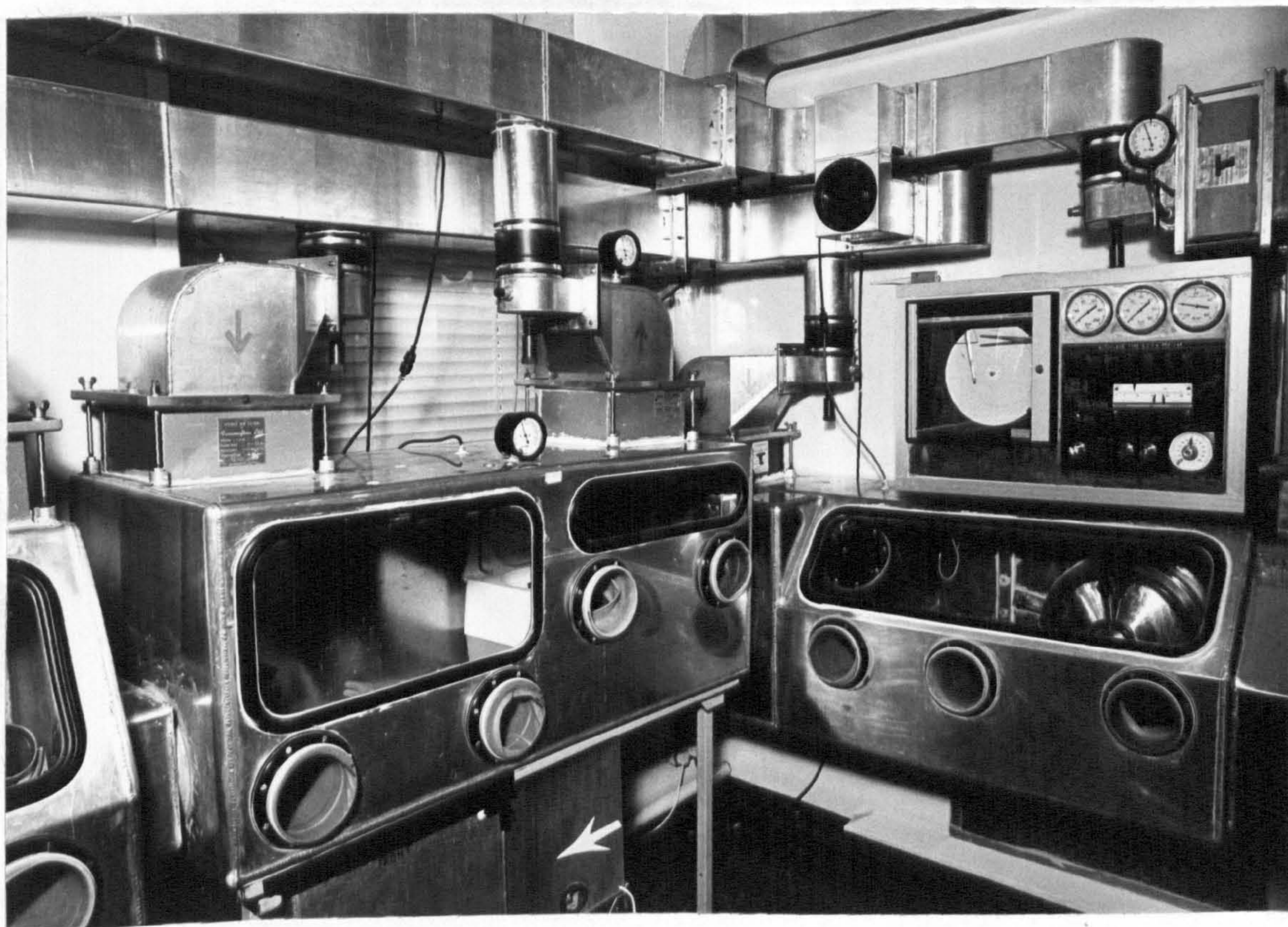
Fig. 6. Cabinets housing +4^{\circ}\text{C} refrigerator ( \blacktriangle ), bench centrifuge and double-ended autoclave.
