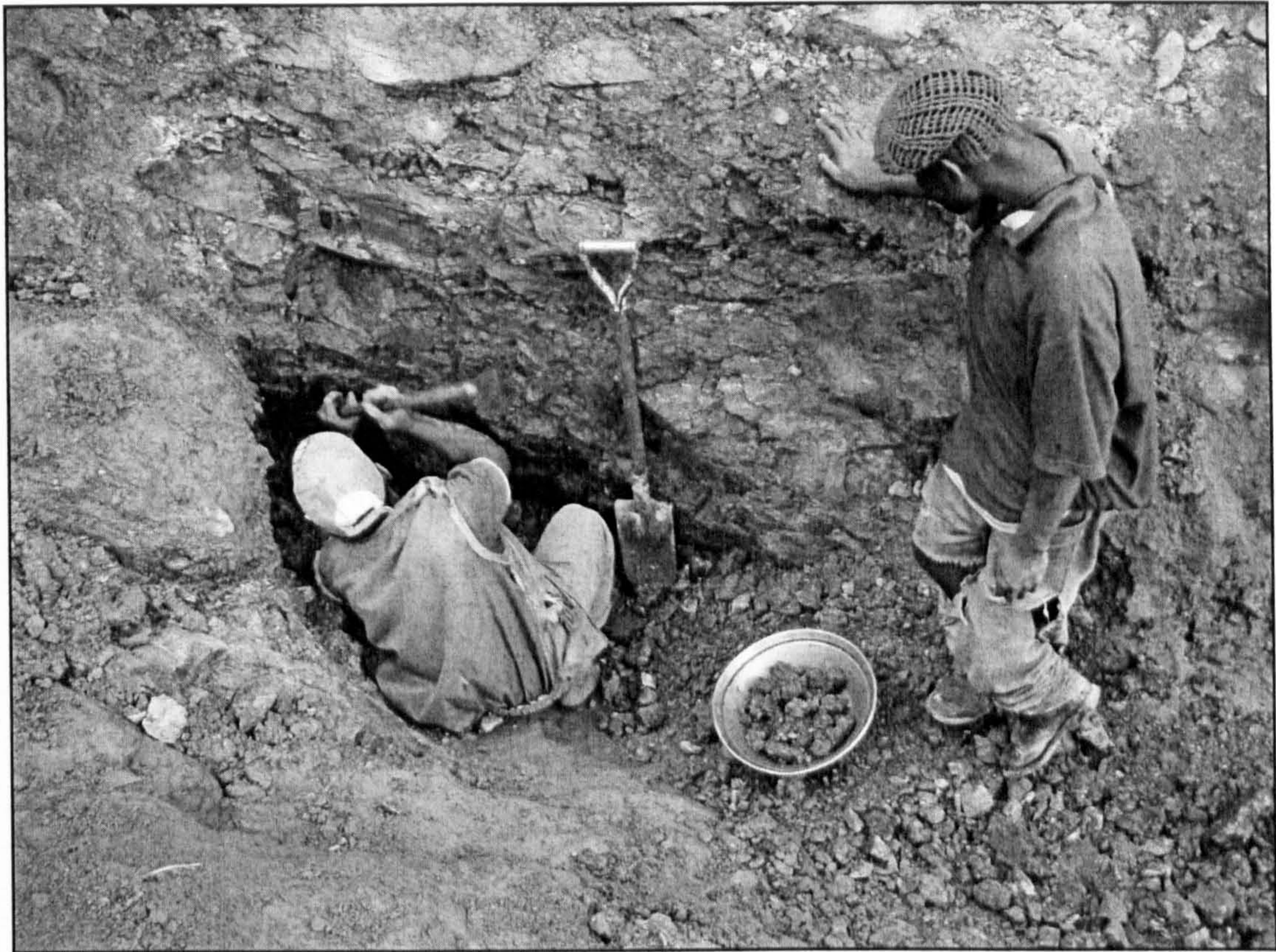
Figure 17. Digging a vein with a kroba .
