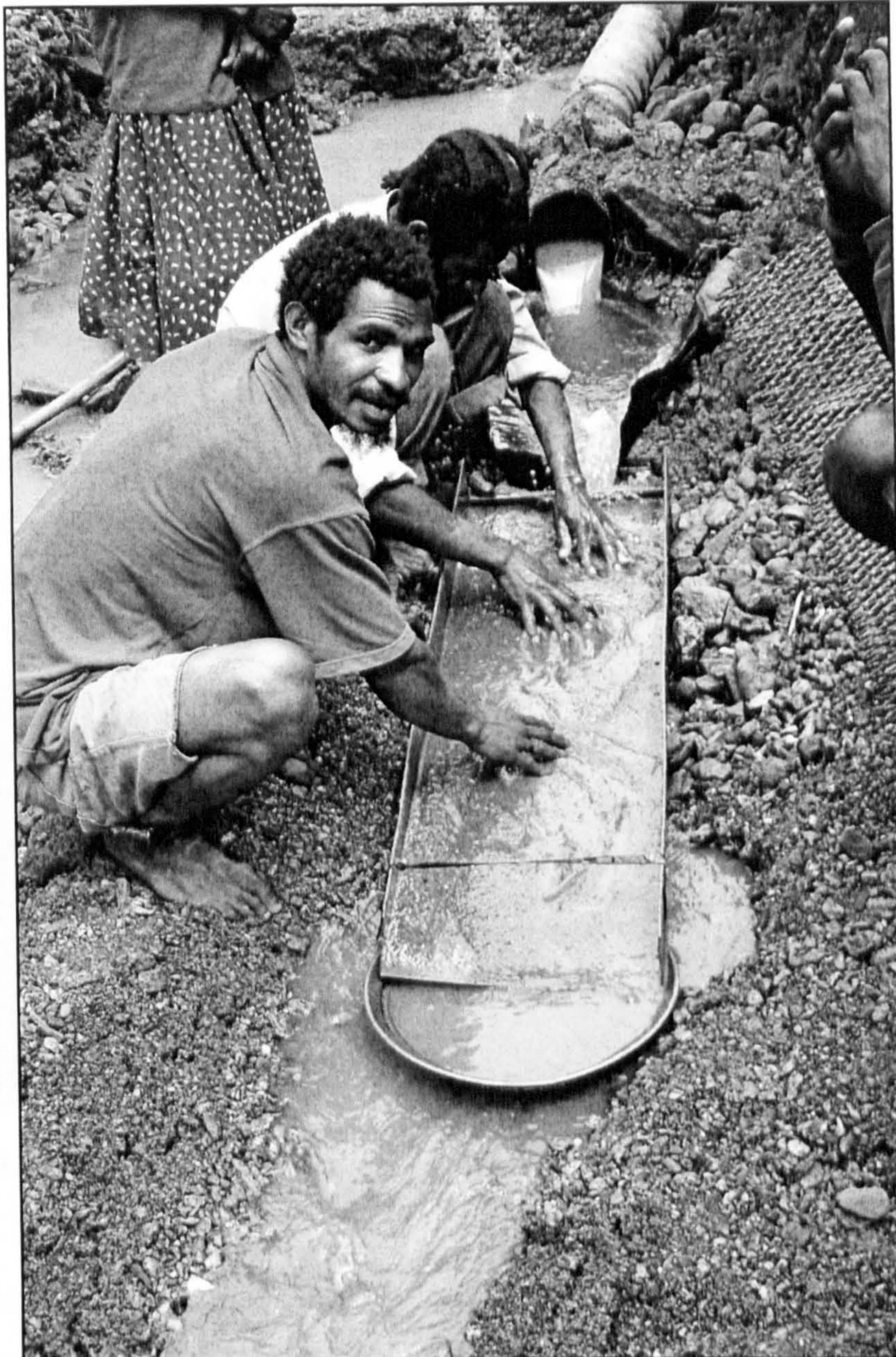
Figure 14. Miners in the process of cleaning a sluice box.
