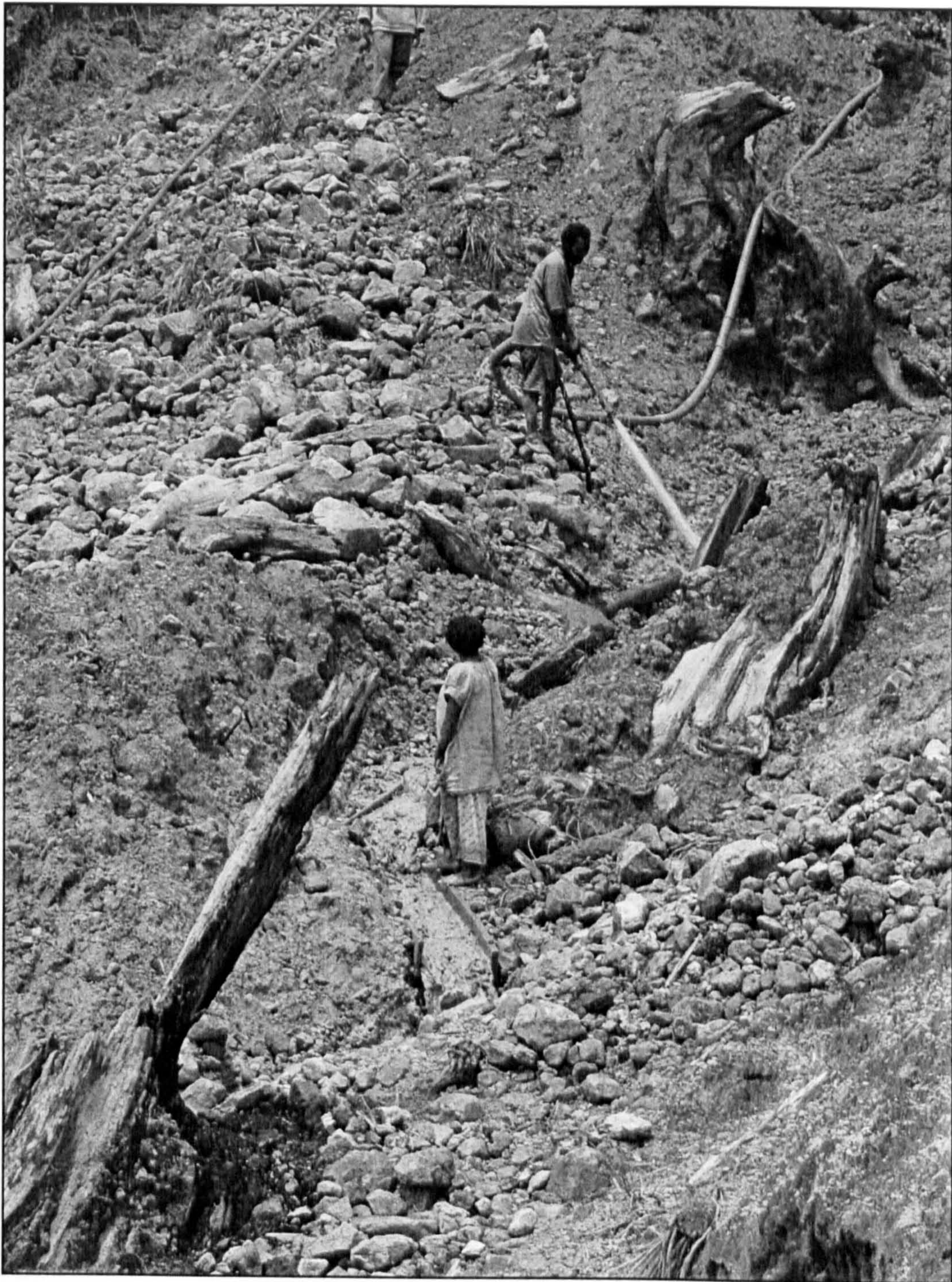
Figure 16. Hydraulic sluicing by means of a masket .
