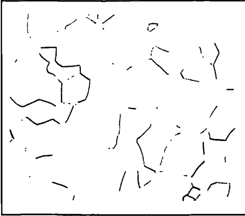
Figure 2.1 High-purity (iodide-process) unalloyed titanium sheet, cold rolled, and annealed 1 hr at 700 °C. Equiaxed, recrystallised grains of \alpha . Kroll's reagent (ASTM192). ( Metals Handbook, Ninth ed., vol. 9, American Society for Metals, Metal Park, Ohio, 1978, p.462. )
