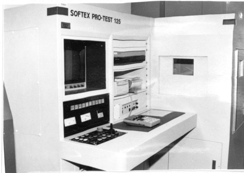
Fig 5 6 SOFTEX x-ray system for void investigations
