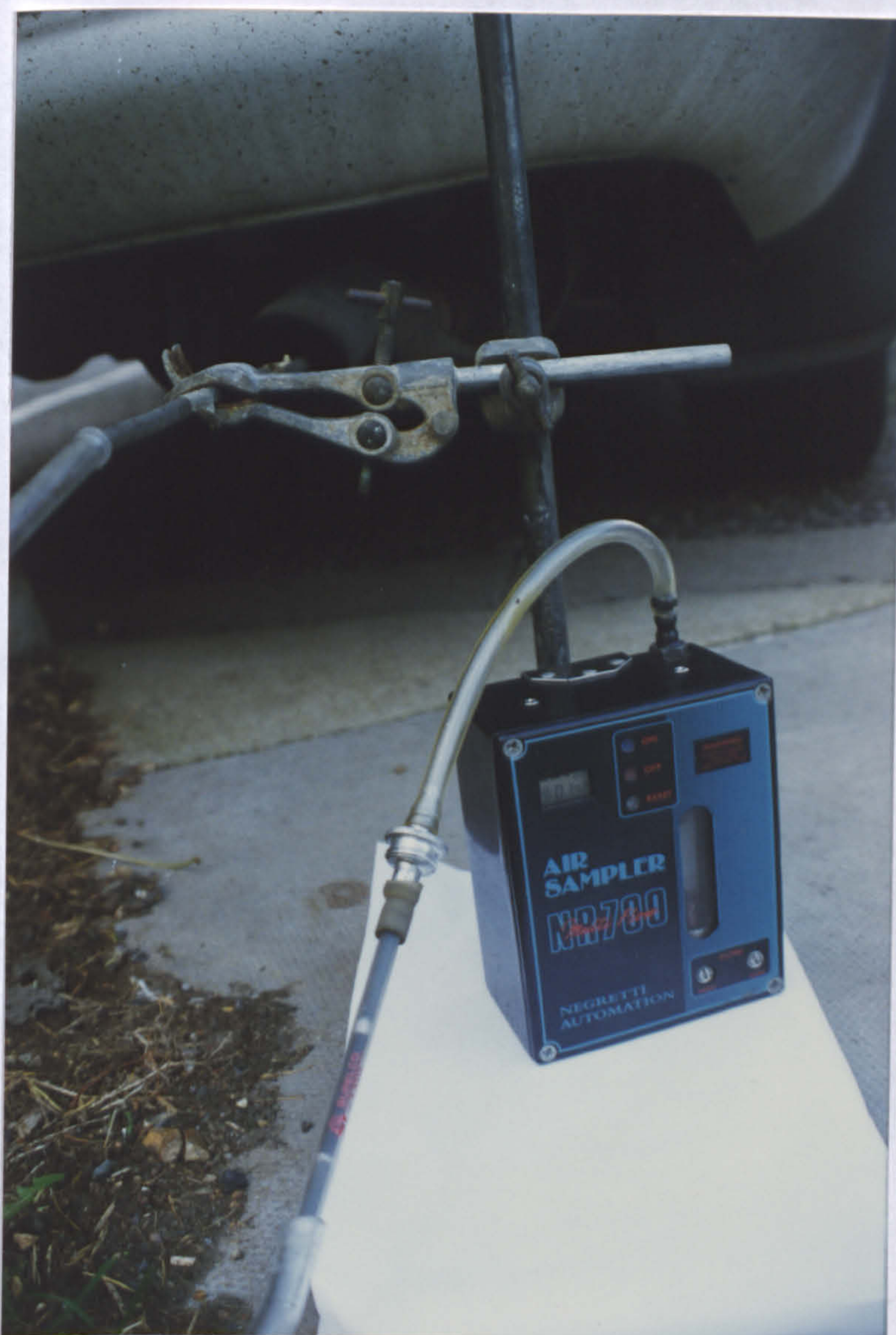
Figure 5.21 Sampling with a small pump from car exhaust
