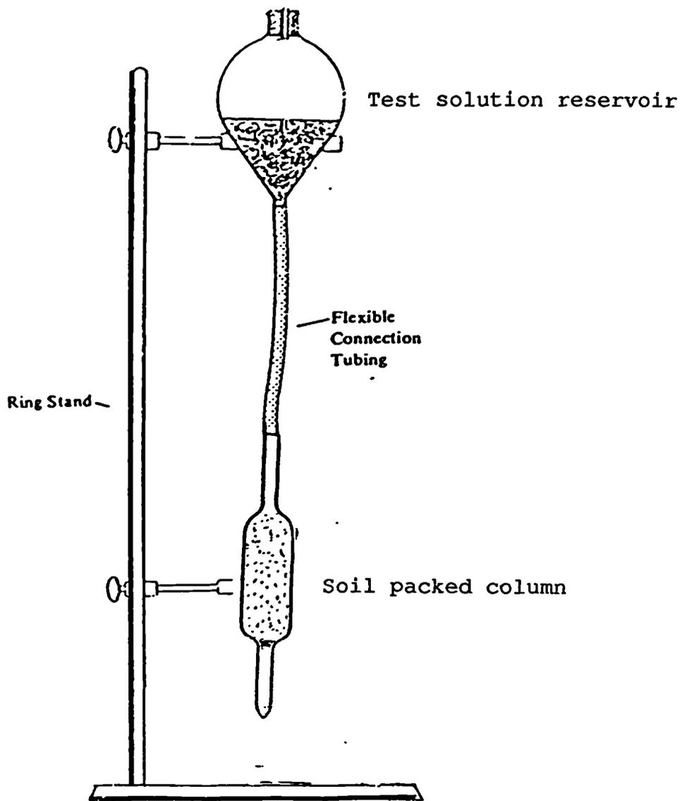
Figure Setting of the apparatus used in dynamic adsorption system
