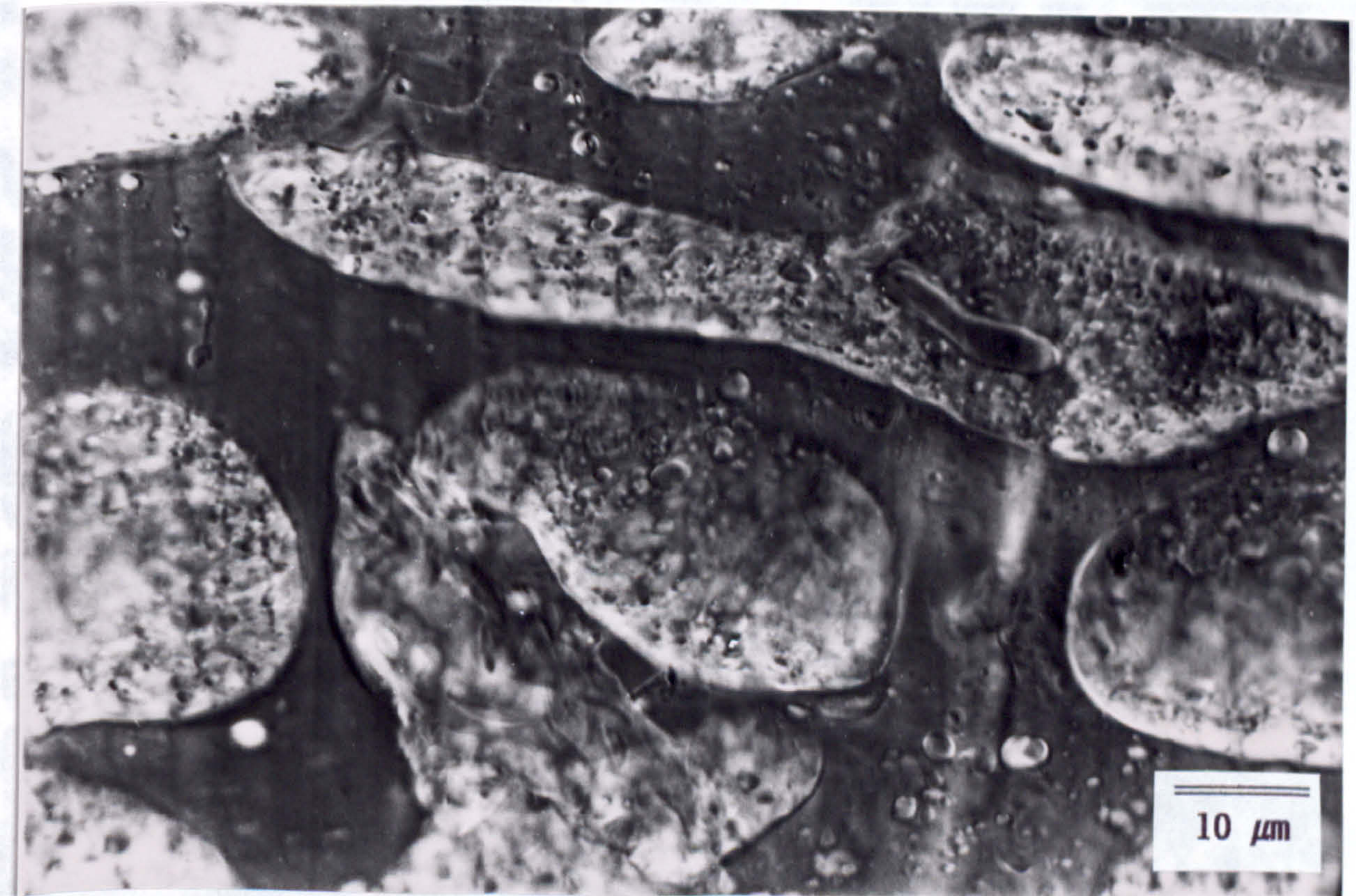
Figure 41 : 60wt% PA6(B5)/40wt% XLPP
