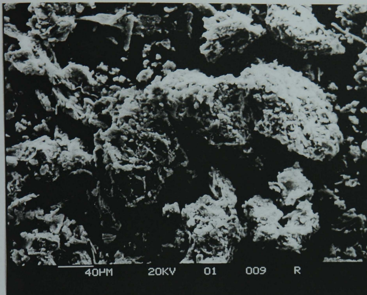
Hydrochloric acid residue
