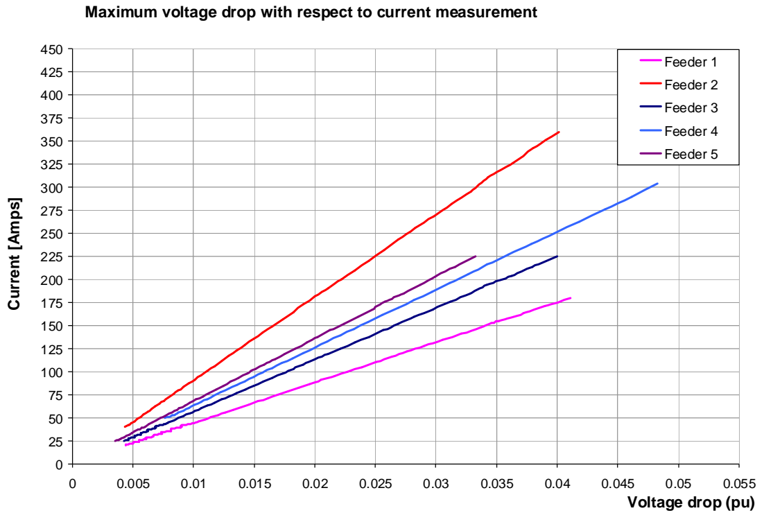
Figure 6.4.2 Relationship of the maximum voltage drop and the feeder current \Delta V_{\max_f}(I_E)
