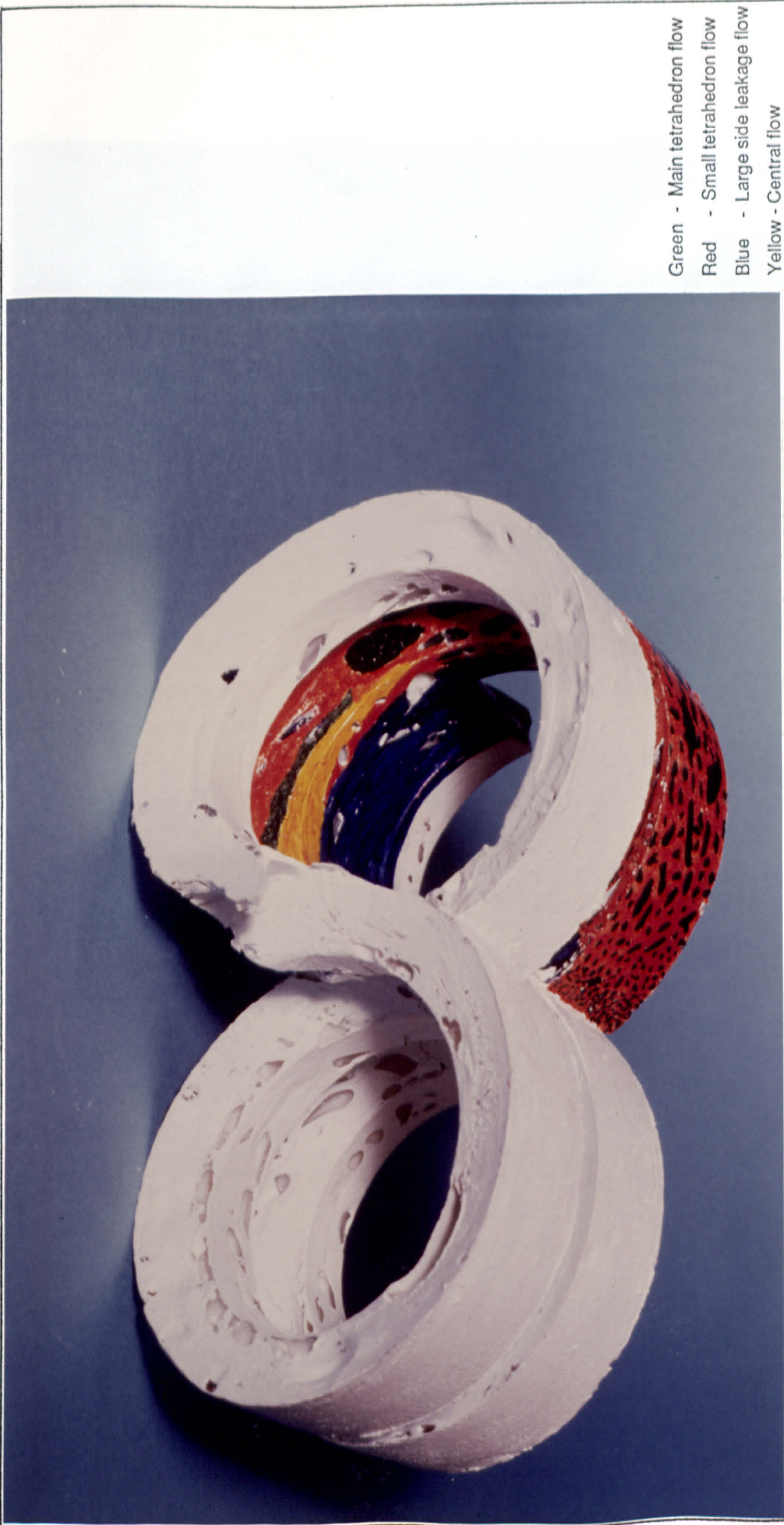
Fig. 4.51 Tentative flow model (photographed from underneath c.f. Fig.4.50 position) showing origin of central flow and large side leakage flow. Also seen is intermixing of tetrahedron flows.
