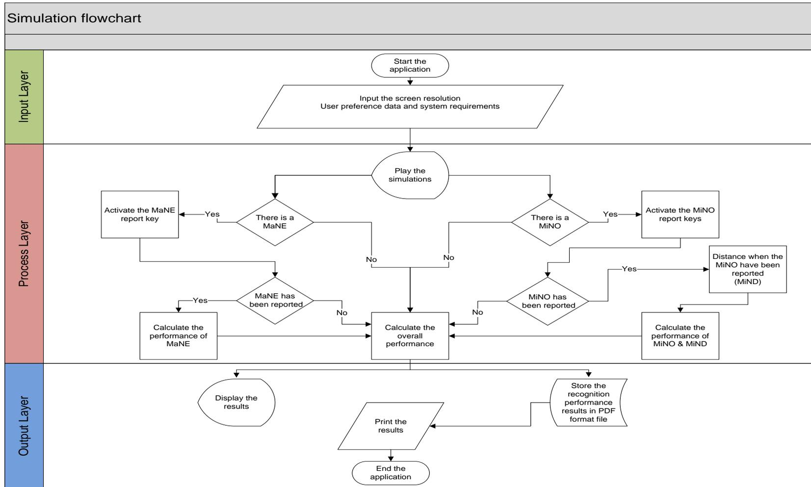
Figure 4. 11 Simulation flowchart
