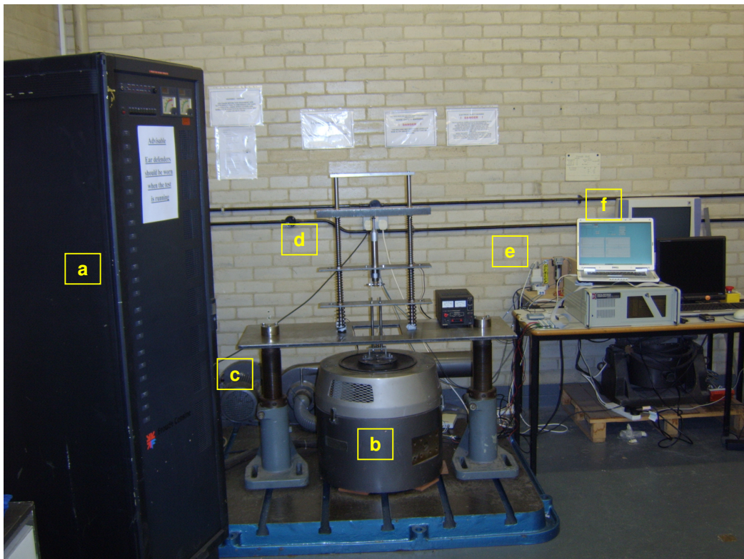
Fig 6.1 instrumentation of the active suspension test rig.
