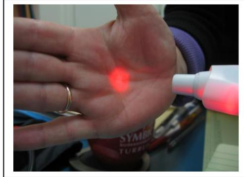
Fig. 2.8 Non-contact infrared Thermometer (cm range). [21]
