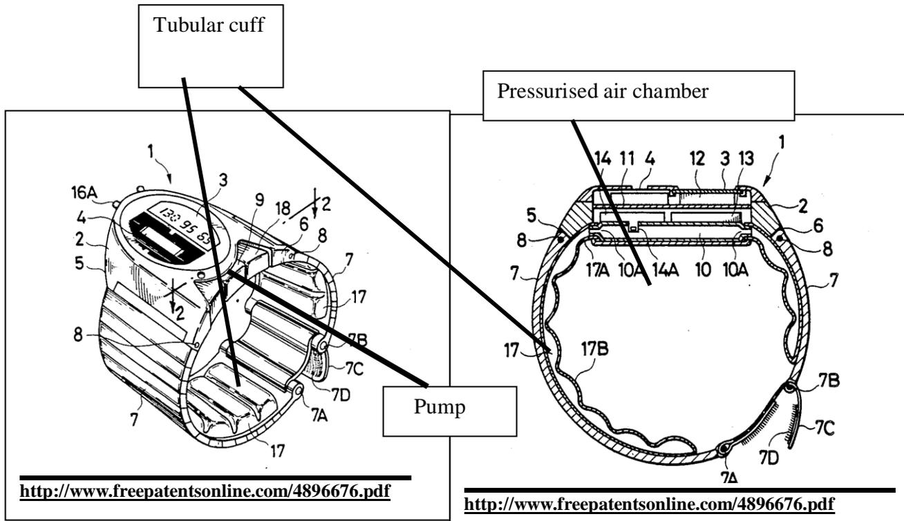
Fig. 4.1 (b) Small Blood-Pressure Watches with a tubular cuff (automatic inflation)
