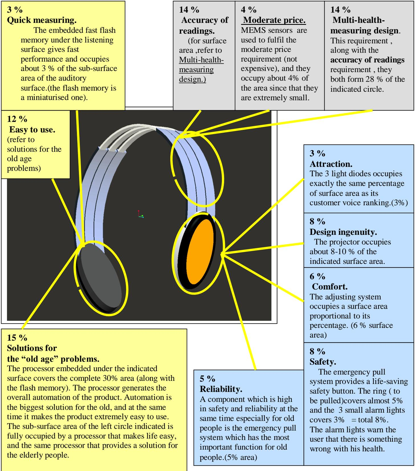
Fig.5.6.3b Dividing the product into portions of variable amounts of feature concentration.
