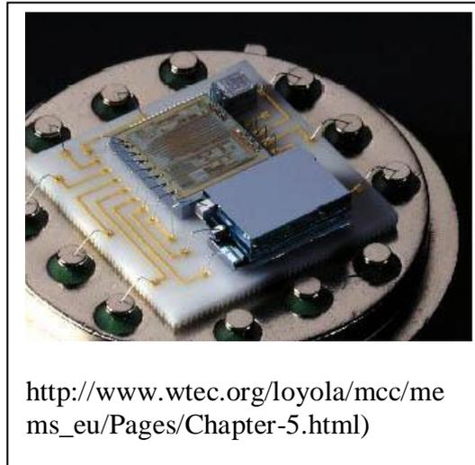
Fig. 2.6.1b CSEM 6100 Accelerometer with interface circuitry. [5], [6]
