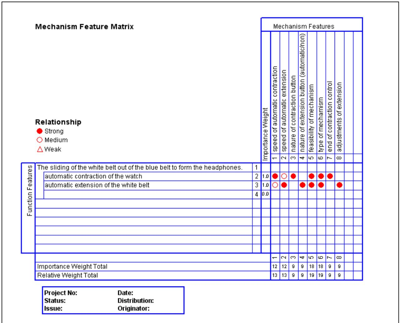
Matrix.3.9d Mechanism Feature Matrix of the white belt component.
