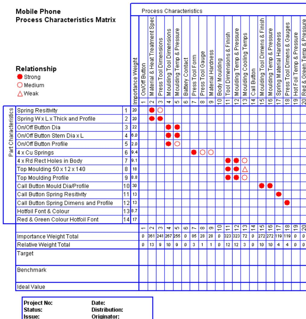
Fig. 2.12.1d QFD matrix (part characteristics vs. process characteristics).
