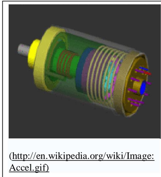
Fig. 2.6.2 A depiction of an accelerometer (MEMS) designed at Sandia National Laboratories.
