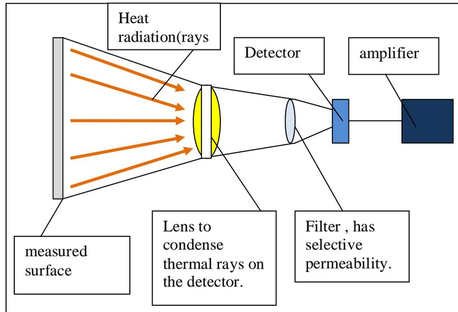
Fig. 5.5.3d MEMS Infrared Thermometer Diagram.[60],[61],[62]
