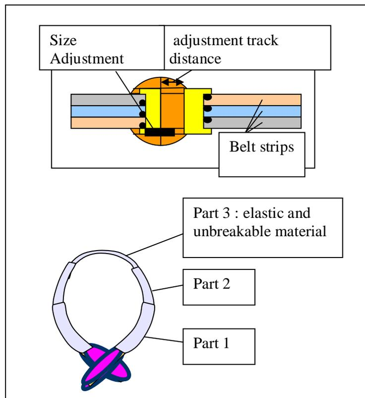
Fig. 5.6.4b watch-EEG conversion components (accepted design solution).
