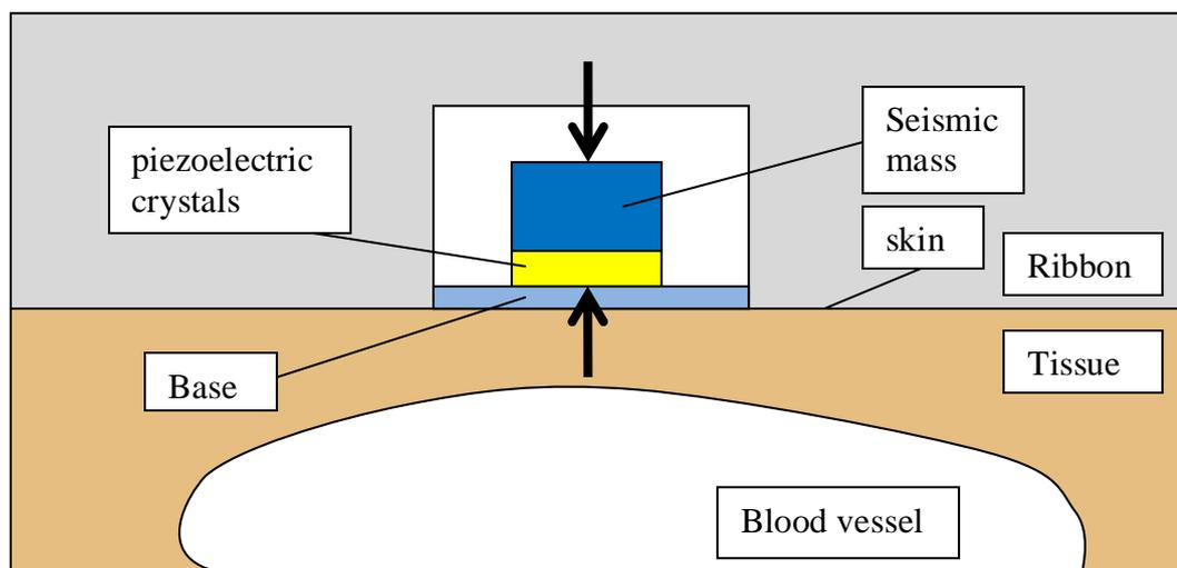
Fig . 5.5.3c Force piezoelectric sensor. [59]
