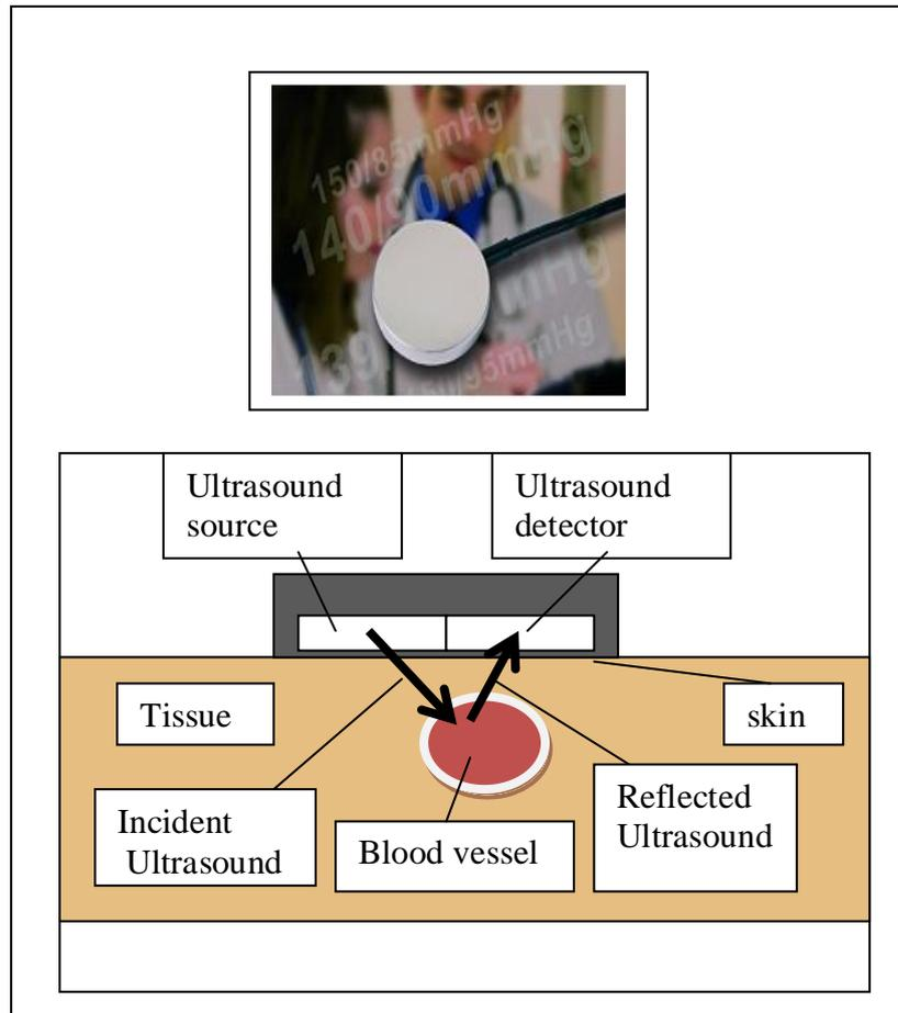
Fig.2.7.1b Diagram and photo of Ultrasonic blood pressure sensor. [11]
