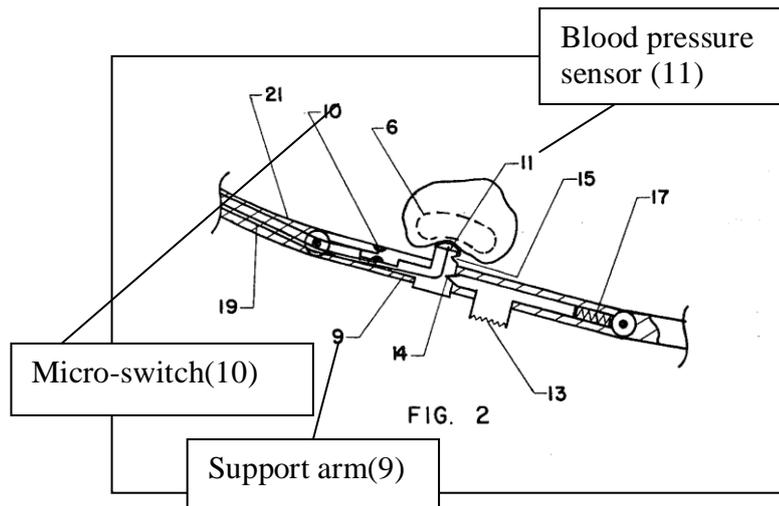
Fig. 2.4.b Advanced contact BP sensory system.
