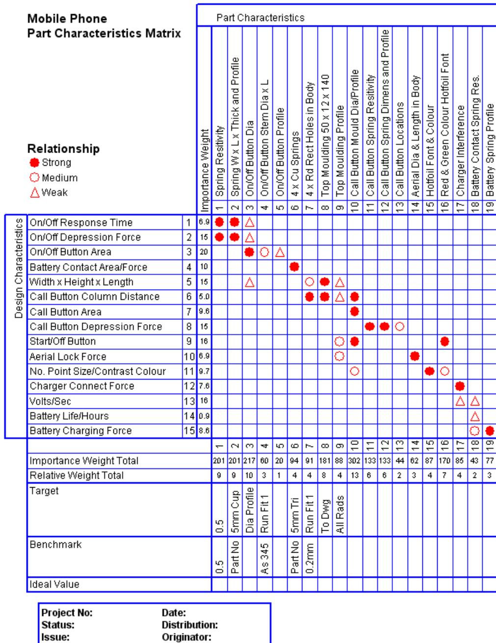
Fig. 2.12.1c QFD matrix (design characteristics vs. part characteristics).
