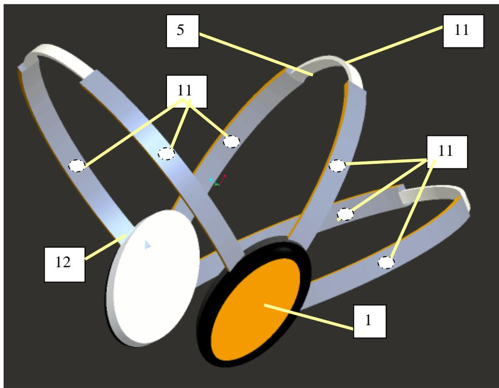
Fig. 6.1e Watch electrode-antennas are separated(proEngineer)
