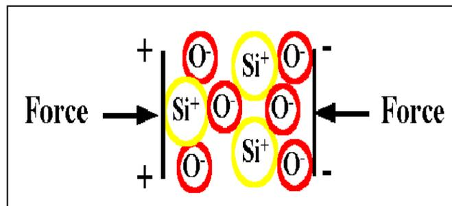
Fig. 2.6.3c Rearrangement of charged particles.
