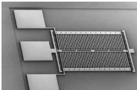
Fig. 5.4.3a Micro accelerometer.
