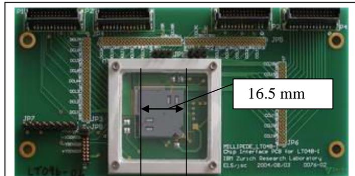
Fig. 6.5c An IBM developed Millipede storage device. (16.5 mm × 17.5 mm × 1.2mm) [71]
