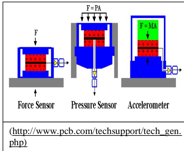
Fig.2.6.3d Types of piezoelectric sensors. [9]
