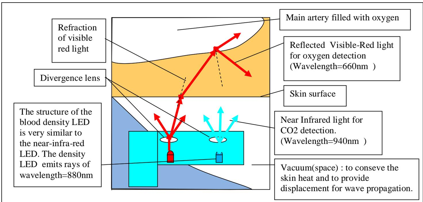
Fig. 5.5.3e Oxygen/CO2 sensor (width = 3mm). [64]
