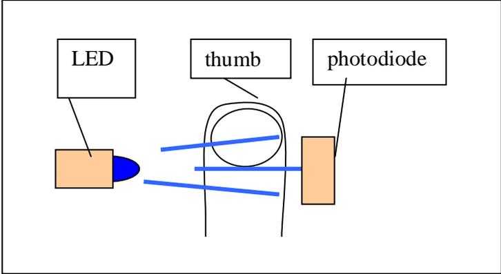
Fig. 2.8.2 Direct infrared probing method.
