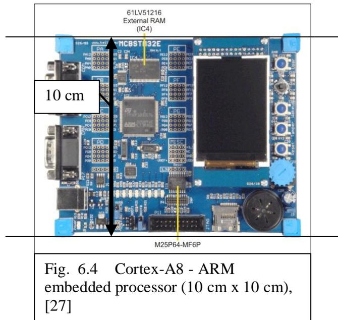
Fig. 6.4 Cortex-A8 - ARM embedded processor (10 cm x 10 cm), [27]
