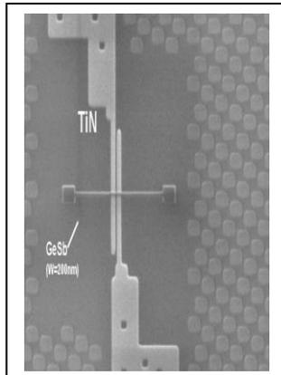
Fig. 6.5a Phase Change Memory Technology (500nm x 500nm): [69]
