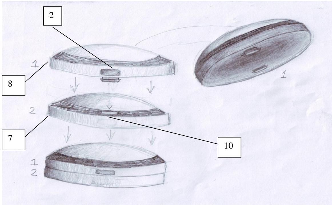
Fig. 6.1c Watch upper body release (2 halves).
