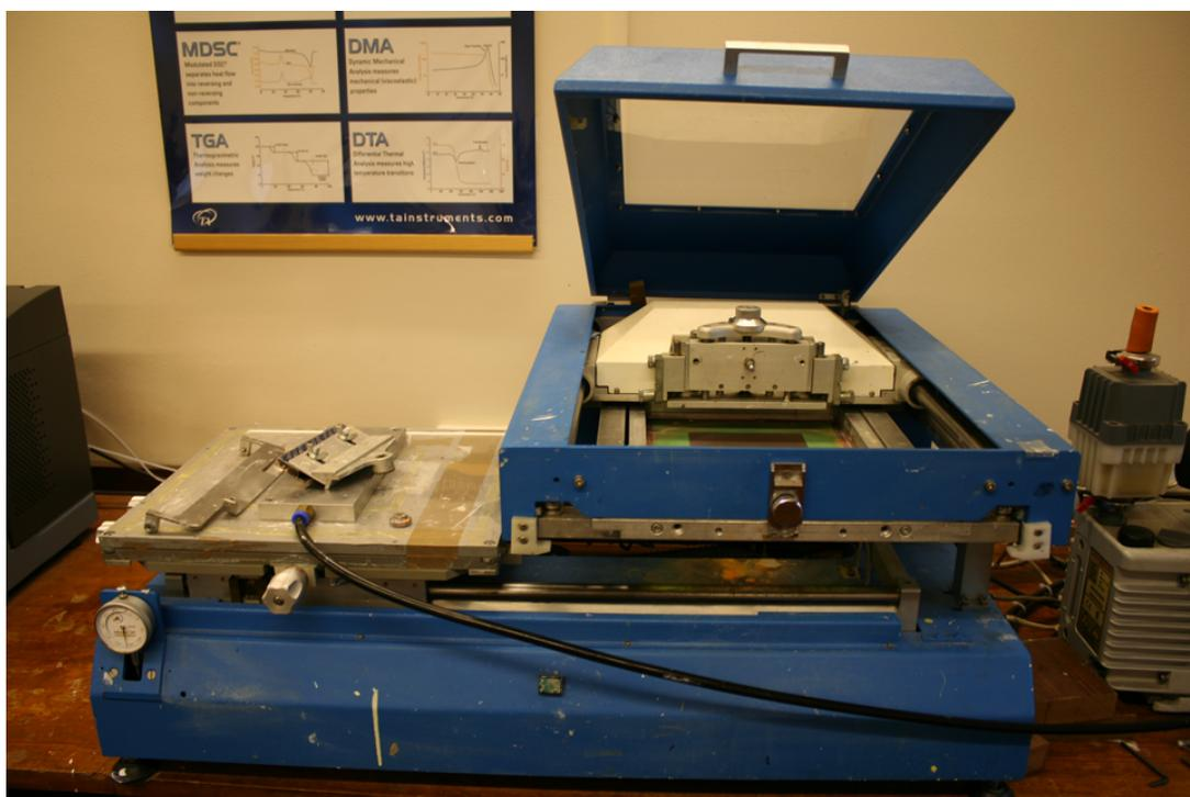
Figure 2.6: DEK 247 screen printer
