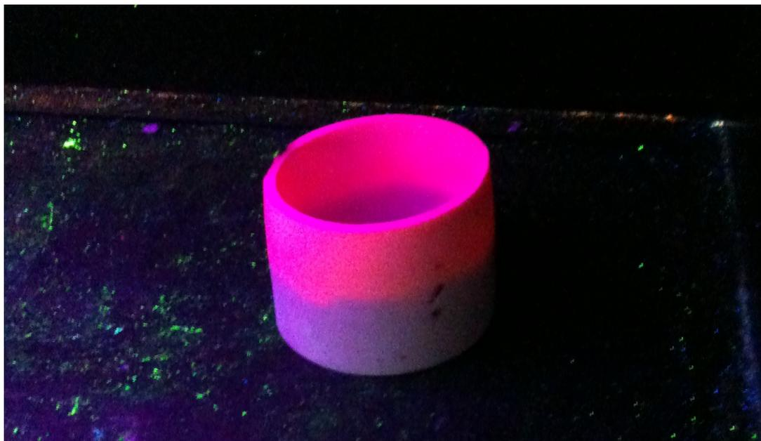
Figure 5.1: Image taken showing the cross section of the crucible under 366nm UV radiation where europium has infused into its structure
