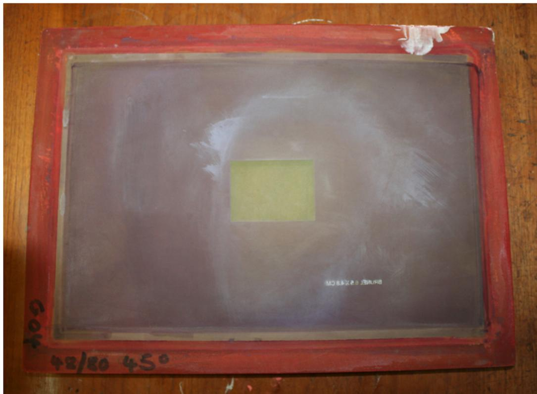
Figure 2.7: Typical screen used with screen printer. Printable area in centre (yellow) is of size 65mm x 48mm
