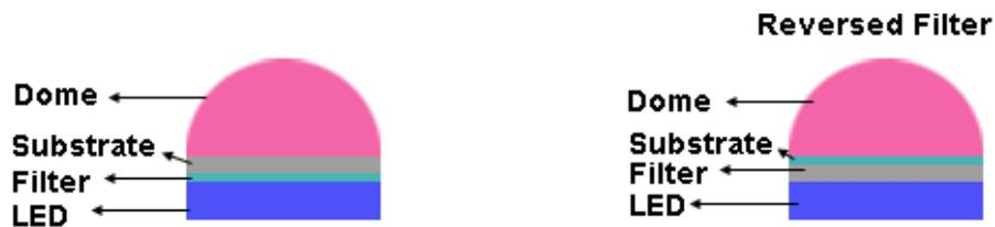
Figure 7.30: Schematic showing the order of the filter and architecture as described in the text
