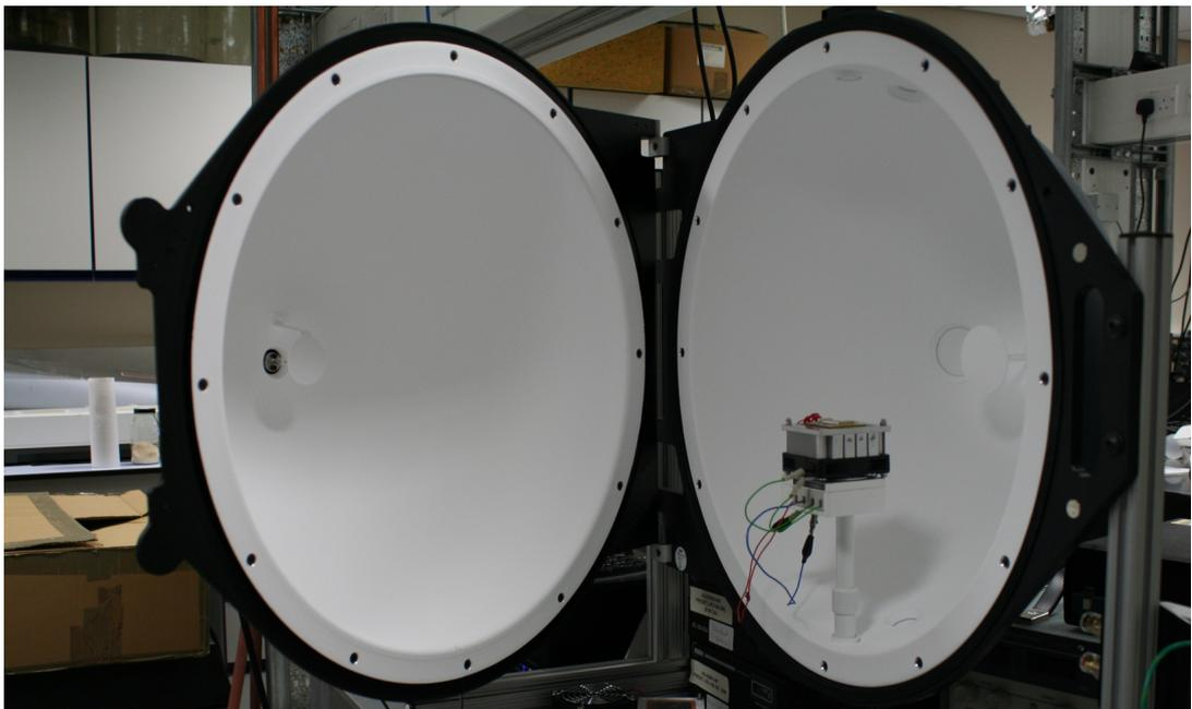
Figure 2.2: Pro-Lite Integrating Sphere
