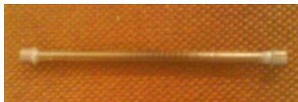
Fig: 4.7. Roll wrapped carbon fibre composite with mild steel plugs at both ends. It is important to note that the plugs are held in place by some adhesive.
