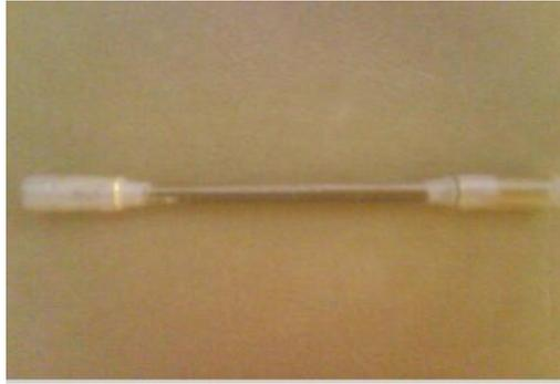
Fig: 4.22. The tubular sample with longer plugs and more adhesive covering more length in and out of the tube.
