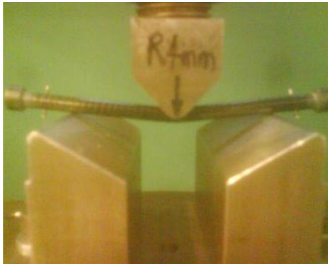
Fig: 4.20. The sample is under some load is visibly deflecting.
