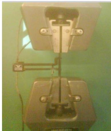
Fig: 4.23. The V grips- the fixture that secured the tubular test sample in place. The inner sections have V grooves that ensure better gripping of the sample. See attached also the extensometer.
