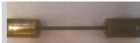
Fig: 4.8. The sample fitted with grips at both ends. The grips are actually split collars that are kept in place by slip rings and unthreaded bolts. See the holes for the bolts.
