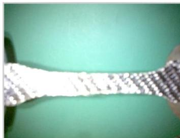
Fig: 4.34a. Picture of the poorly made dumbbell strip with aluminium tabs
