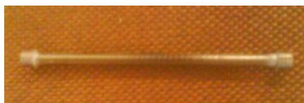
Fig: 4.7. Roll wrapped carbon fibre composite with mild steel plugs at both ends. It is important to note that the plugs are held in place by some adhesive.
