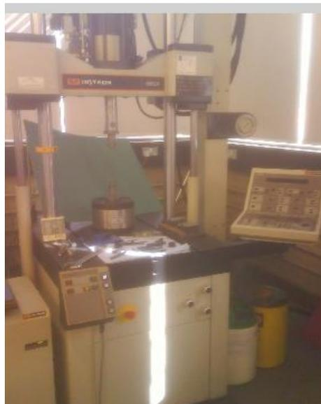
Fig: 3.1. Instron series 9 test rig.
