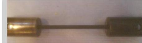
Fig: 4.8. The sample fitted with grips at both ends. The grips are actually split collars that are kept in place by slip rings and unthreaded bolts. See the holes for the bolts.
