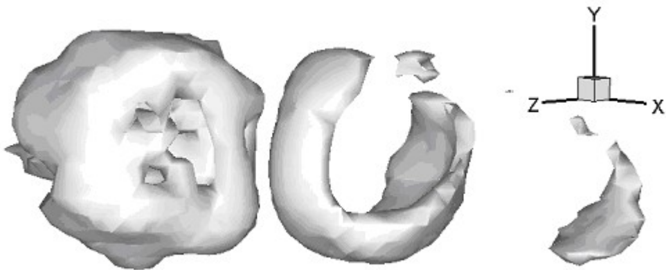
Fig. 6.1(f) Magnification of the vortex rings present with an enstrophy value of 0.5.
