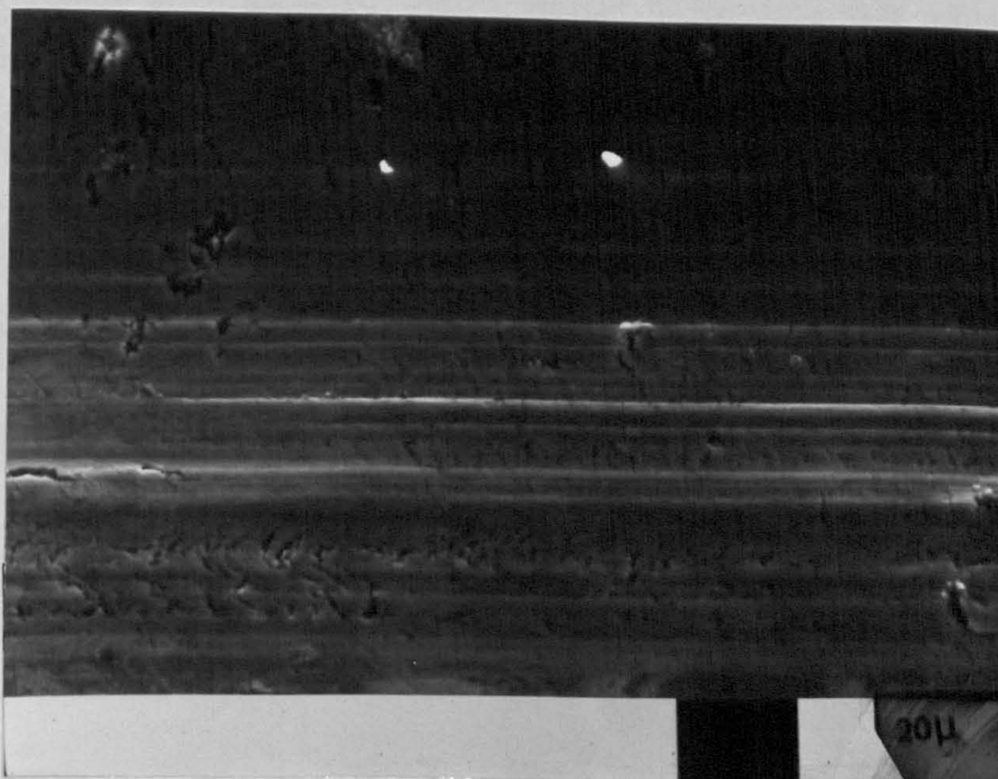
Fig. 98b. Bottom track of steam treated (Fe) after 1000 cm sliding distance under 3 Kgs load. D = 6.8 \text{ g/cc} x 1K
