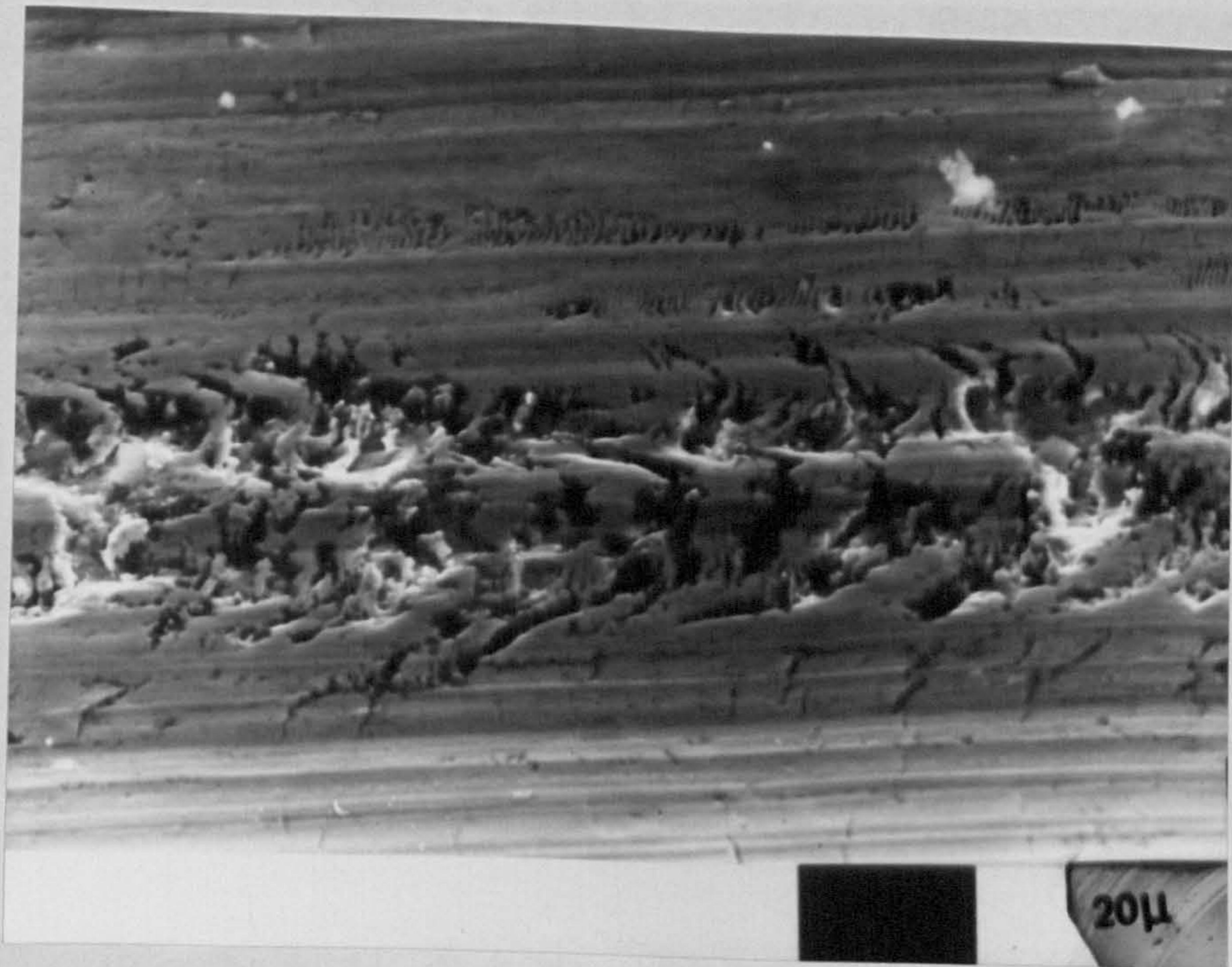
Fig. 96b. Bottom of track in steam treated (Fe + 4% Cu) after 1000 cm sliding distance under 5 Kgs load.
