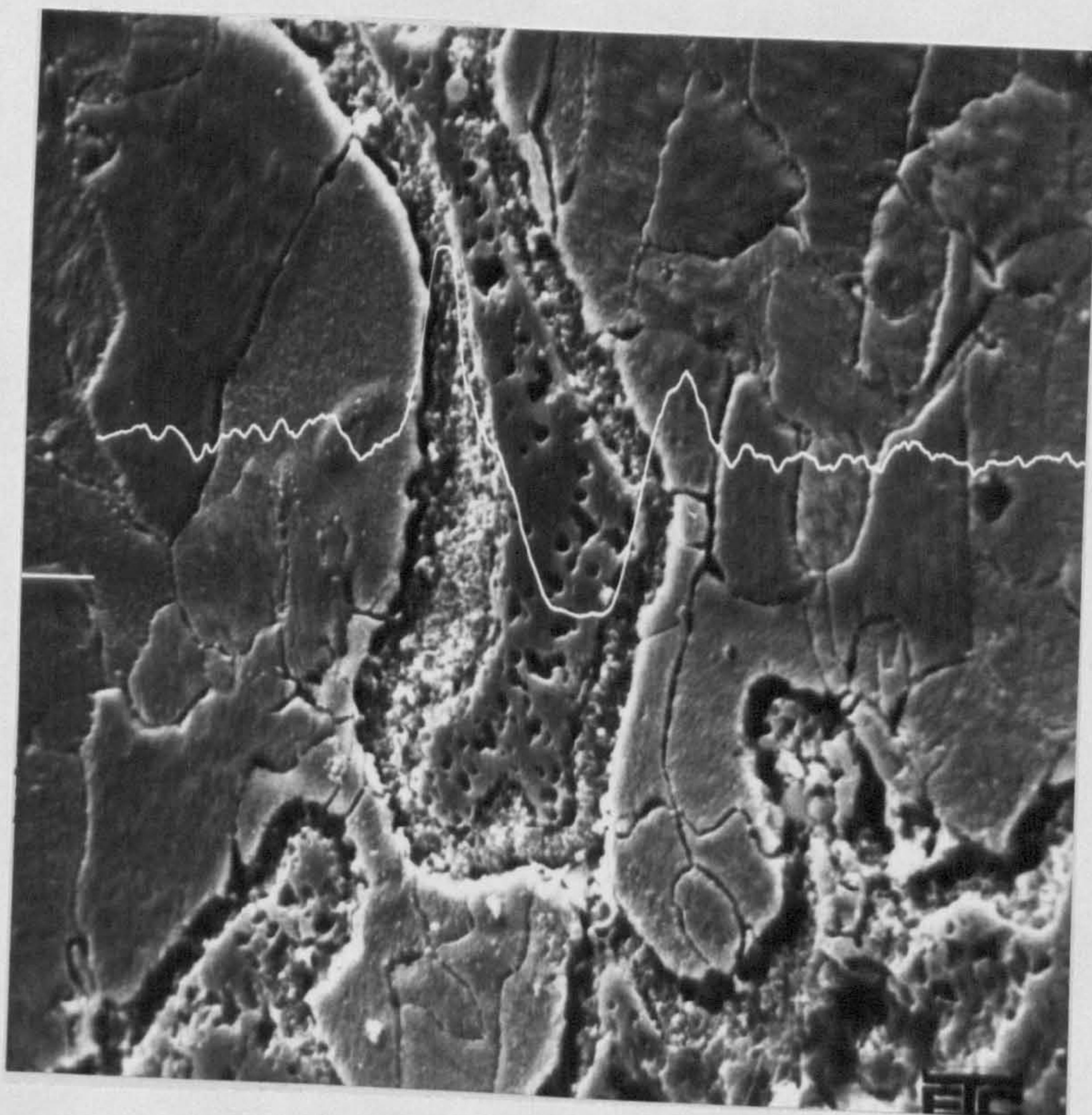
Fig. 67. - 100 # Pre-alloyed (Fe + 4% Cu) D = 6.0 \text{ g/cc} (W.Q.) Steam treated (100 minutes (525° C) x 2K Cu Line Probe
