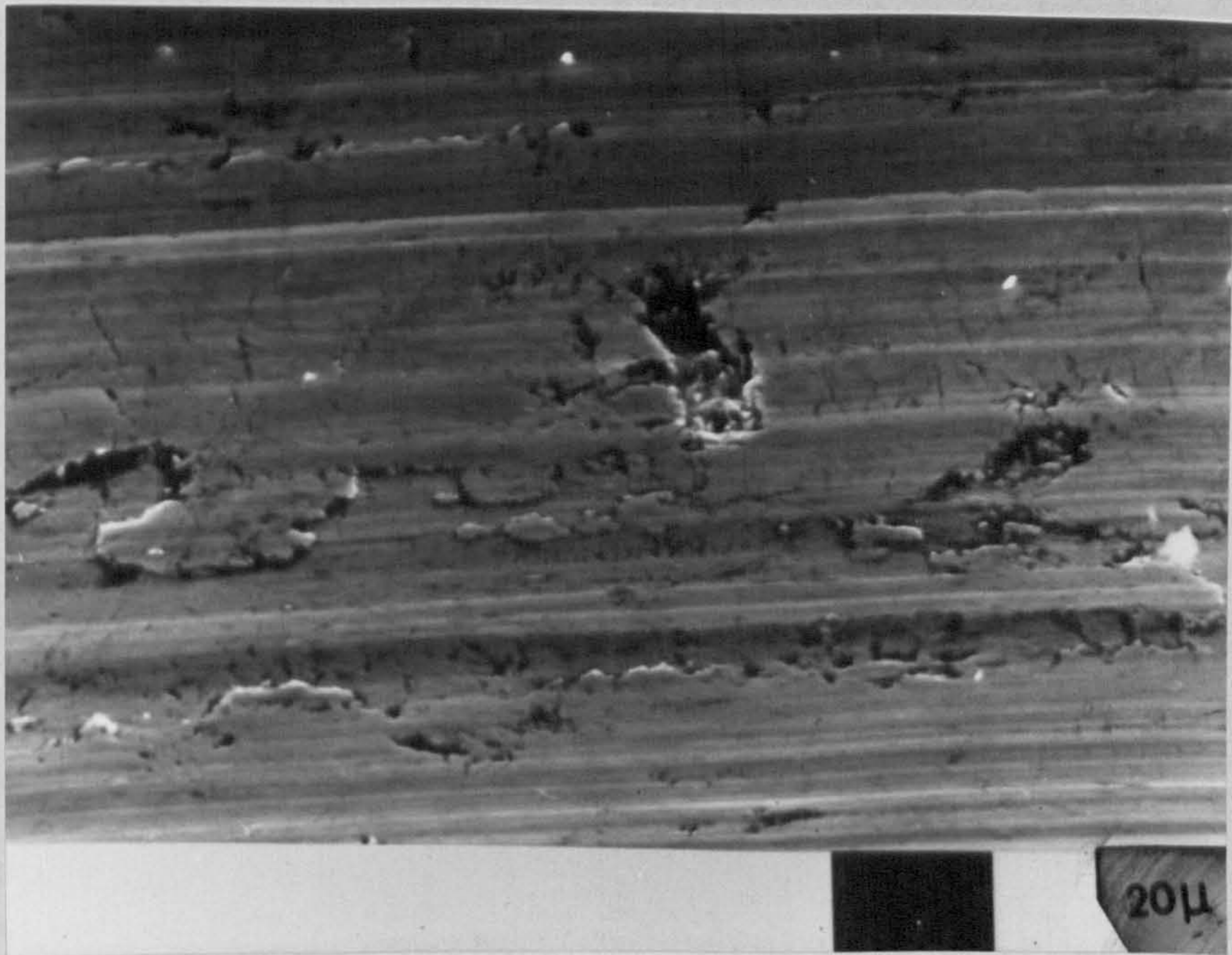
Fig. 101b. Bottom of track in steam treated (Fe + 6% Cu) after 1000 cm sliding distance under 5 Kgs load.
