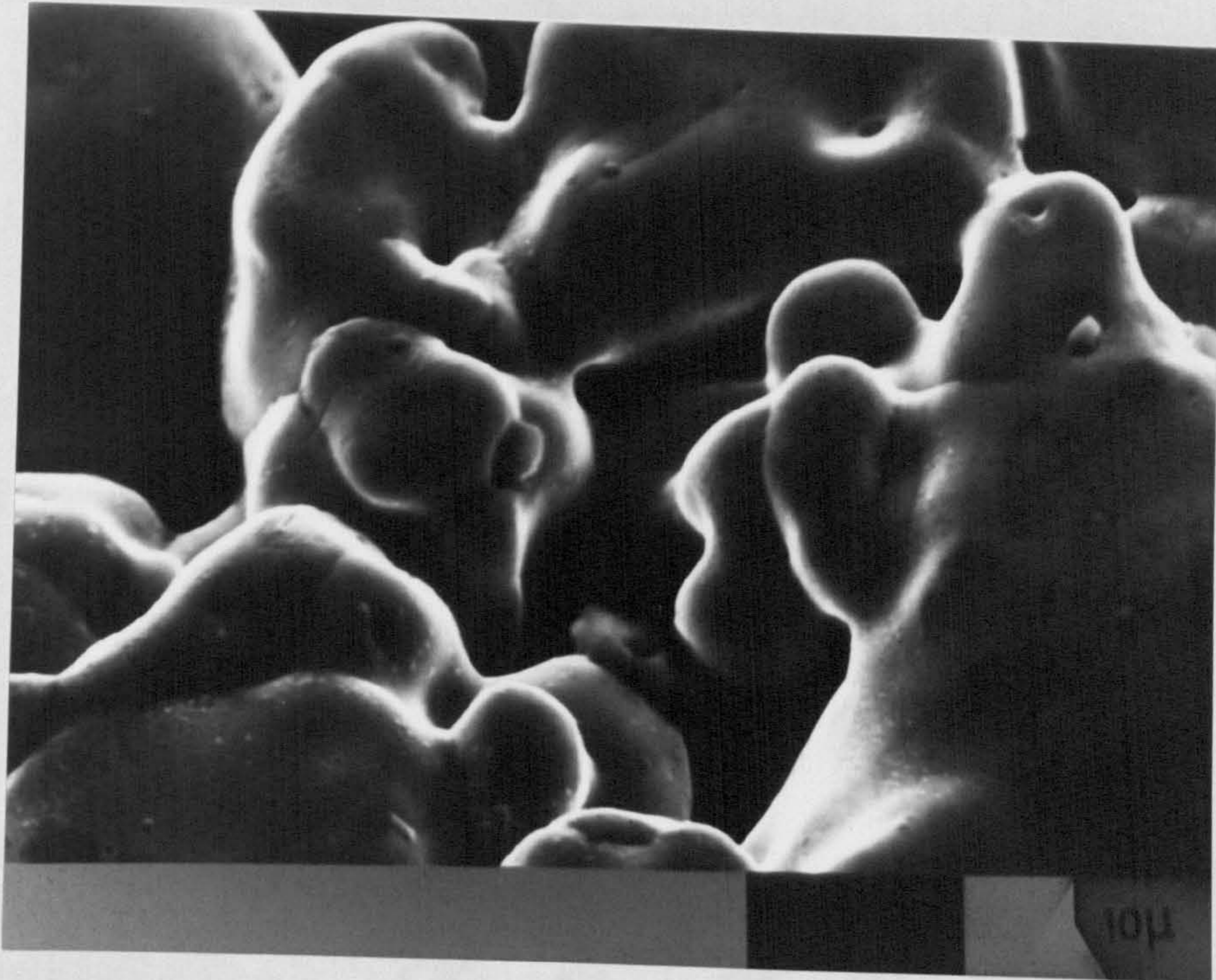
Fig. 42. - 100 # Pre-alloyed (Fe + 8% Cu) D = 6.4 g/cc (sintered) x 2K
