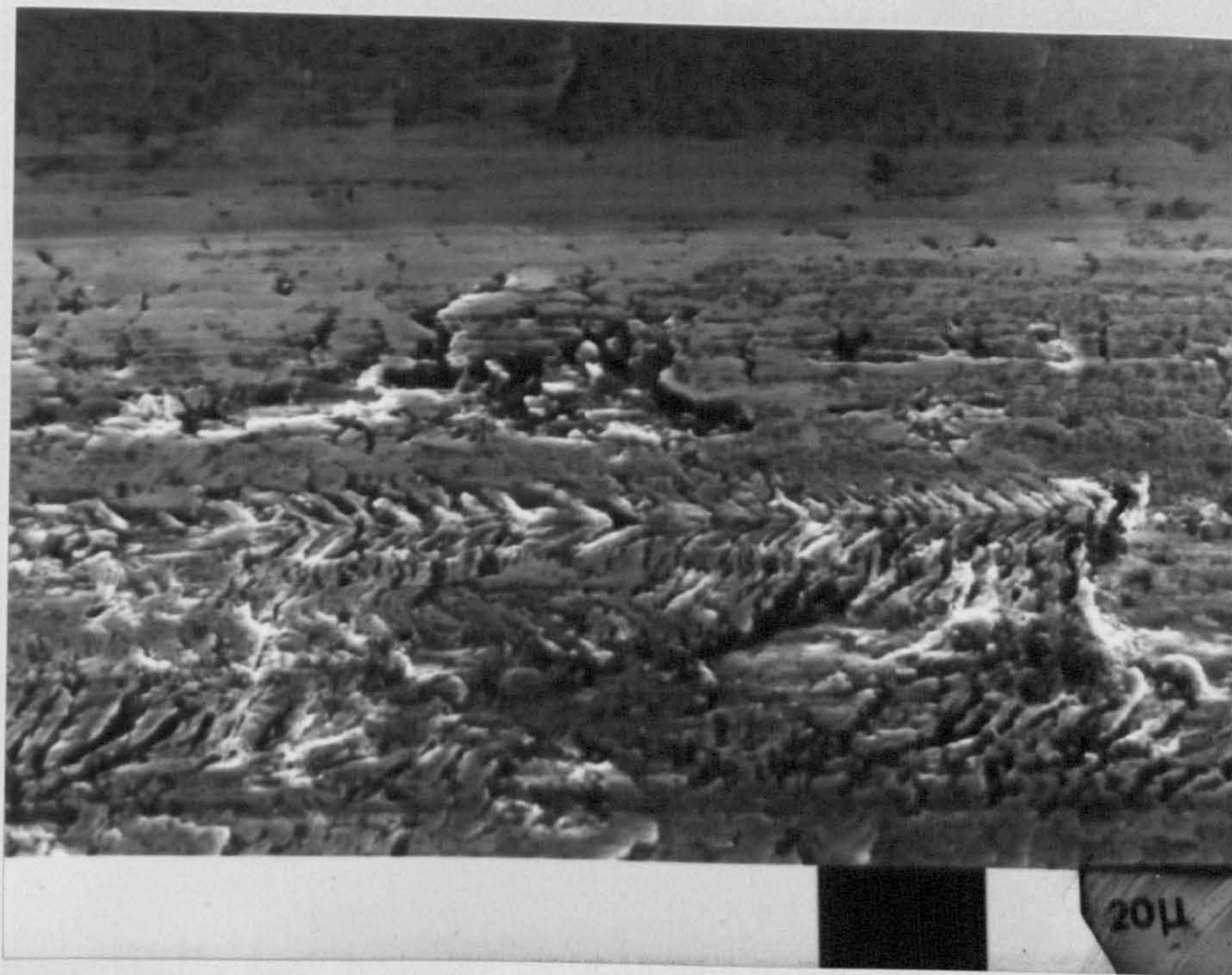
Fig. 99a. Bottom track of sintered (Fe) after 1000 cm sliding distance under 9 Kgs load.
