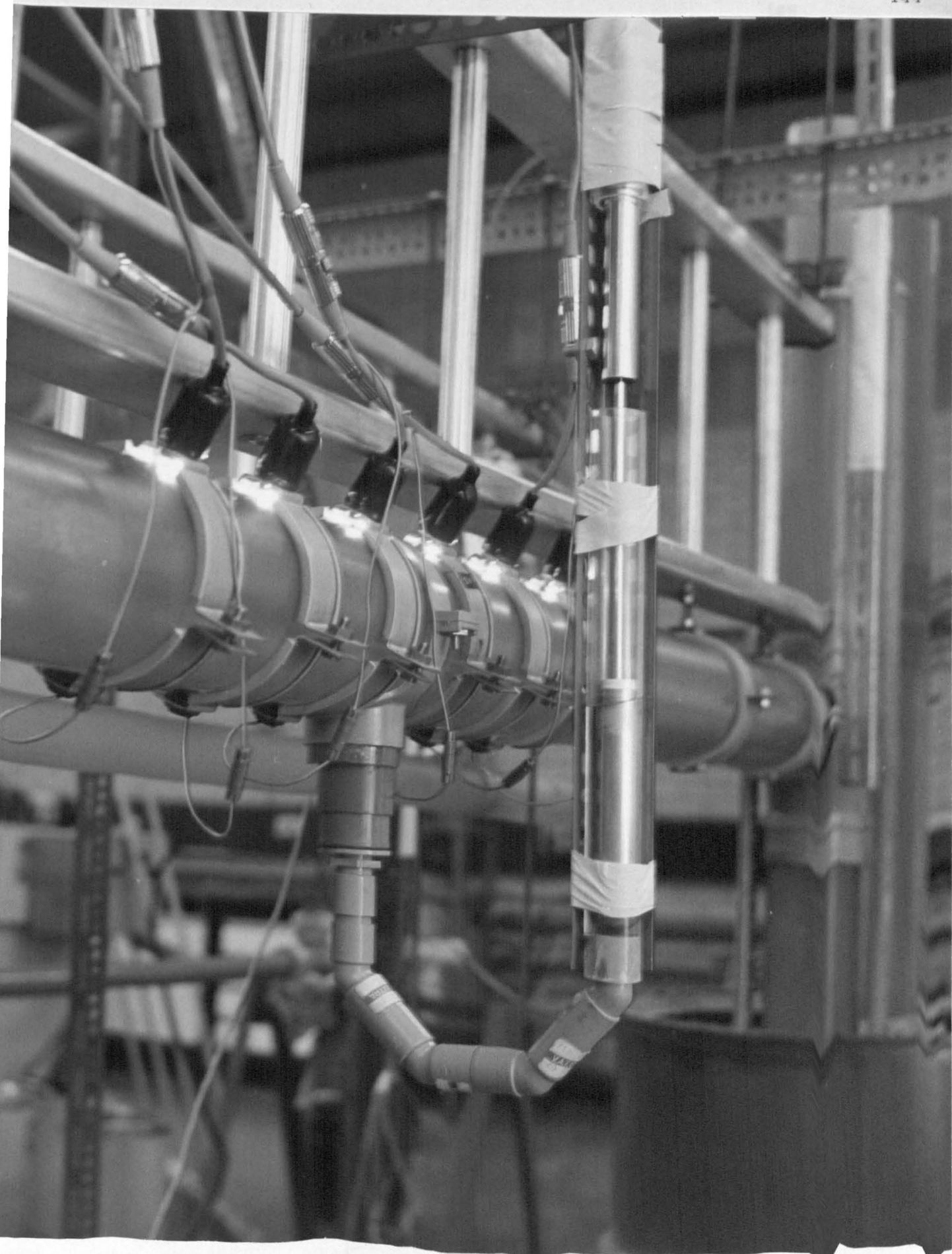
FIGURE 9. Layout of depth measurement u-tube and float chamber.
