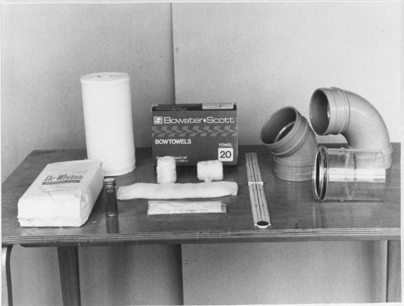
FIGURE 14. Photograph of the waste materials used during the research and during the pilot study. Back row, left to right: Kleenex paper towel roll, Bowater Scott 20 paper towel pack, 135° plastic knuckle bend and 92½° plastic radiused bend. Front row, left to right: Dr White C<sub>2</sub> pack of maternity pads and flat and rolled examples of these and a clear acrylic pipe coupler. Front centre: Simulated faeces kit made up of horse serum and baby milk powder.
