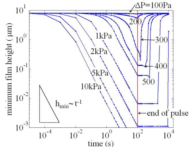
**Figure 5:** Time evolution of the minimum value of the height profile ( $h_{min}$ ) of a wetting film subjected to an air-jet for 100s at different  $\Delta P$ .
