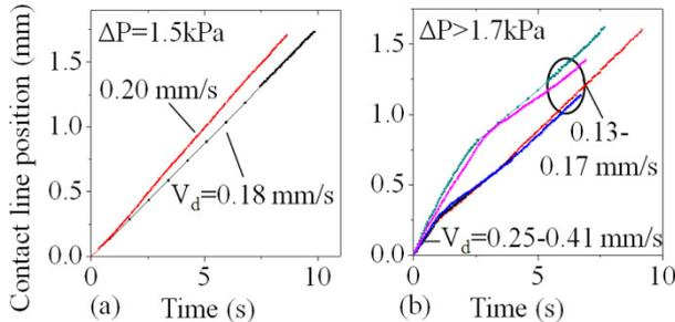
**Figure 9:** Experimentally determined position of the contact line as a function of time for the case of (a) a single rupture site ( $\Delta P=1.5$  kPa) and (b) for the case of a thin center layer with multiple rupture sites ( $\Delta P>1.7$  kPa).
