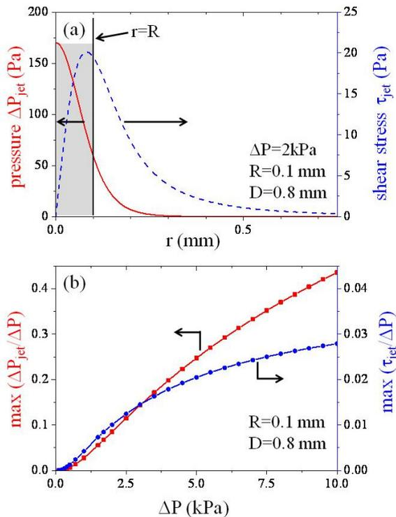
**Figure 3:** (a) The pressure  $\Delta P_{jet}(r)$  (red, left axis) and shear stress  $\tau_{jet}(r)$  (dashed blue line, right axis) numerically calculated for  $\Delta P=2$  kPa. (b) The normalized maximum values of  $\Delta P_{jet}$  (red squares, left axis) and shear stress  $\tau_{jet}$  (blue circles, right axis) as a function of  $\Delta P$ .
