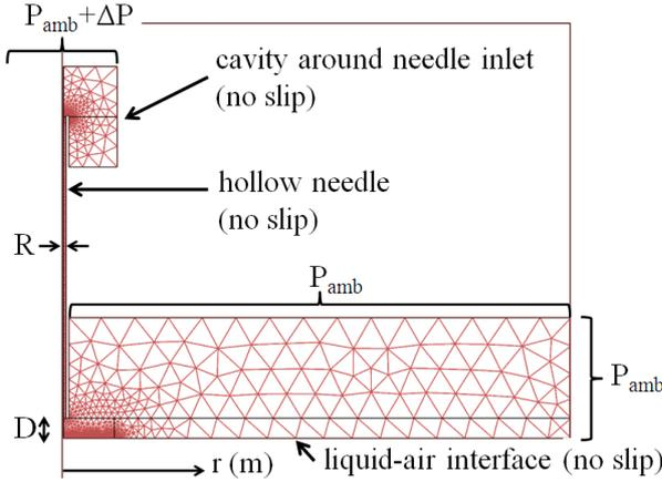
**Figure 2:** The geometry and mesh used for the air-jet simulation.
