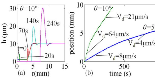
**Figure 10:** Numerical simulation of the dewetting of a film with a step in film thickness. (a) height profiles for different times (b) contact line position as a function of time for two different contact angles  $\theta$ .
