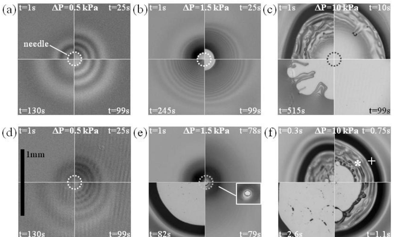
**Figure 6:** The impact of an air-jet pulse from a hollow needle ( $\varnothing 200\mu\text{m}$ , duration 100s) onto (a,b,c) a wetting film of 3EG on glass ( $6-8\mu\text{m}$ ) and (d,e,f) a partially wetting film of 3EG on PMMA at different pressure settings and different times during and after the jet.
