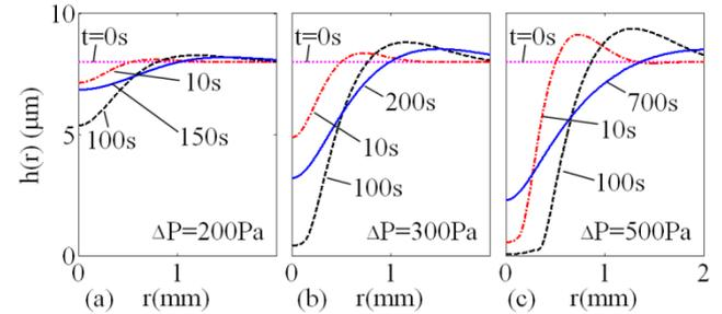
**Figure 4:** Film height profiles as a function of time for a wetting film ( $h_0=8\mu m$ ) subject to an air-jet pulse of duration 100s for (a)  $\Delta P=200$  Pa, (b)  $\Delta P=300$  Pa and (c)  $\Delta P=500$  Pa.
