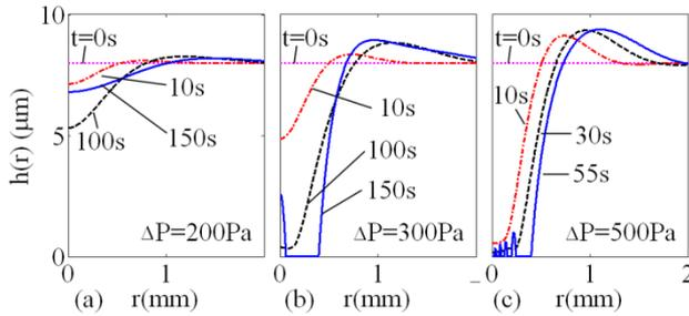
**Figure 7:** Film height profiles as a function of time for a partially wetting  $8\mu\text{m}$  wetting film under a 100s air-jet pulse for (a)  $\Delta P=200\text{Pa}$ , (b)  $\Delta P=300\text{Pa}$  and (c)  $\Delta P=500\text{Pa}$ .
