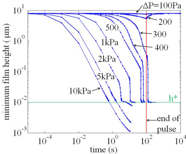
**Figure 8:** Time evolution of the minimum value of the height profile of a partially wetting film subjected to an air-jet for 100s at different  $\Delta P$  derived from numerical simulations.
