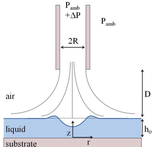
**Figure 1:** Schematic representation of the experimental configuration (not to scale).
