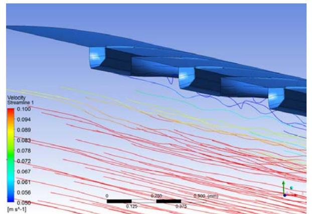
**Fig. 6.** Velocity (m/s) streamlines near to endothelium at the very end region of the stented artery. Flow from right to left
