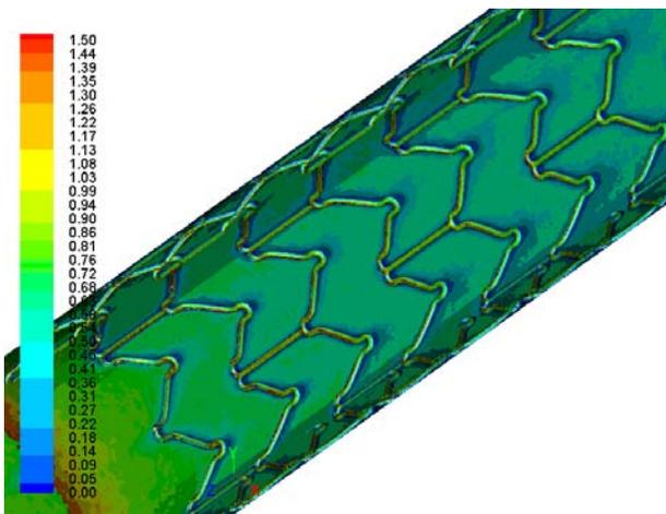
**Fig. 8.** WSS (N/m<sup>2</sup>) contours of the artery (stent and endothelium). Flow from left to right
