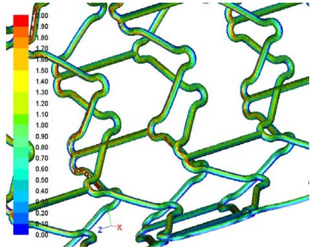
**Fig. 10.** WSS (N/m<sup>2</sup>) contours on struts of the artery. Front and rear view projected in a single plane. Flow from left to right
