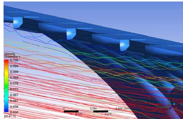
**Fig. 5.** Velocity (m/s) streamlines near to endothelium of the stented artery. Flow from right to left
