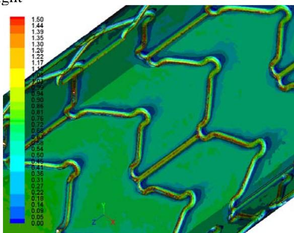
**Fig. 9.** WSS (N/m<sup>2</sup>) contours of the artery (stent and endothelium). Enlarged view. Flow from left to right
