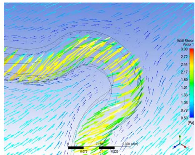
**Fig. 12.** WSS (N/m<sup>2</sup>) vectors of the artery (stent)
