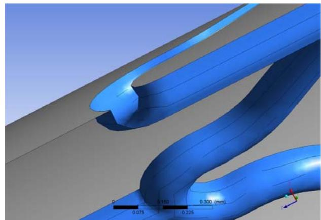
**Fig. 2.** Stent struts are 50.0 % embedded into the arterial wall
