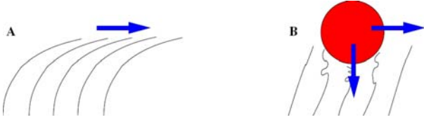
Fig. 3: Assumed mechanical properties of the glycocalyx protein chains, subject to a streaming flow only (A) and direct, ballistic interaction with a particulate (B). Note that the principal deformation is assumed to be confined to the tip of the filaments, adjacent to the lumen (figure not to scale).
