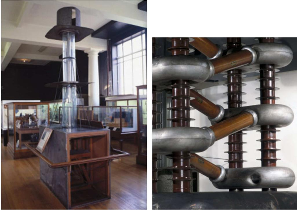
FIGURE 1.4: Cockroft and Walton's accelerator and voltage generator. The accelerator has large potential difference built up between the terminal at the top and the earth. The particles are fired downwards through the evacuated drift tube to a target at the bottom. The generator has large capacitors, encased in the vertical pipes, and diodes, in the diagonal pipes, to prevent them discharging. Image from [11]
