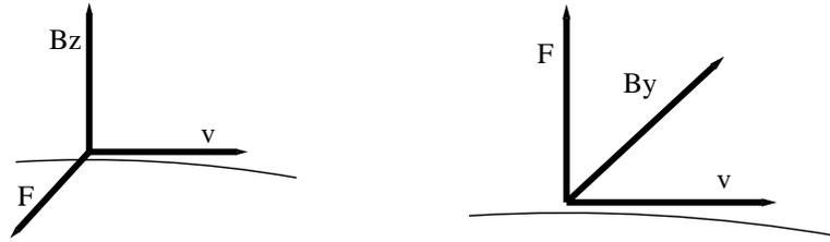
FIGURE 2.3: A particle just above the reference orbit will experience a force upwards if  $B_y$  is positive.
