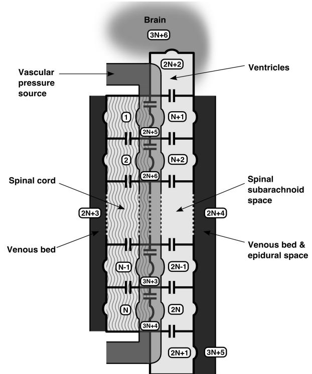
Fig. 1: Schematic diagram of the lumped-parameter model.
