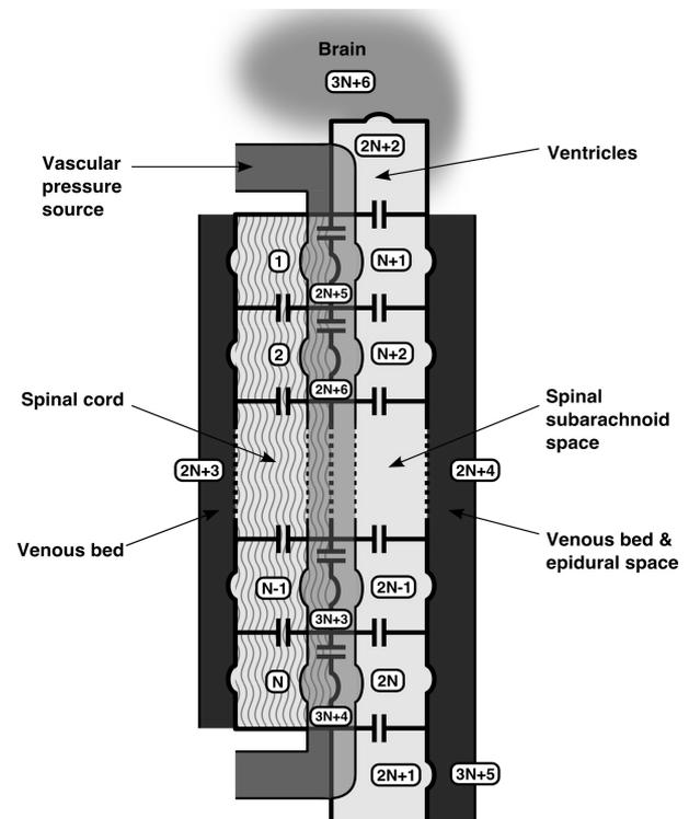
Fig. 1: Schematic diagram of the lumped-parameter model.
