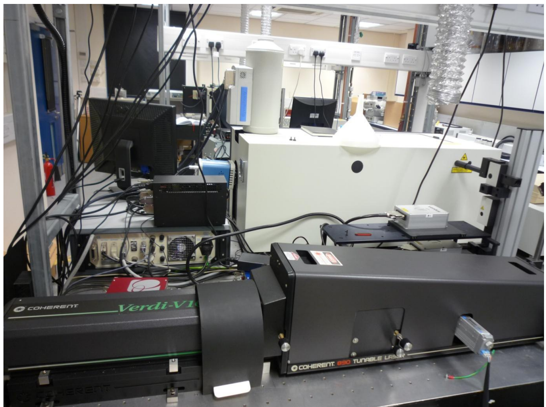
Figure 2.7 HORIBA JOBIN YVON LabRAM HR800 Raman microscope. Top: Front view; Bottom: External green and infrared lasers.
