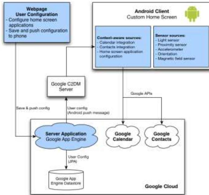
**Figure 2 System architecture**
