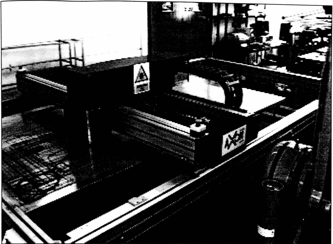
Figure (9.2.1.1). The computer controlled cutting table. The laser head is surrounded by a case of special plastic which acts as a filter to reduce the possible hazard of beam reflectance.
