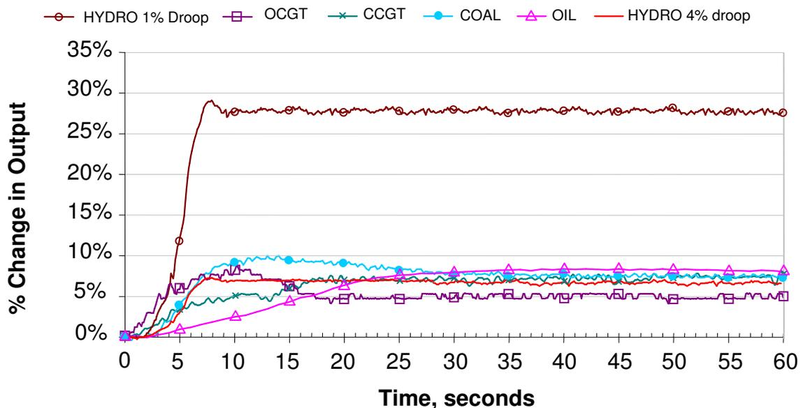
**Figure 4.6 - Generator response to applied test frequency injection signal**
