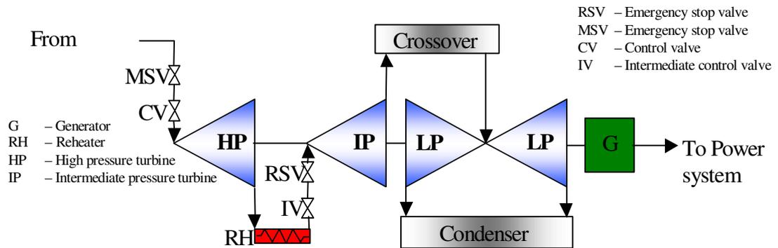
**Figure 5.9 - Single reheat steam turbine**
