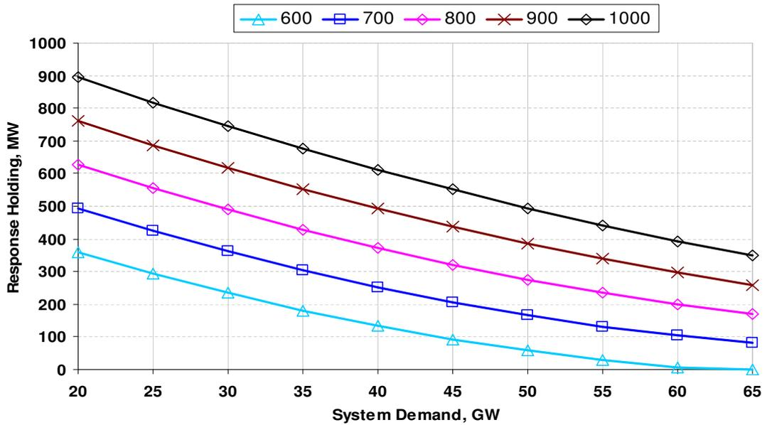
Figure 7.16 – Primary response requirement (including margin) for significant losses
