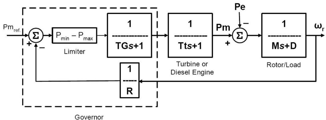
**Figure 4.12 – System transfer function**
