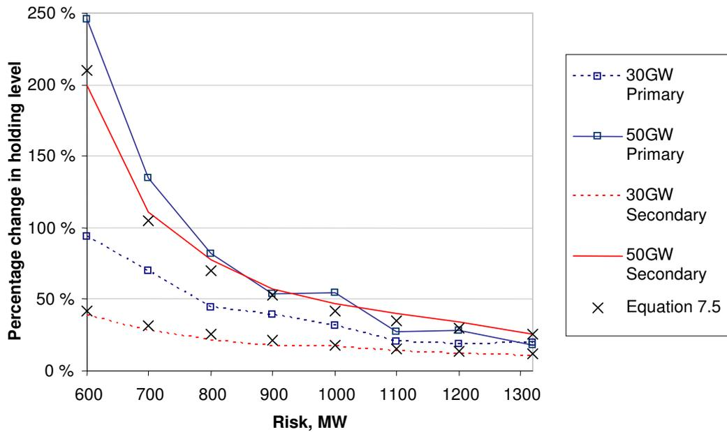
**Figure 7.11 – Differences in response requirements for alternate start frequencies (three standard deviations)**
