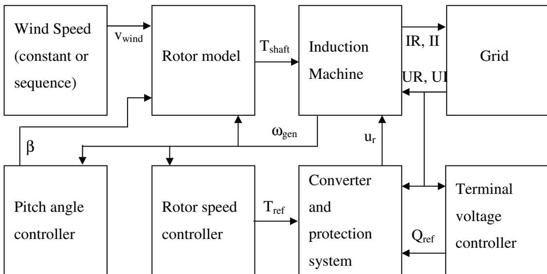
**Figure 8.2 – Variable speed wind turbine model**
