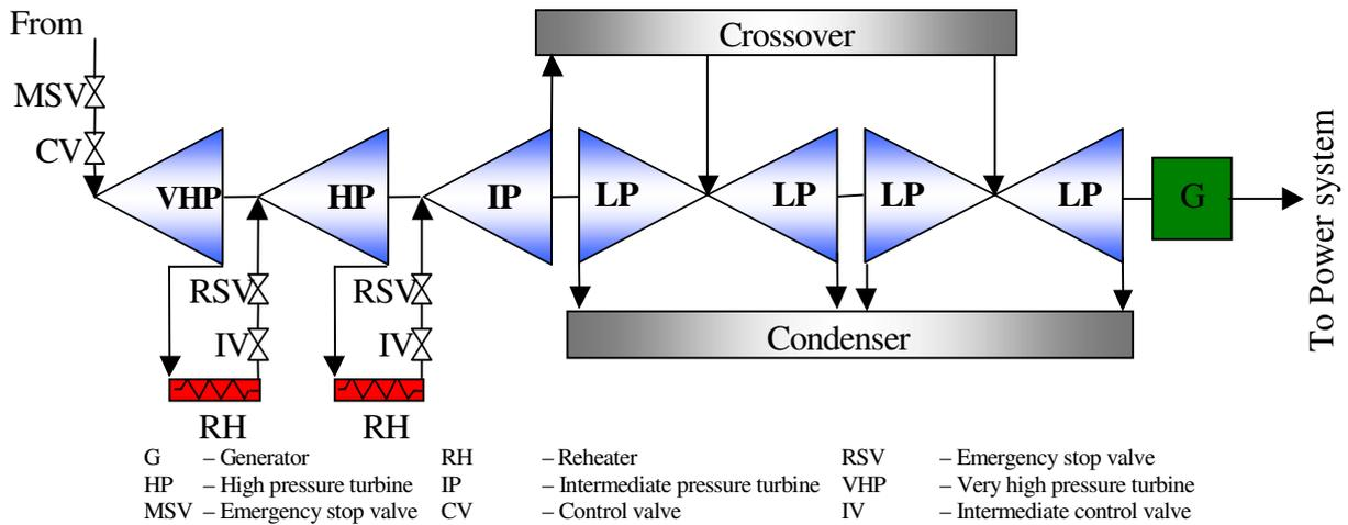
**Figure 5.10 - Double reheat steam turbine**
