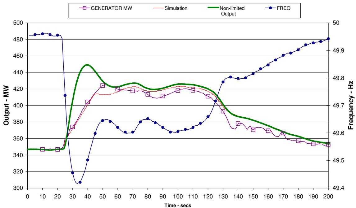
**Figure 5.27 - Frequency response of a rate-limited generator during an actual incident and the simulated response**
