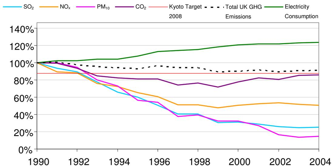
**Figure 2.4 – Emissions to air from electricity generators indexed to 1990 levels<sup>‡‡</sup>**
