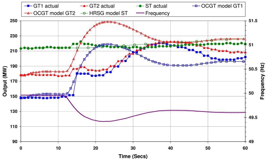
**Figure 5.19 - Frequency response of a CCGT gas turbine module during an actual incident and the simulated response using OCGT representation**
