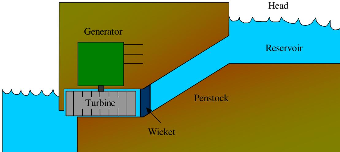
**Figure 5.23 - Hydroelectric turbine arrangement**
