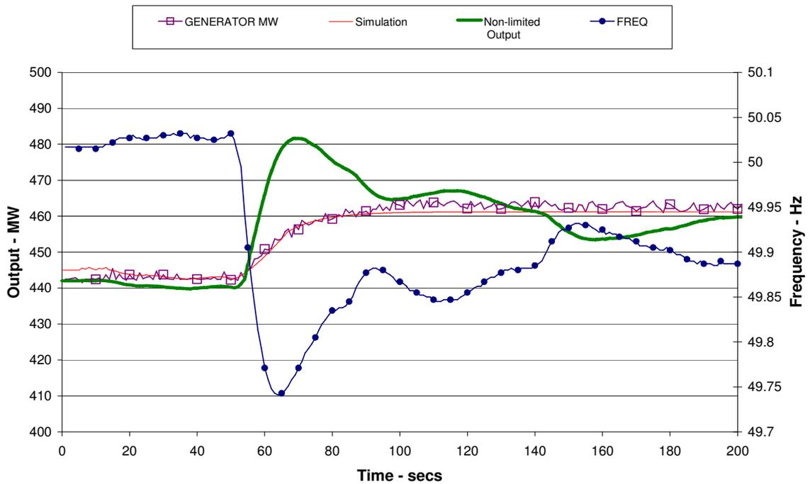
**Figure 5.28 - Frequency response of an output-limited generator during an actual incident and the simulated response**
