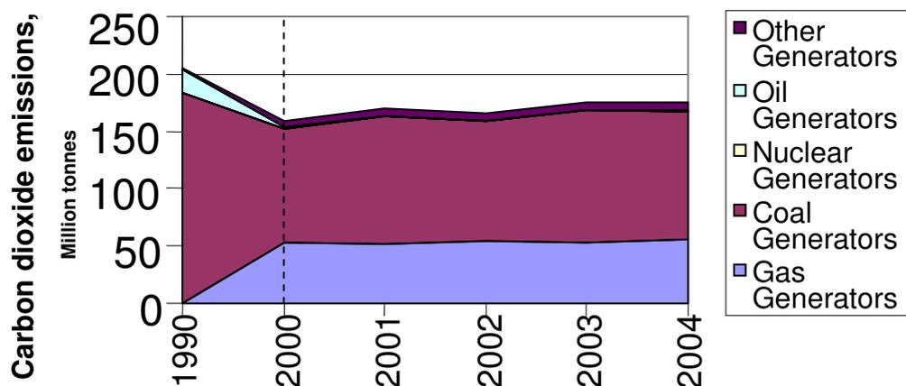
Figure 2.3 – CO<sub>2</sub> emissions to air from electricity generators<sup>##</sup>
