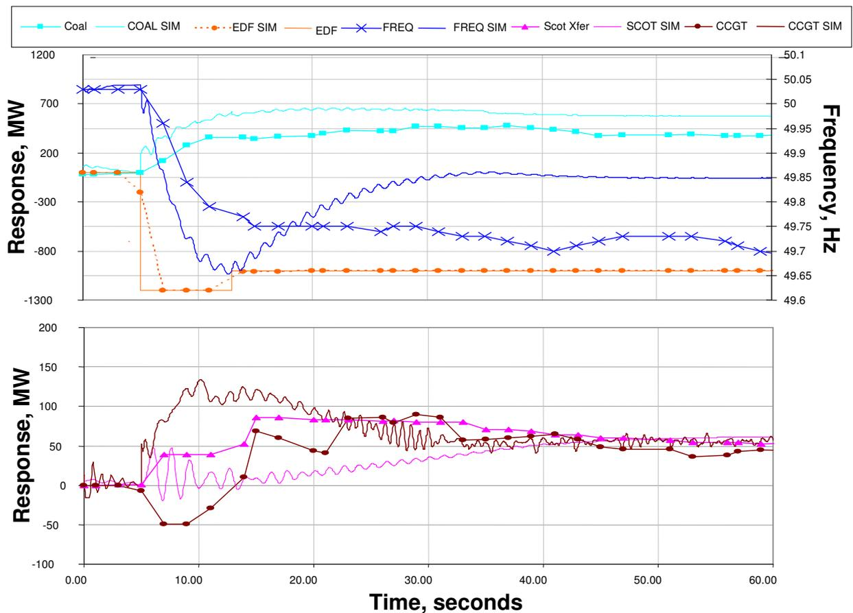
**Figure 7.2 – Simulated 1000 MW loss from 02/12/05**
