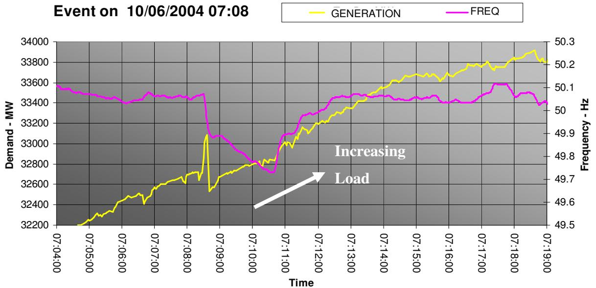
**Figure 6.4 - Generator loss under unclear load conditions**
