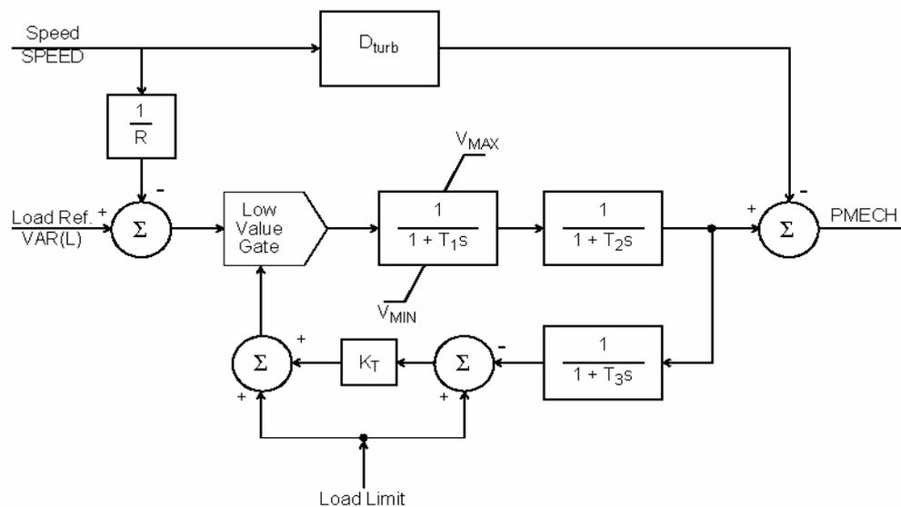
**Figure 5.18 – Open cycle gas turbine model**
