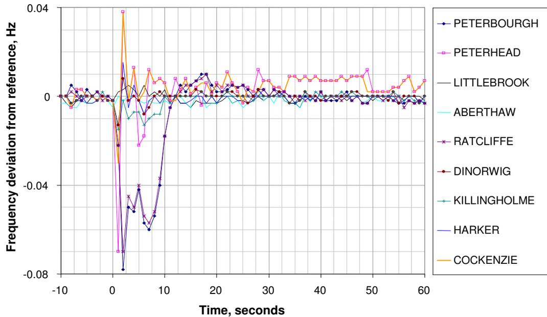
**Figure 4.13 – Impact of location on grid frequency**
