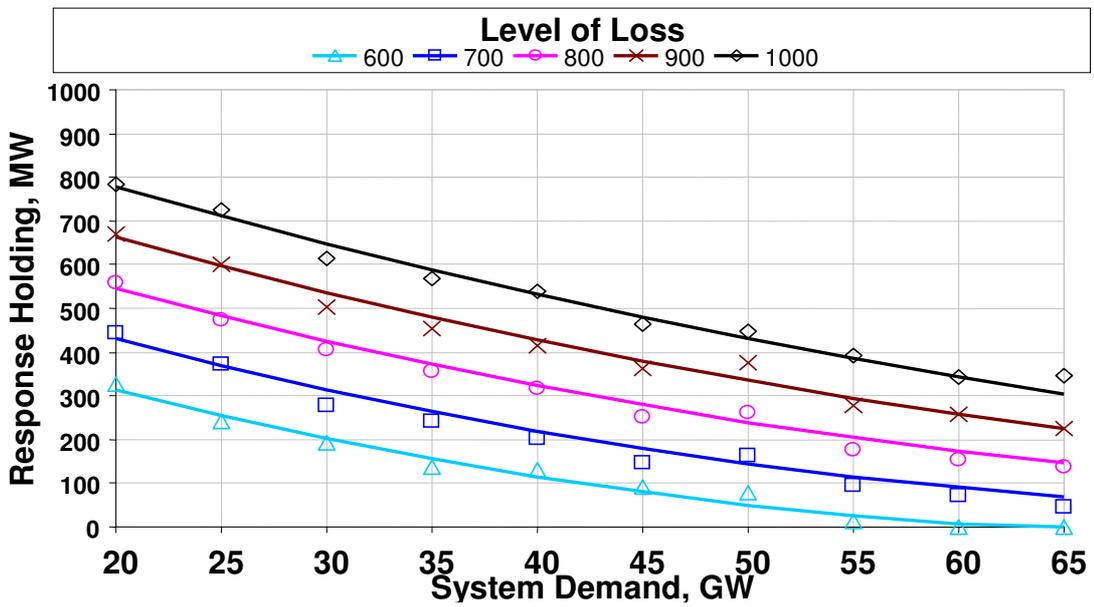
Figure 7.7 – Primary response requirements for significant losses
