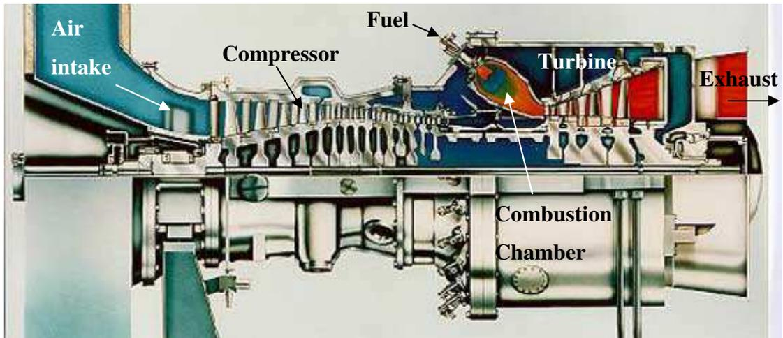
**Figure 5.15 - Diagram of a simple gas turbine**
