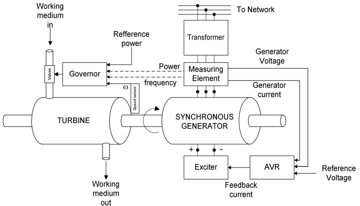
**Figure 5.3 - Block diagram of generator control system**
