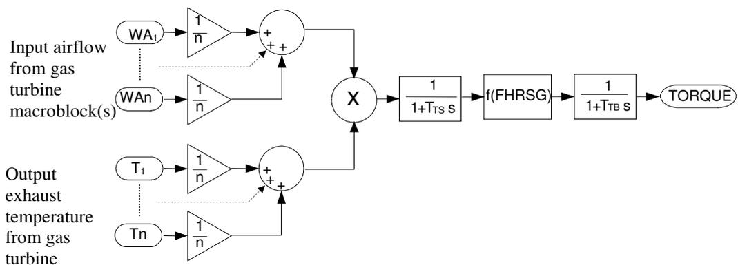
Figure 5.22 – HRSG model
