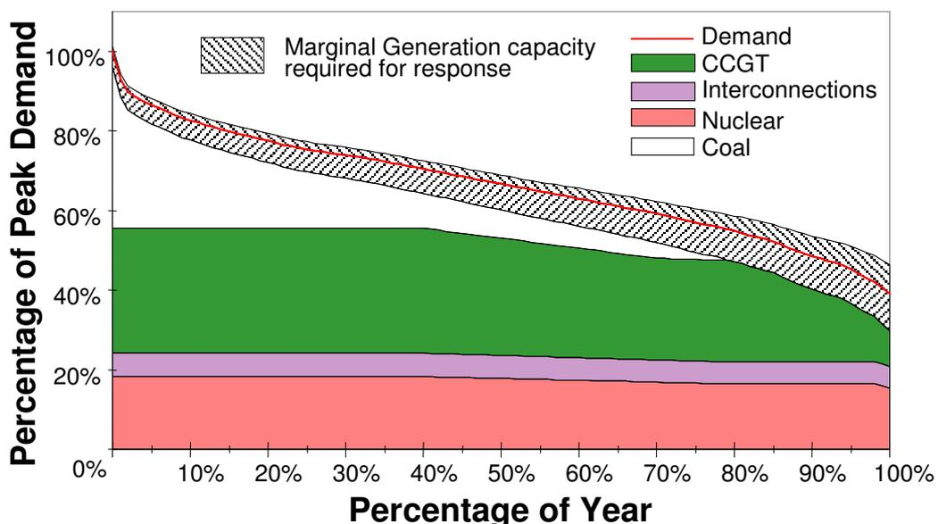
**Figure 3.2 - Load duration curve showing breakdown of grid connected generation**
