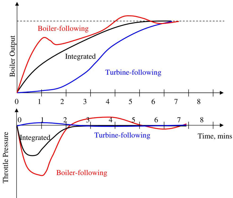
**Figure 5.6 - Dynamic behaviour of steam boiler controls**
