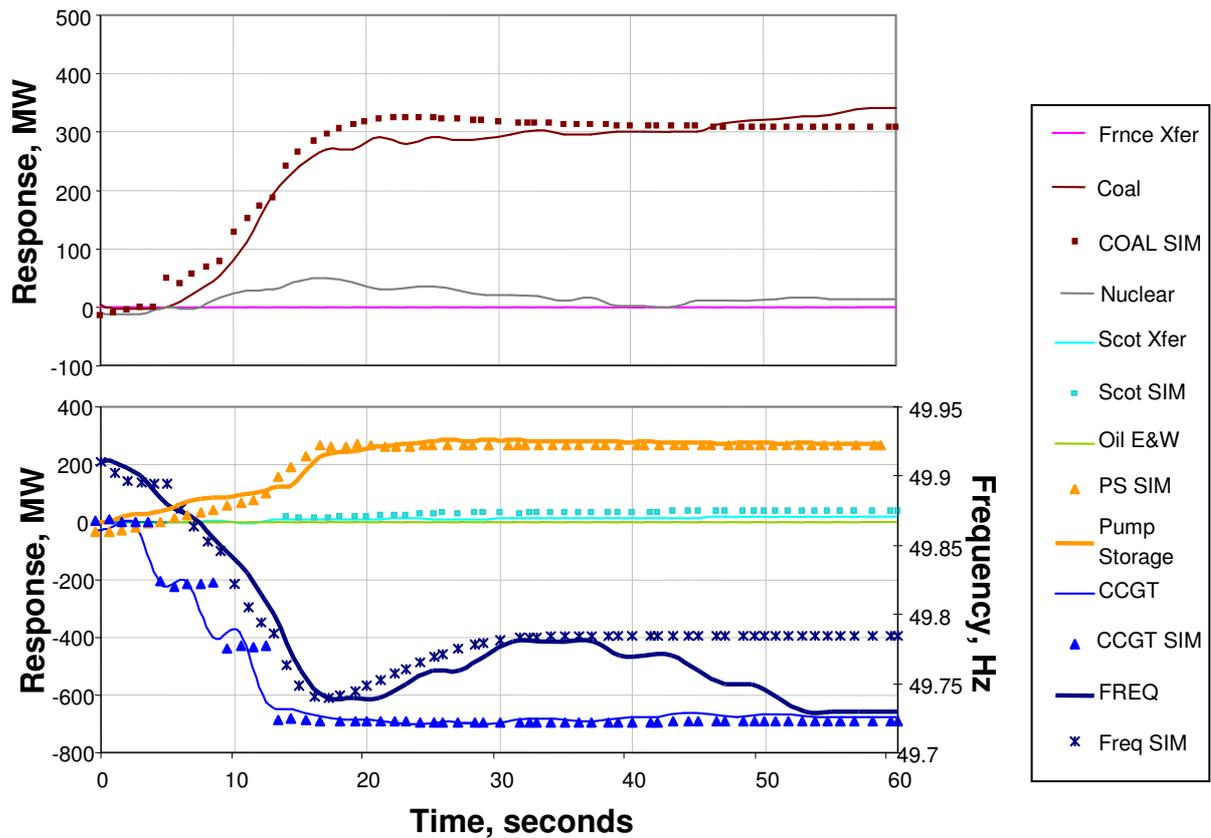
**Figure 7.3 – Simulated 790MW loss from 21/01/06**
