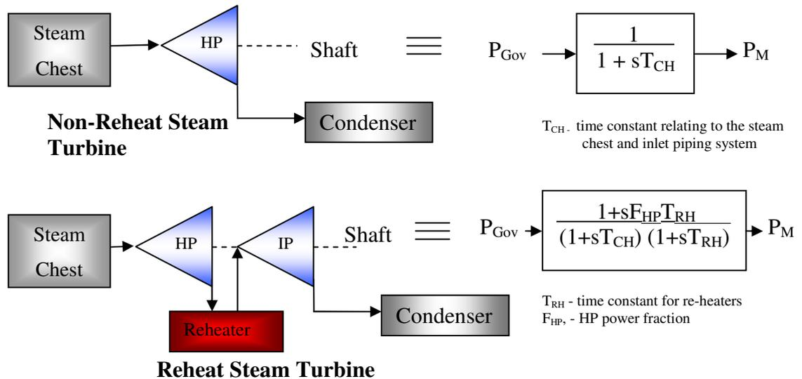
**Figure 5.11 – Simple steam turbine models**
