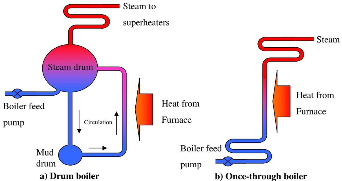
**Figure 5.5 - Typical steam boiler arrangements used in power stations**
