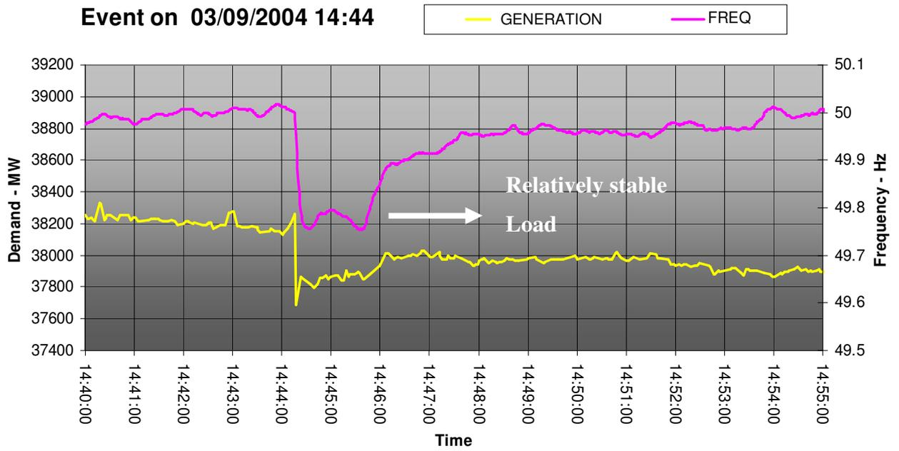
**Figure 6.3 - Generator loss under constant load conditions**
