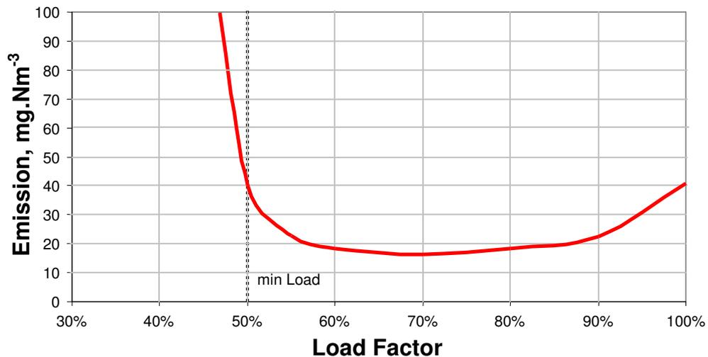
**Figure 2.8 – Emissions of nitrogen oxides associated with partload operation of F Class Combined Cycle Gas Turbines** [Tauschitz and Hochfellner(2004)]
