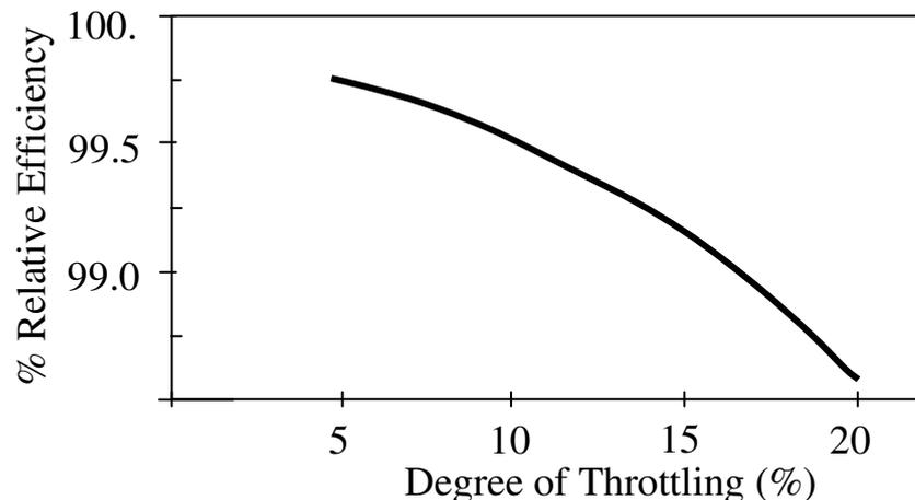
**Figure 2.5 – Partload efficiency of conventional steam power stations**<sup>[Kuerten(1998)]</sup>
