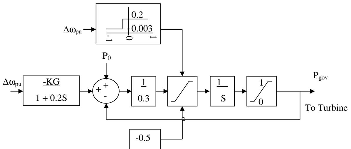
**Figure 5.13 - Modification to coal governor to allow frequency triggered rate-limit**
