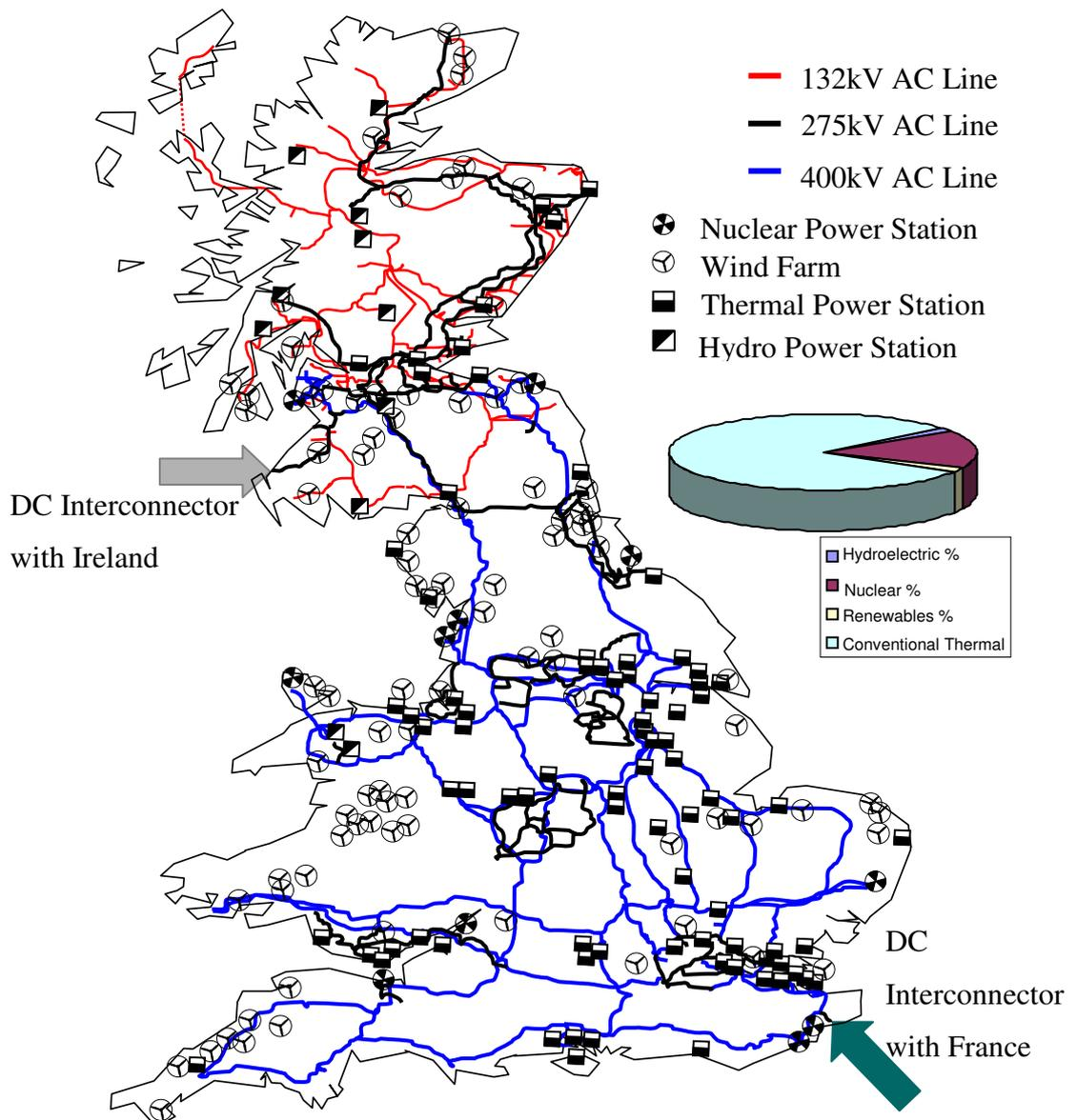
**Figure 3.1 – Generation capacity and national transmission lines of the Great Britain super grid.**
