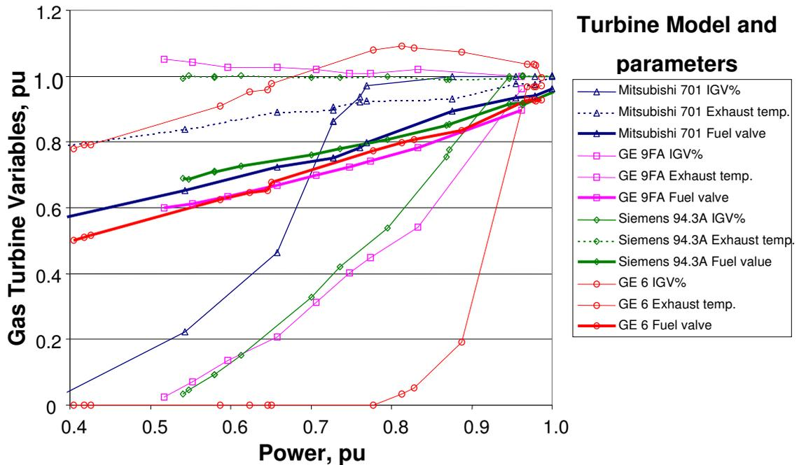
**Figure 5.20 - Exhaust temperature, IGV position and fuel valve position of a number of combined cycle gas turbines**
