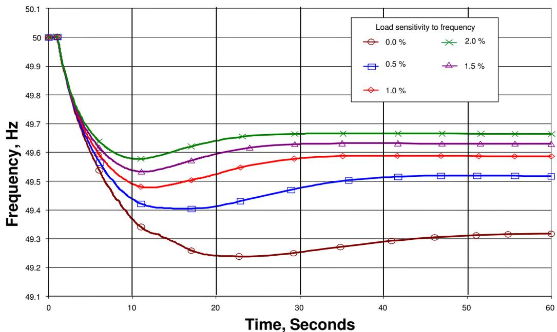
**Figure 4.5 - Effect of load sensitivity on system frequency**
