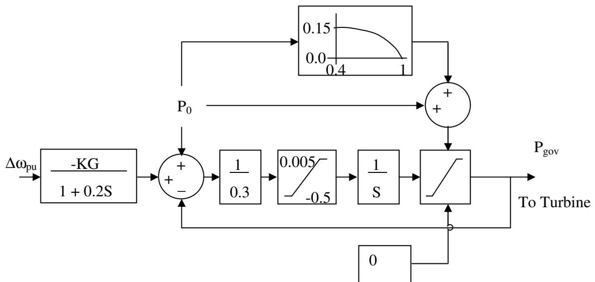
**Figure 5.14 - Modification to coal governor to allow an output-limit**
