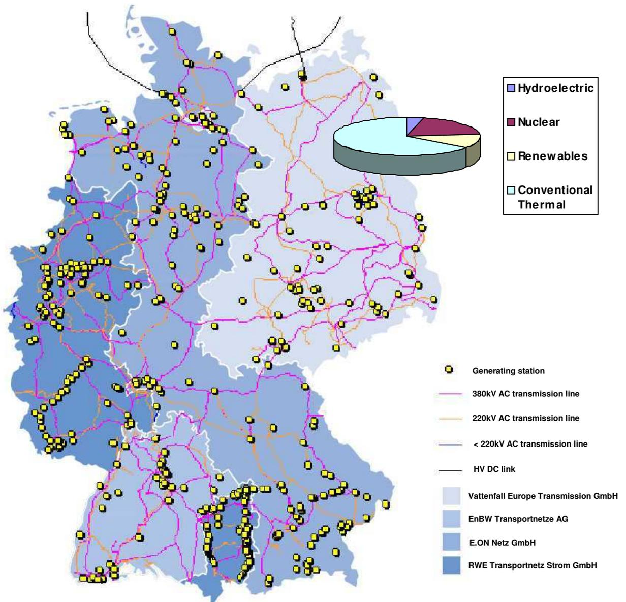
Figure 3.4 - German system operators, generation mix<sup>\*\*\*</sup> and HV grid network<sup>†††</sup>
