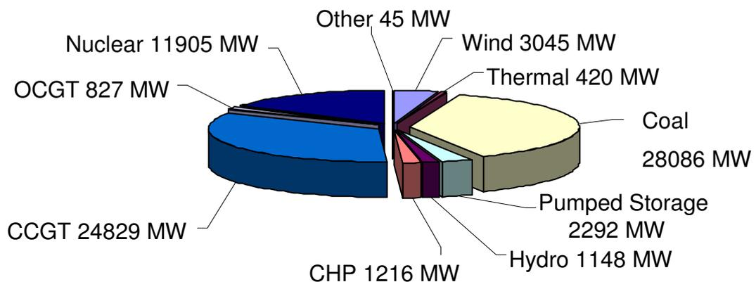
**Figure 5.1 - GB generation capacity by fuel types** [source from the DTI]
