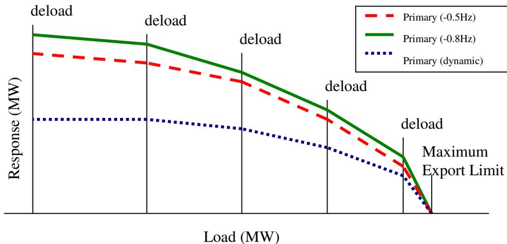
**Figure 4.7 - Example generator response profile curve**
