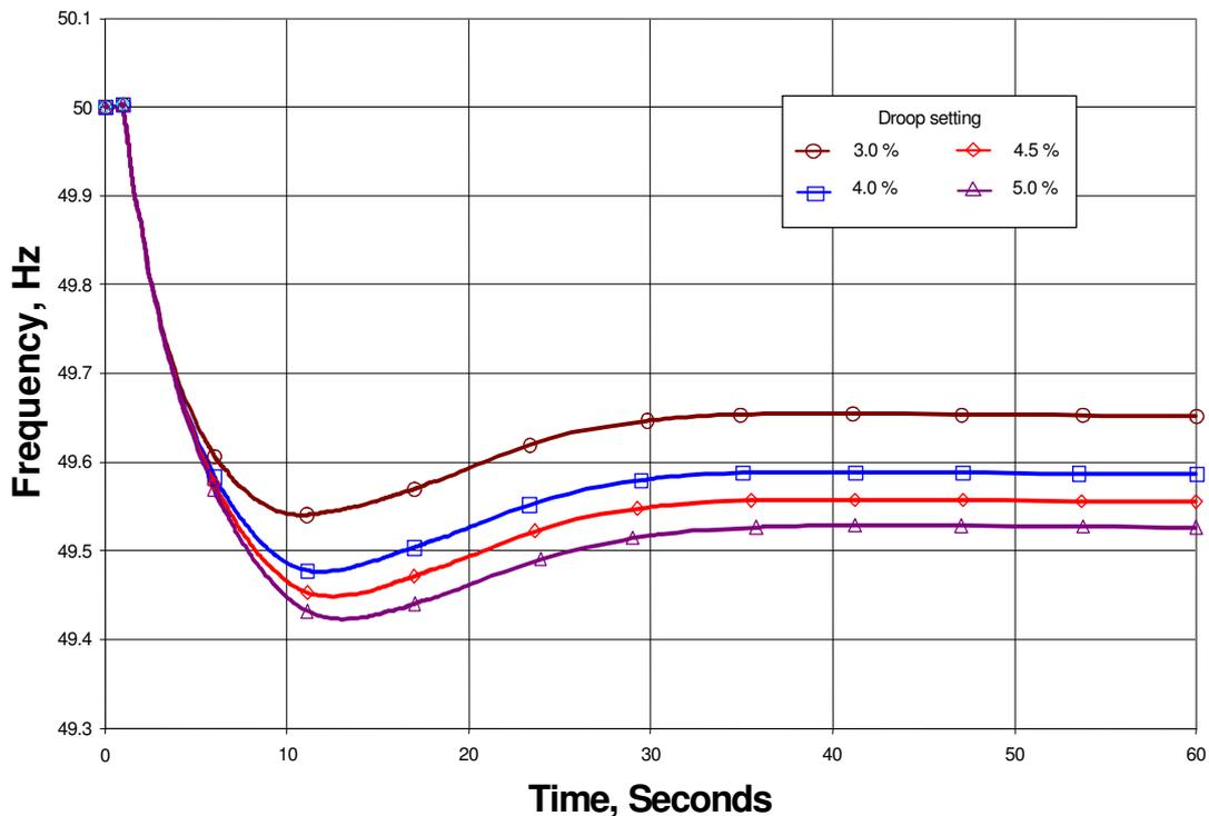
**Figure 4.2 - Effect of generator droop on system frequency**
