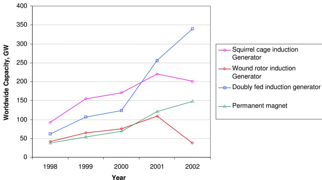
**Figure 8.1 – Installed capacity of wind turbines by type** [source: Ackermann(2005)]
