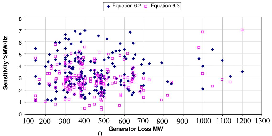
**Figure 6.8 – Magnitude of generator loss against load-sensitivity during April 2004 to June 2005**
