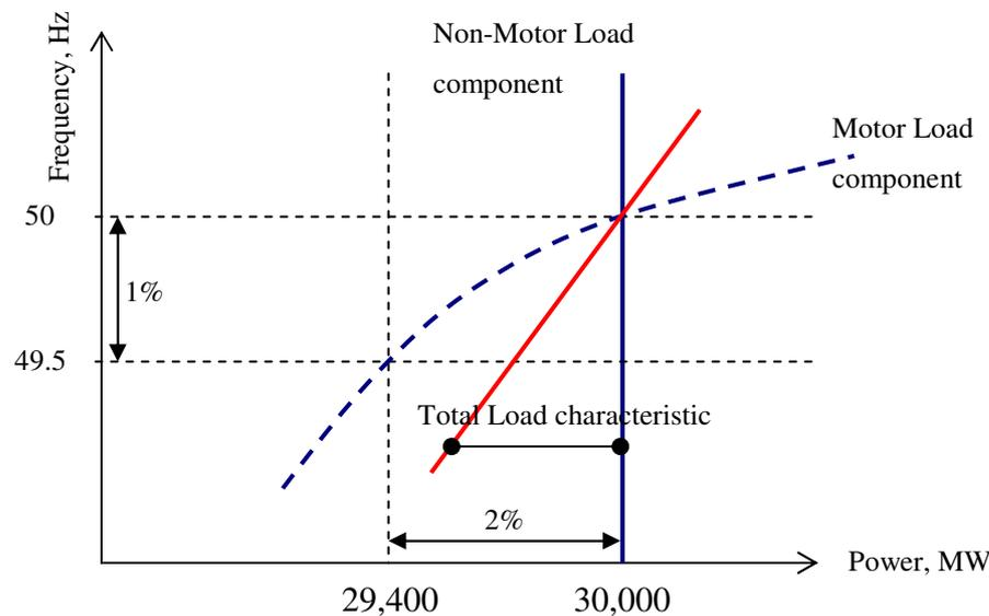
**Figure 6.2 - Power-frequency effects of motor and non-motor Loads**
