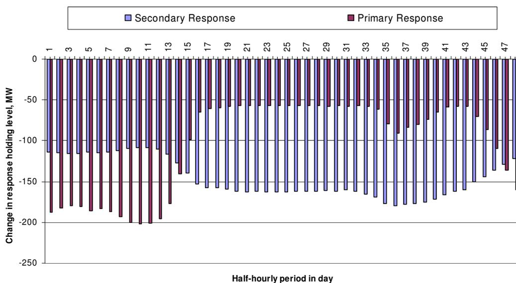
**Figure 6.11 – Changes in response holding when considering a 0.5% increase in load sensitivity against a 1320MW loss**
