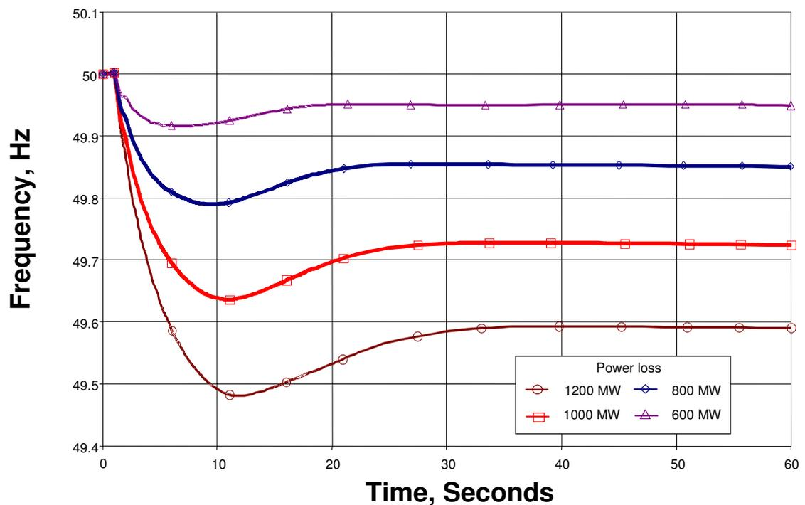
Figure 4.3 - Effect of disturbance magnitude on system frequency
