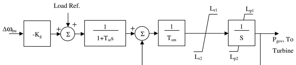
$K_R = 1/\text{Droop}$      $T_{sr} = \text{Time constant}$      $T_{sm} = \text{Servo time constant}$      $L_{r*} = \text{Rate limit}$      $L_{p*} = \text{Position limit}$
