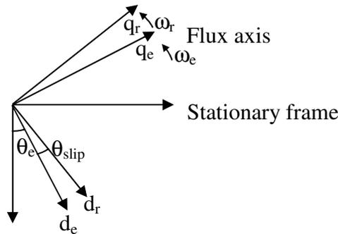
**Figure 8.3 – The direct-quadrature reference frame**
