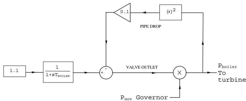
**Figure 5.7 - Model for influence of steam boiler on plant response**
