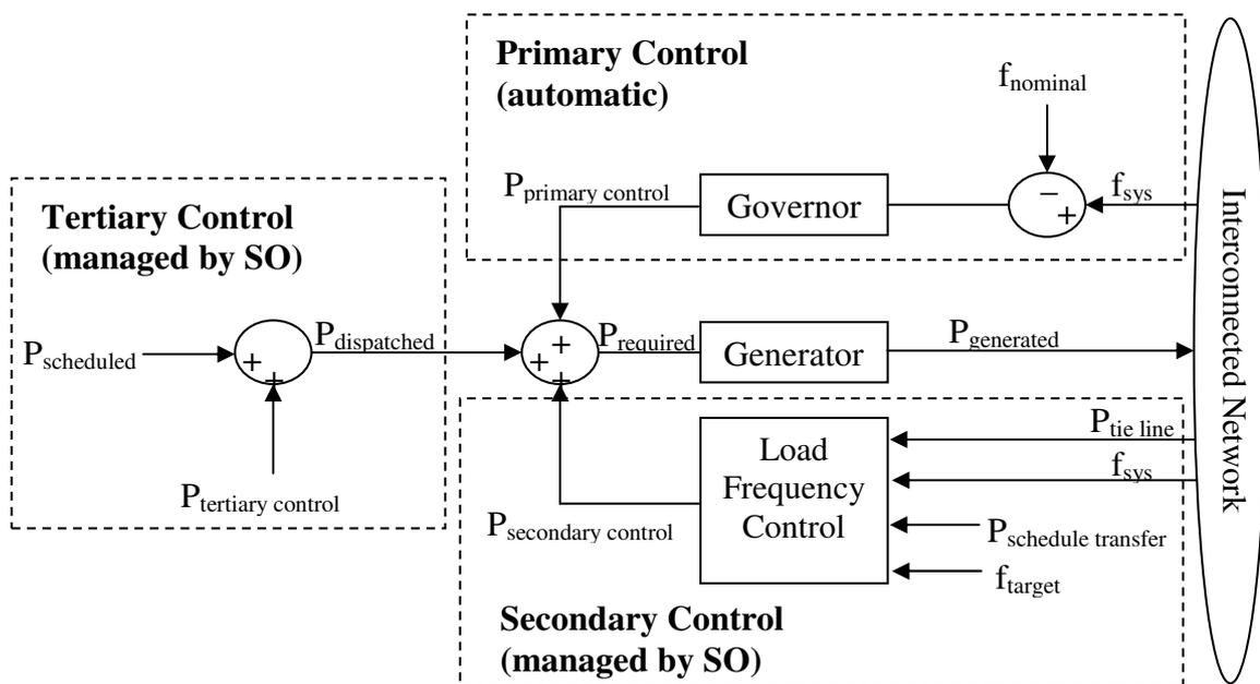
**Figure 3.5 - Frequency model provided by zones and generators within the UCTE**
