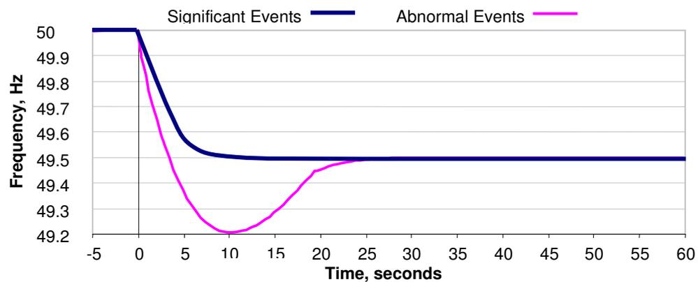
**Figure 7.4 – Frequency transients for significant and abnormal losses**
