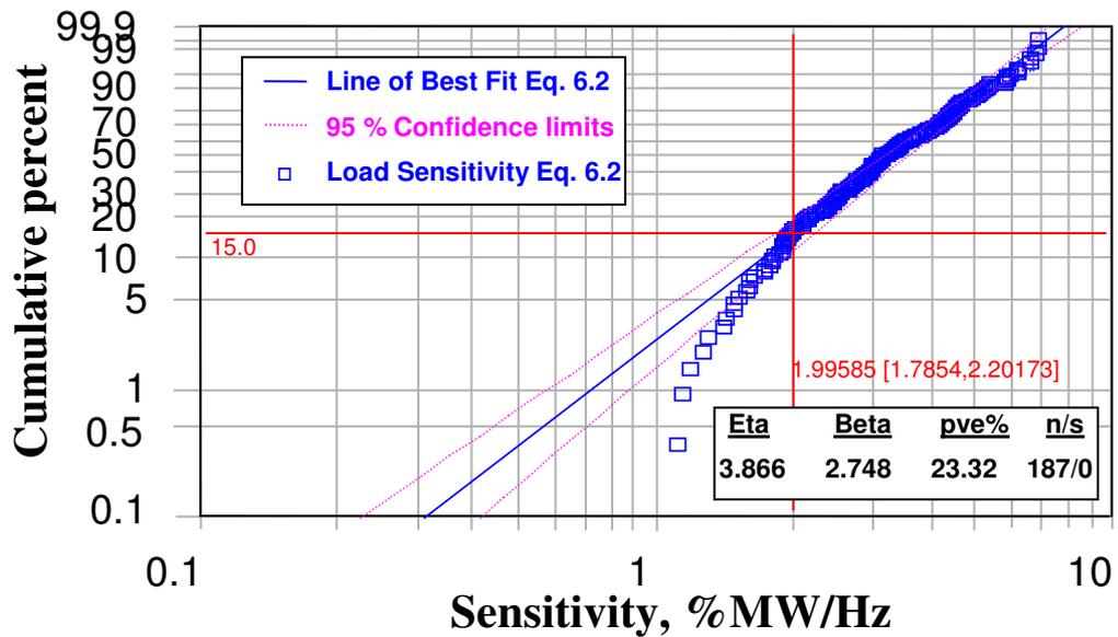
Figure 6.9 - Distribution of load sensitivity to frequency
