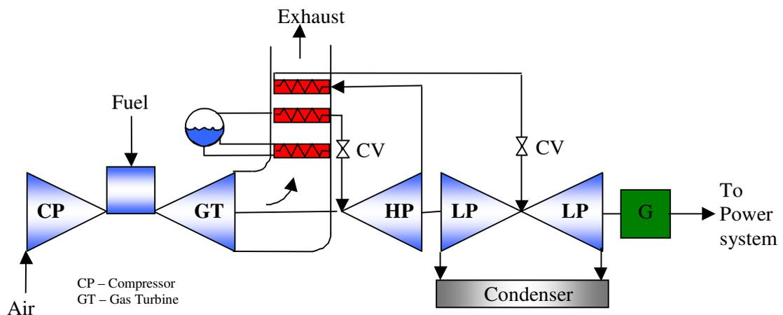
**Figure 5.16 - Single shaft tandem plant configuration**
