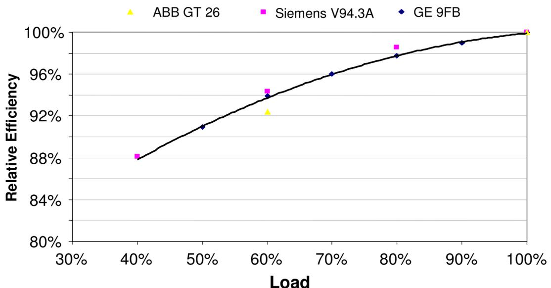
**Figure 2.6 – Partload operation of F class combined cycle gas turbines** [Tauschitz and Hochfellner(2004)]
