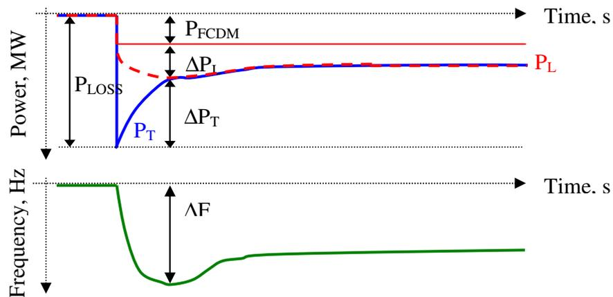
**Figure 6.5 - Assumed network response used in the calculation of load sensitivity**
