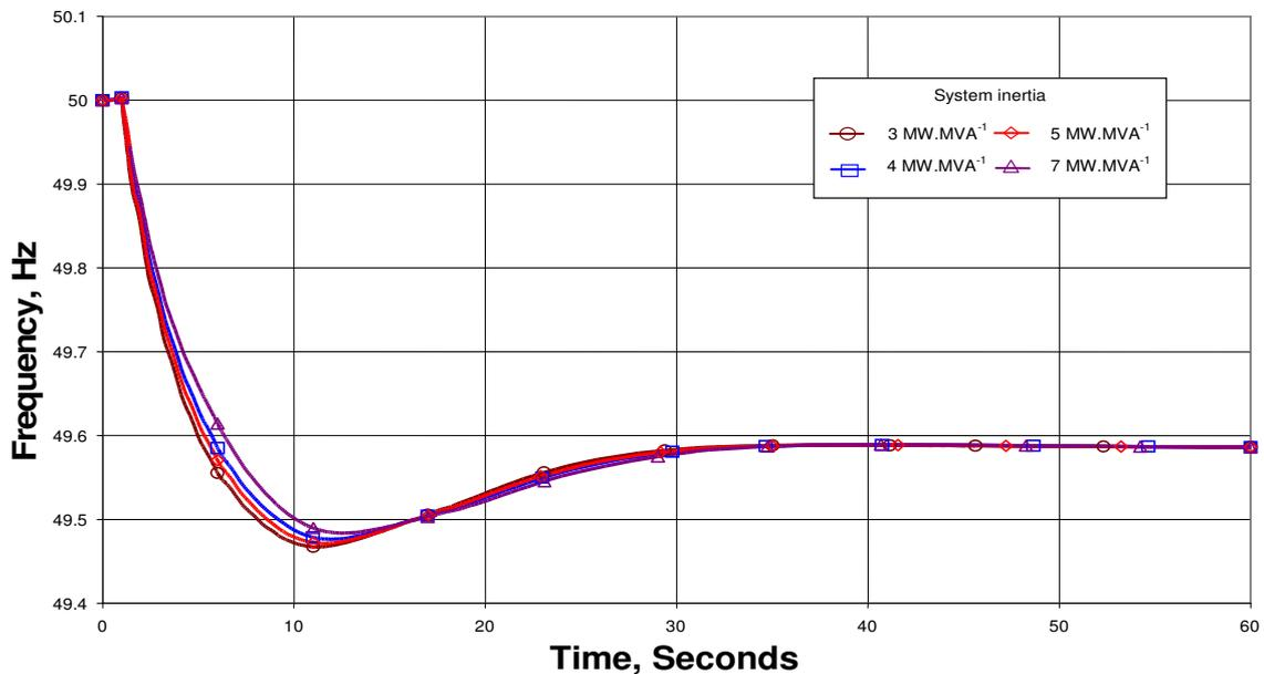
Figure 4.4 - Effect of inertia on system frequency
