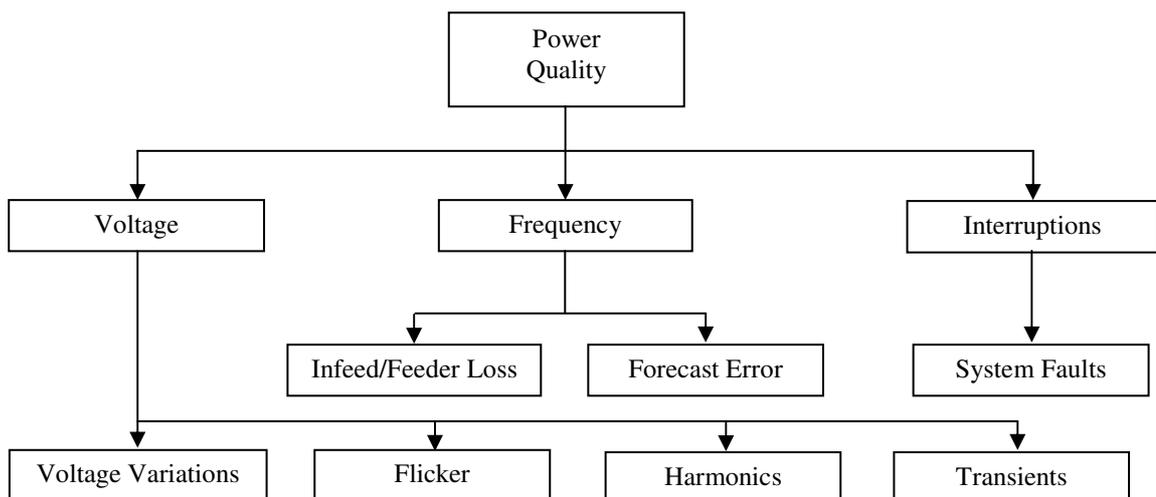
**Figure 1.1 – Components of power system quality**
