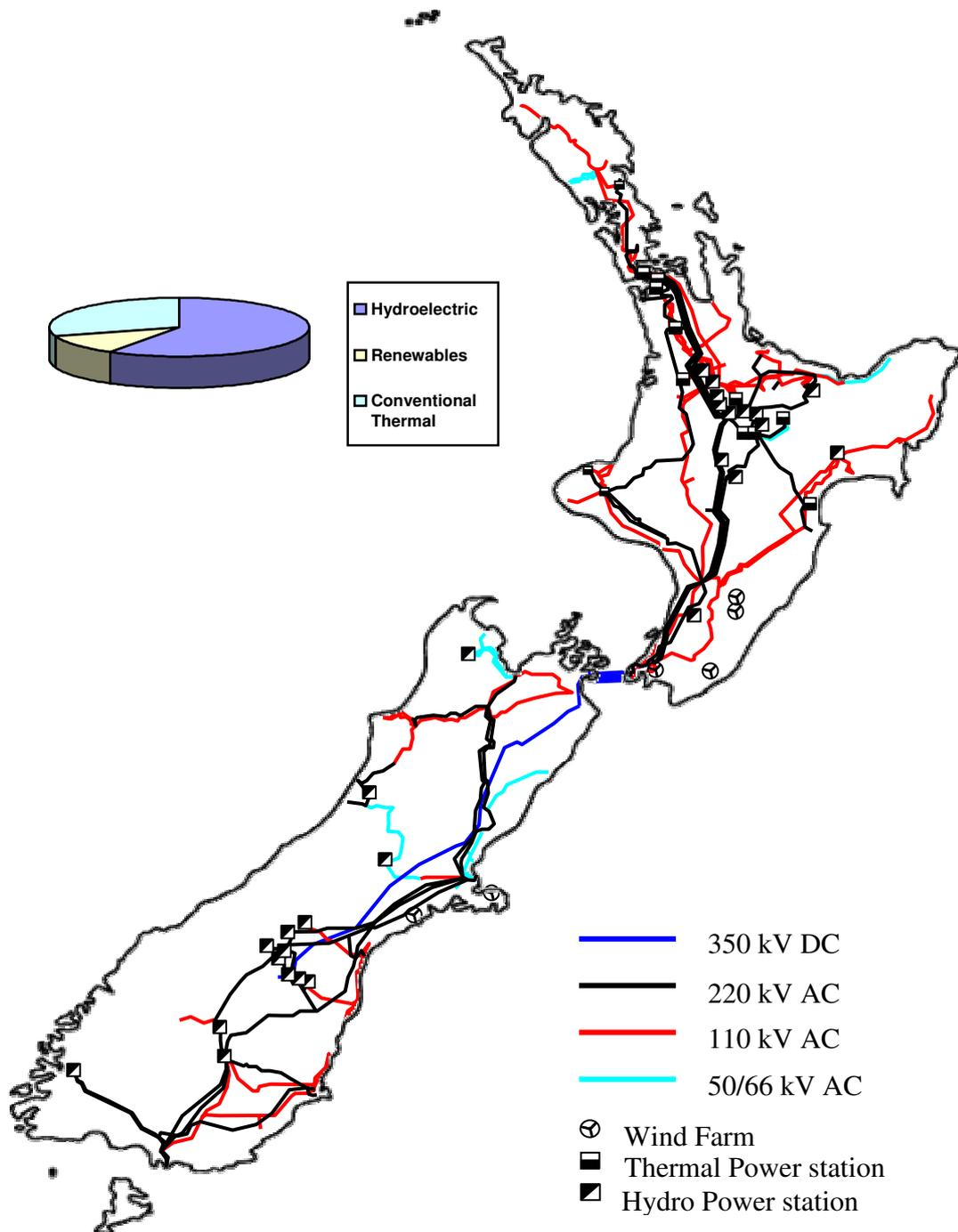
**Figure 3.7 – New Zealand transmission grid on north and south islands**
