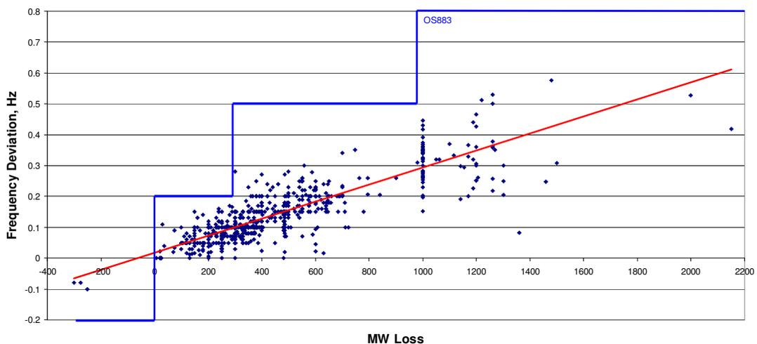
**Figure 2.9 Infeed losses and associated frequency deviations (against operating limits - OS883)**
