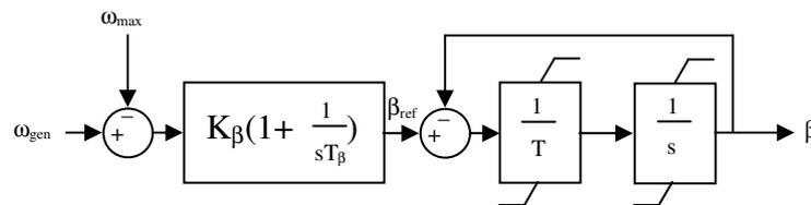
Figure 8.5 – Block diagram of pitch controller
