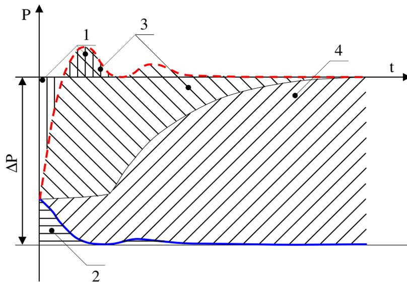
1 – Generator Rotating masses, 2 – Rotating masses of the loads, 3 – Primary Control, 4 - Secondary Control
