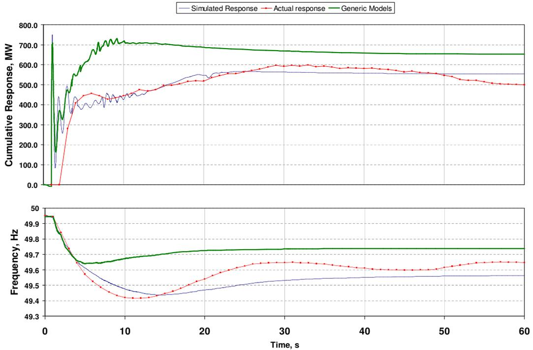
**Figure 7.1 – Simulated 1260 MW loss from 26/05/03**
