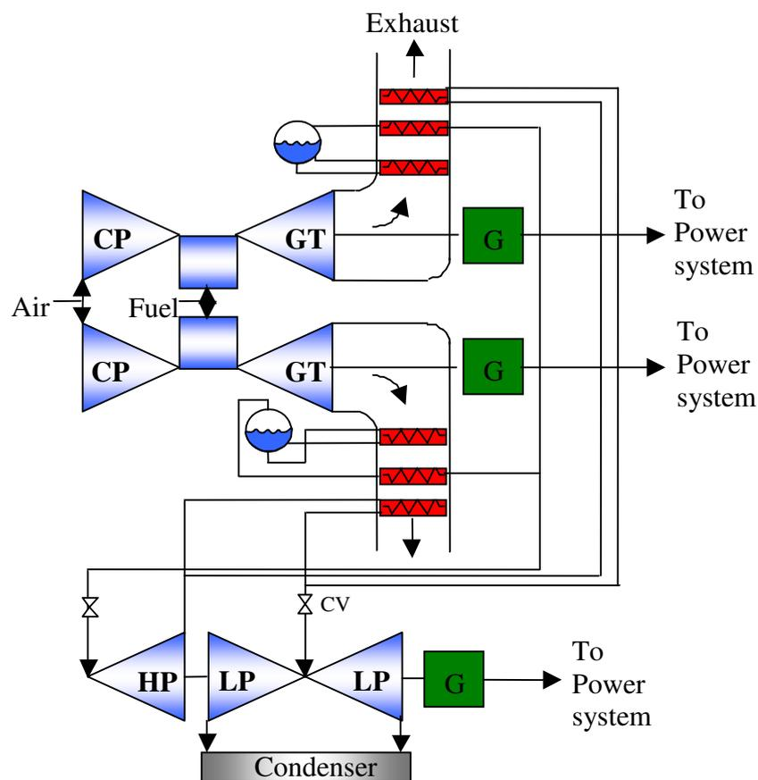
**Figure 5.17 - Multi-shaft plant configuration**
