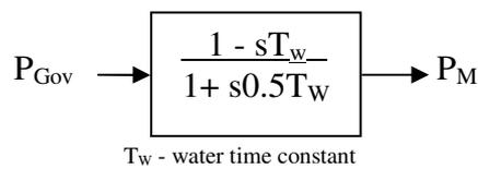
**Figure 5.25 – Hydroelectric turbine model**
