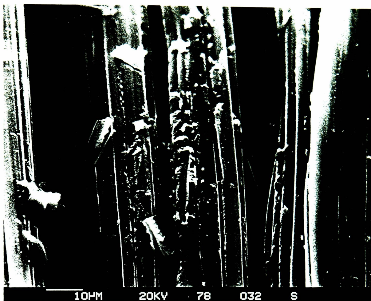
FIGURE 7.6 - Higher Resolution Image and Digimap of Boehmite Deposition on Phosphate Impregnated Carbon Cloth A
