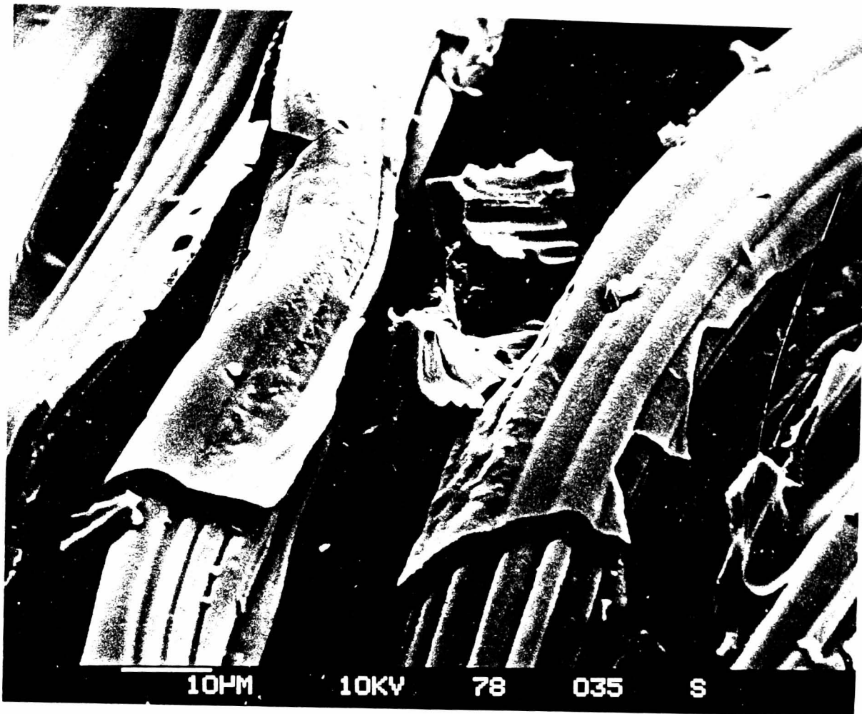
FIGURE 7.7 - Boehmite Deposition on Pre-Wetted Carbon Cloth A
