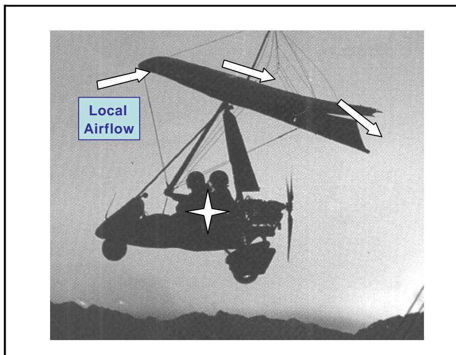
?? This “induced camber” locks the aircraft into the nose-down autorotation, which continues until the aircraft either hits the ground or breaks up.
