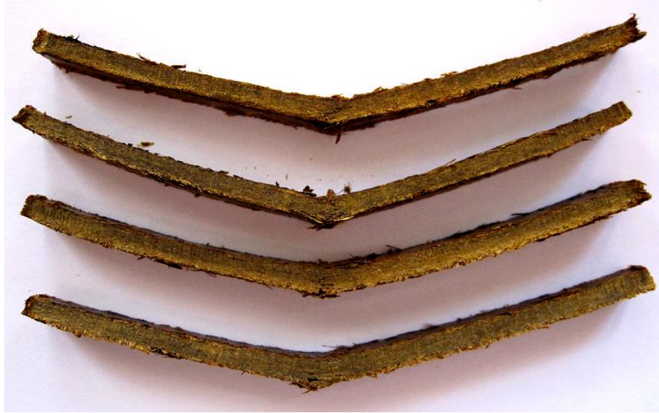
Figure 6.16: Fracture mode of TMB2 board showing absence of delamination.
