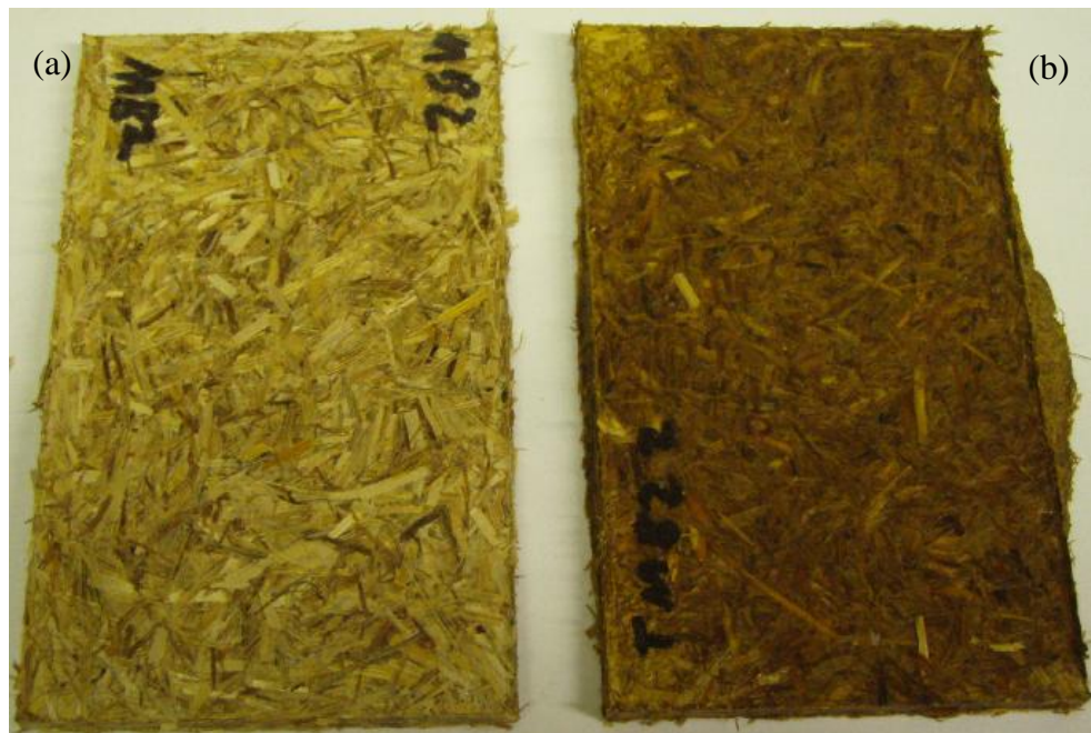
Figure 6.4: Comparison of the appearance of compression moulded straw boards showing the effect of leach-out phase in improved flow (by the flash in 6.4b) and inter-straw bonding. a) MB2 from straw without NaOH pre-treatment; b) TMB2 from straw with 6% NaOH pre-treatment.
