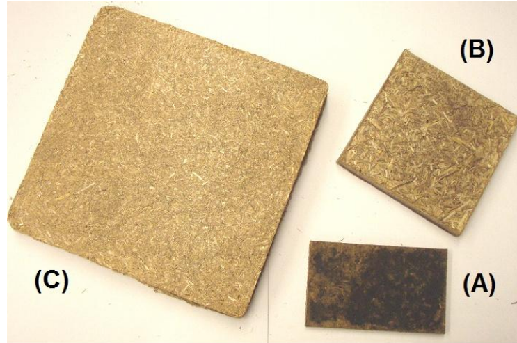
Figure 3.10: Straw boards of different dimensions: (A) 100x60x4mm; (B) 100x100x12mm; (C) 200x200x16mm
