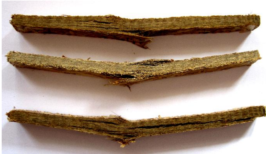
Figure 6.14: Fracture mode of MB2 at different stage post the peak stress showing typical initial delamination.
