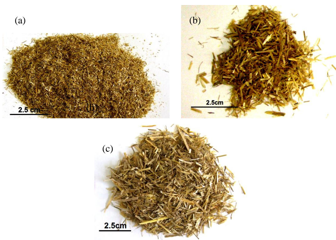
Figure 3.4: Morphology of graded straws prepared for straw boards (a) Short size straw; (b) Medium size straw; (c) Long size straw.
