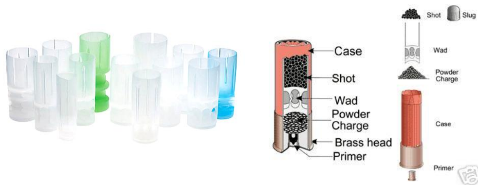
Figure 2.26: Plastic cartridge wads in shotgun (left) and their assembly position in a cartridge (right)
