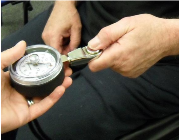
Figure 2.15: Standardised positioning for measurement of pinch force.
