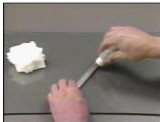
**Figure H.29: Flood the gagging area with conditioner.**
