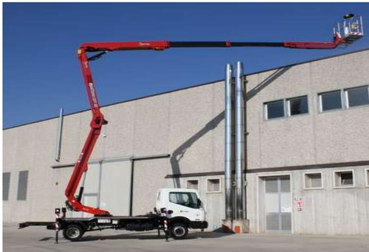
**Figure 2.19: Vehicle Mounted Access Platform [76]**
