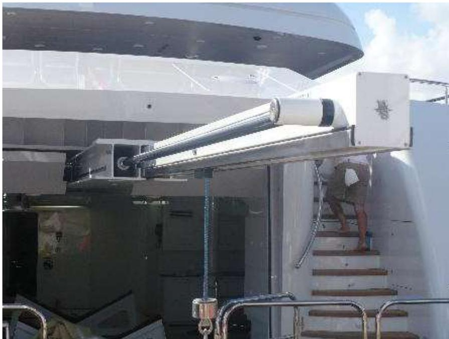
**Figure 2.26: The SL-DEX Type hydraulic overhead beam crane manufactured by Nautical Structures USA [78]**
