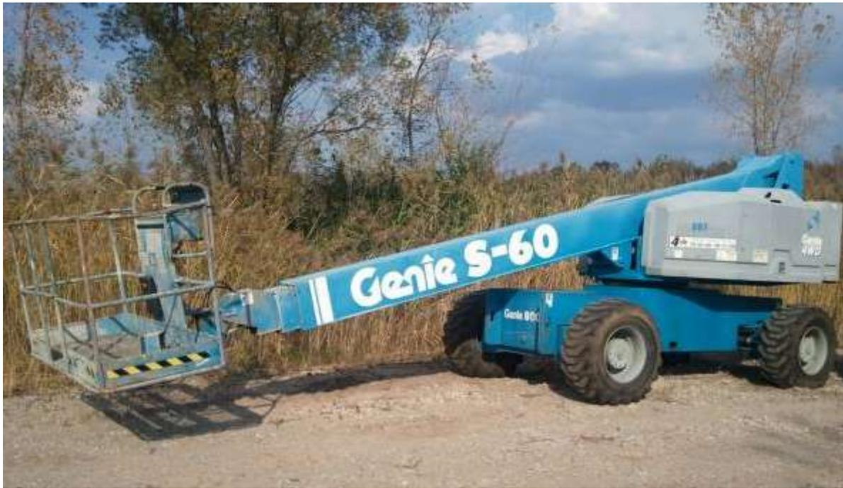
**Figure 2.15: Straight or “stick boom” access platform [74]**
