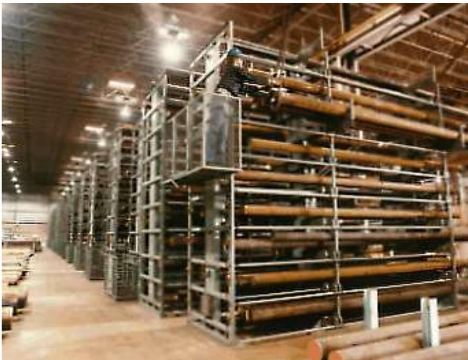
**Figure 2.38: '8 Tall SpaceSaver Rack' installed with optional electric lift cage. For maximum density '8Tall' models nearly six metres high are available [83]**
