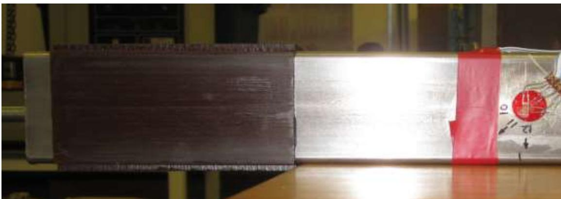
**Figure 8.4: Tufnell wear pads attached to beam 2. These four wear pads are located on the four walls of beam 2, at the end opposite to that where loads are applied**
