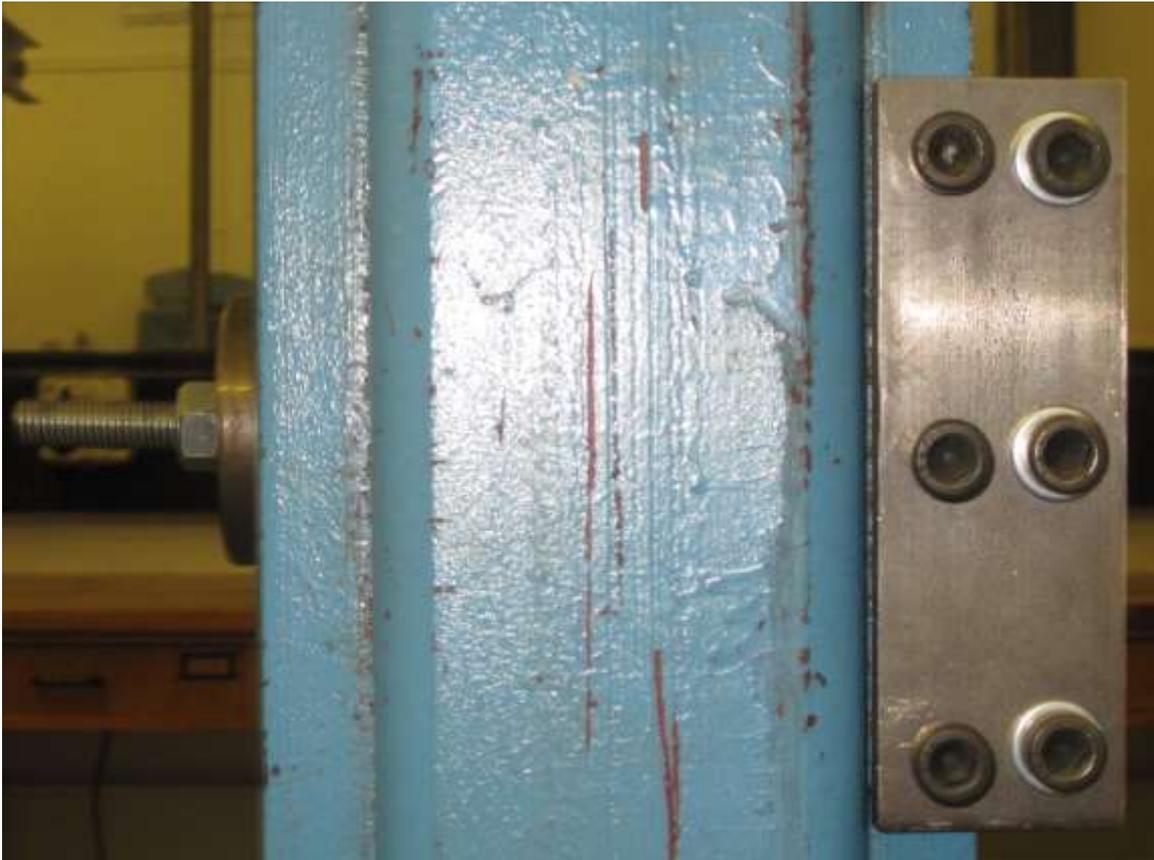
**Figure 8.12: Left hand view of the mounting jig showing the method by which the same is clamped to the support column.**
