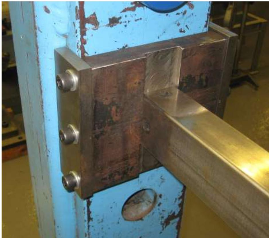
**Figure 8.9: Frontal view of the experimental mounting jig clamped to support column.**
