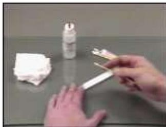
**Figure H.37: Replace the applicators when they become soiled. As before, continue scrubbing until the tip comes up clean.**
