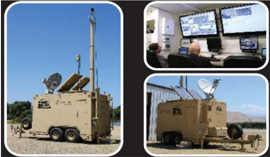
**Figure 2.34: A self contained US Tower manufactured Command, Control, Communications and Tactical Shelter or C3T Trailer [82]**
