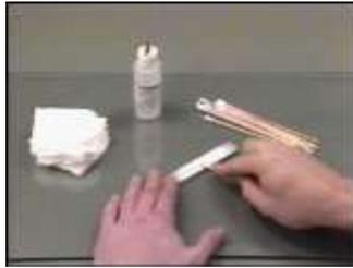
**Figure H.34: Use a liberal amount of acid conditioner to remove all graphite from the burnished layout line by scrubbing along the line with a cotton-tipped applicator.**
