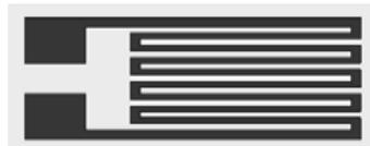
**Figure H.21: Uni-axial strain gauge [112]**
