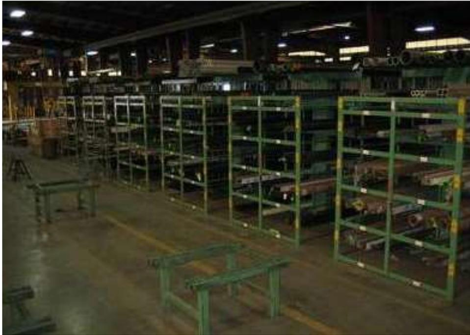
**Figure 2.39: ‘5 Tall SpaceSaver Rack’ storing 50-60 cm tubing at Marmon/Keystone. A rolling platform ladder is used to access the upper levels [84]**
