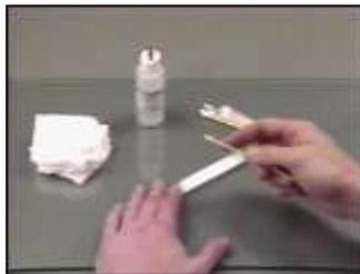
**Figure H.35: Keep scrubbing, but check the applicator tip for soiled appearance. Continue until the tip comes up clean.**
