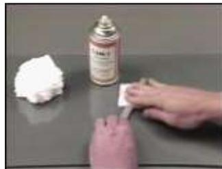
**Figure H.27: Wipe the specimen surface thoroughly with a gauze sponge.**
