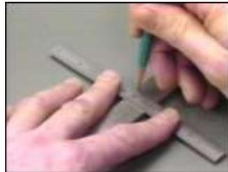
**Figure H.33: With a clean straight edge, and a 4H pencil firmly burnish a layout line.
