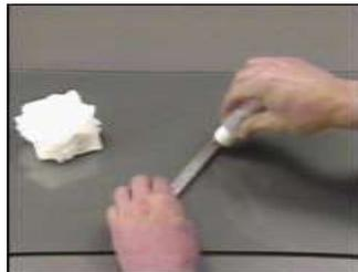
**Figure H.29: Flood the gagging area with conditioner.**
