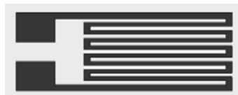
**Figure H.21: Uni-axial strain gauge [112]**
