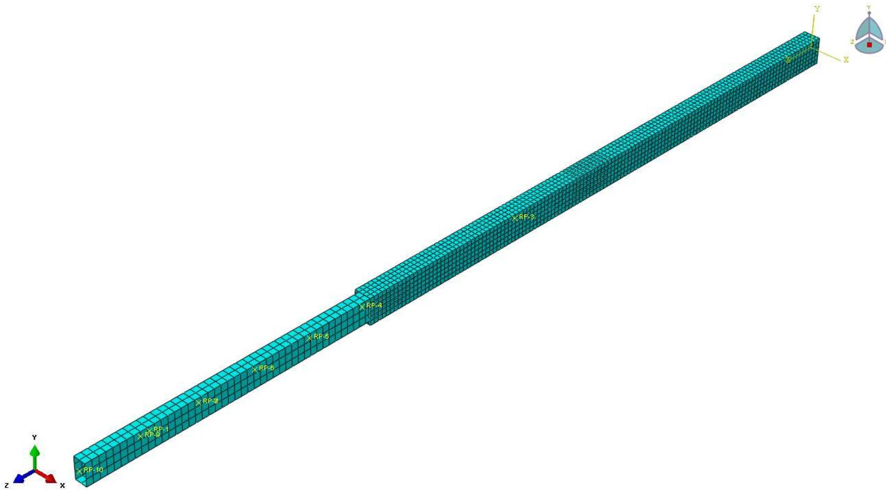
Figure G.33: Meshed telescopic beam assembly
