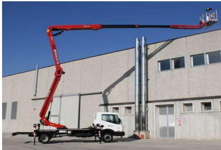
**Figure 2.19: Vehicle Mounted Access Platform [76]**
