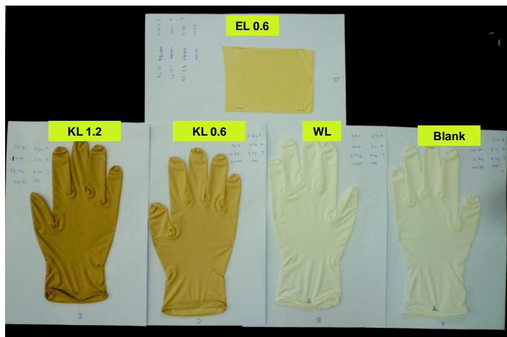
Figure 9.2 : Glove samples dipped from various compounds
