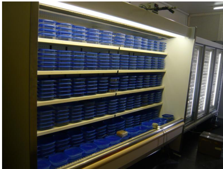
Figure 5.7 Photos of MT and LT multi-deck cabinets in the test chamber
