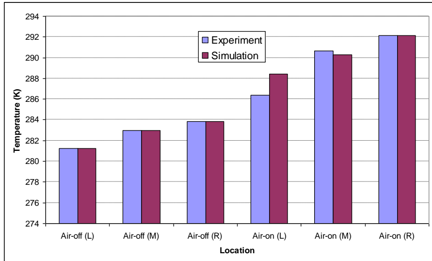
Figure 5.22 comparison of the air-off and air-on temperatures at the left, middle, and right sections of the cabinet
