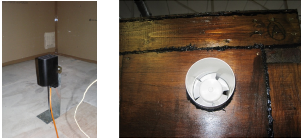
Figure 6.6 Test cell features. The heater Omega CS060 150W enclosure heater (left) and the XIL 100T Xpelair cell extract fan (right).
