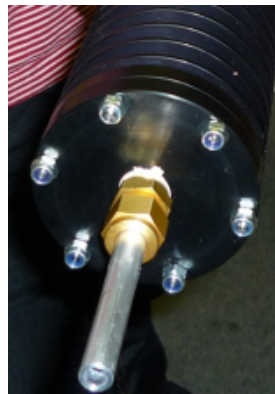
(ii) End cap screwed onto one finned tube end and the 3/8" Swagelok fitting screwed in with PTFE tape.
