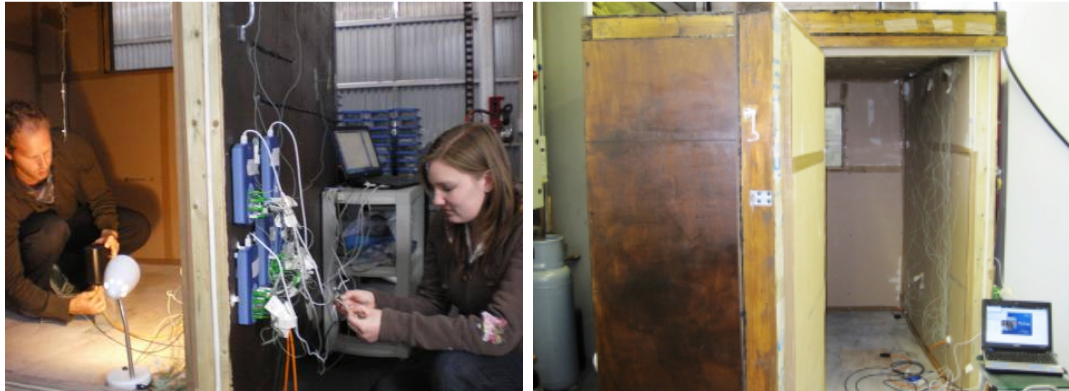
Figure 6.2 Images of the thermal test cell. The cell heater being checked whilst the externally located data loggers and thermocouples are labelled (left). The cell with its door open and laptop for data logging (right).
