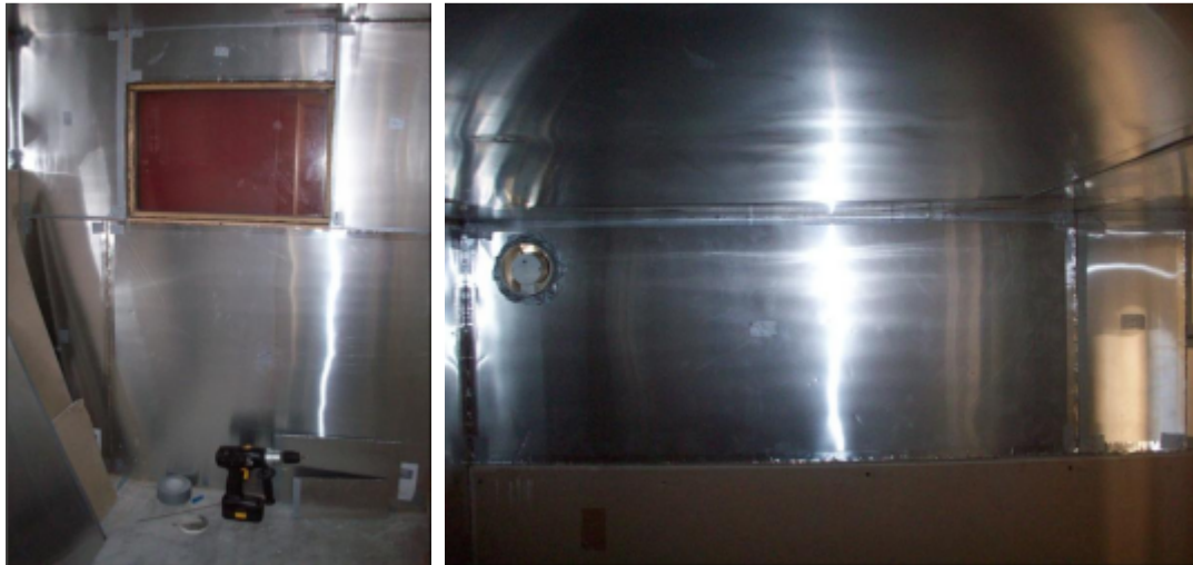
Figure 6.10 Energain panels applied to the internal surfaces of the test cell.
