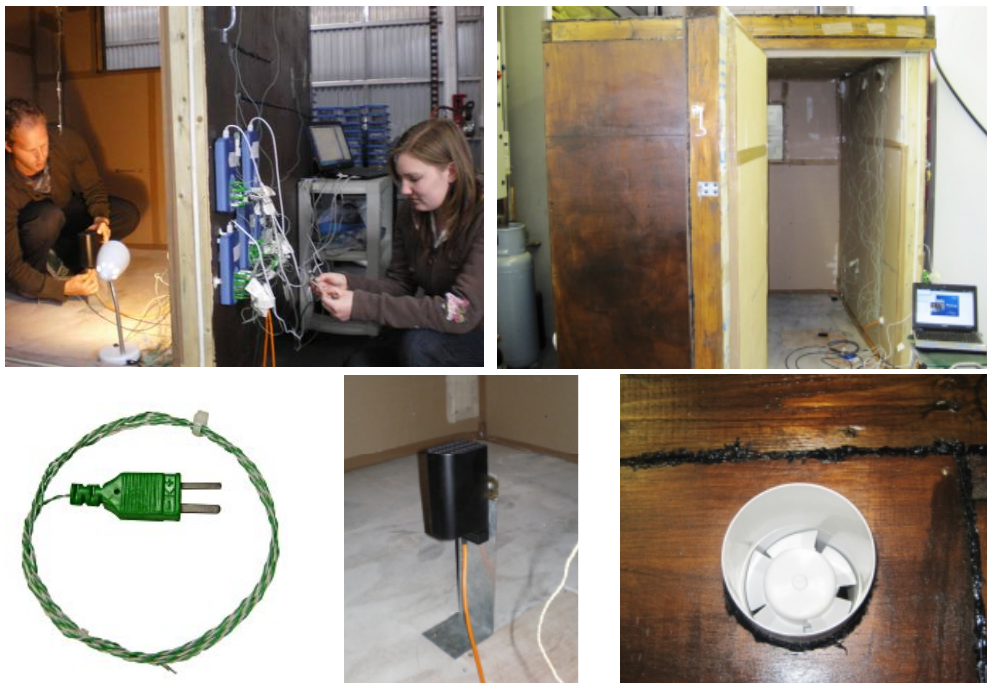
Figure ES.14 Test cell images. Heater and thermocouple connections being checked (top left). Test cell with door open and laptop for data logging (right). Example thermocouple (Pico technology, 2011) (bottom left). Heater, Omega CS060 150W (bottom centre). Extract fan, XIL 100T Xpelair (bottom right).
