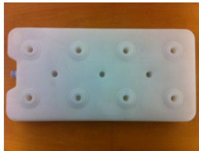
Figure 2.5 Macroencapsulated PCM. A PlusICE unit containing salt hydrate.
