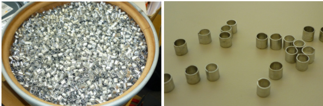
Figure 7.8 Raschig rings. Barrel of Raschig rings (left) and individual rings (right).
