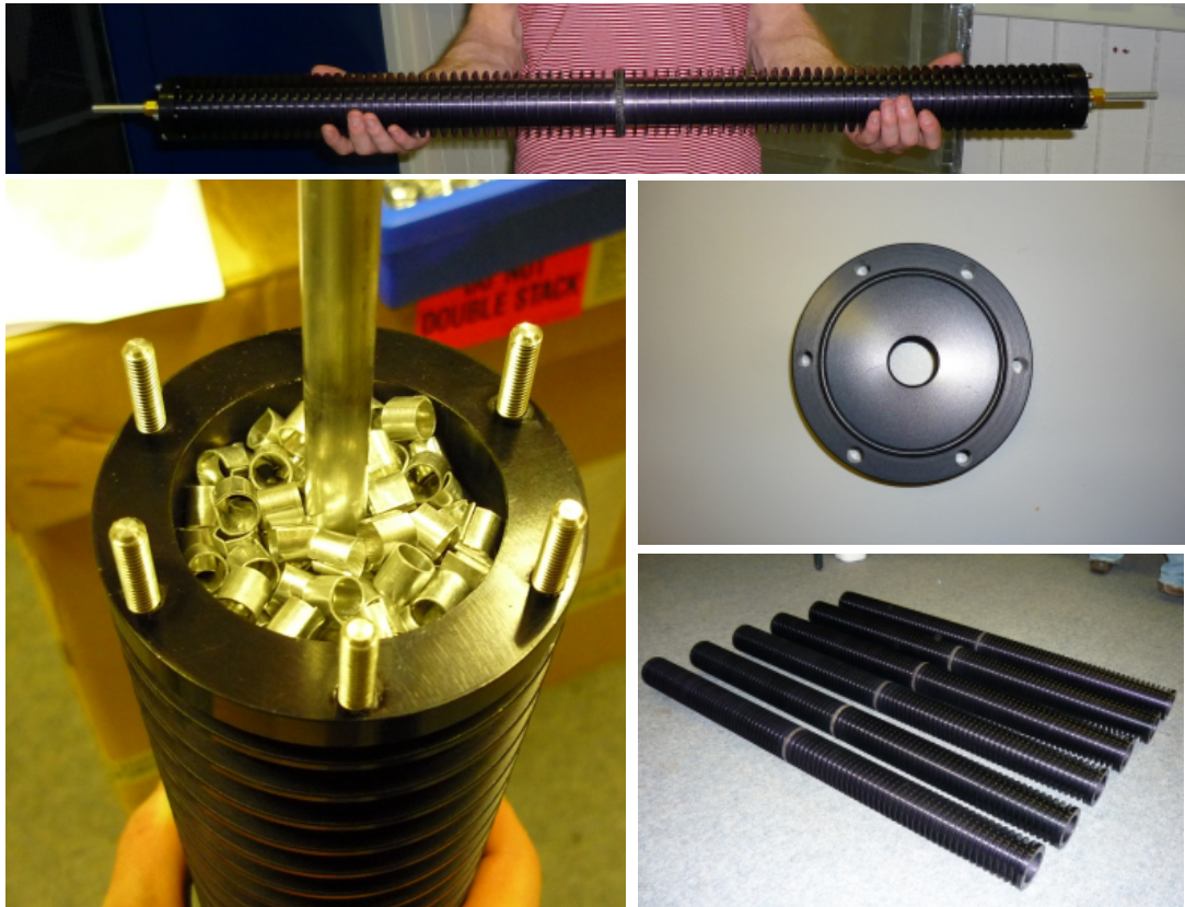
Figure ES.20 Images of the NewMass units. Completed unit (top), uncapped unit exposing Raschig rings and the chilled water pipe (left), cap with O-ring (upper right) and all finned tubes prior to assembly (bottom right).
