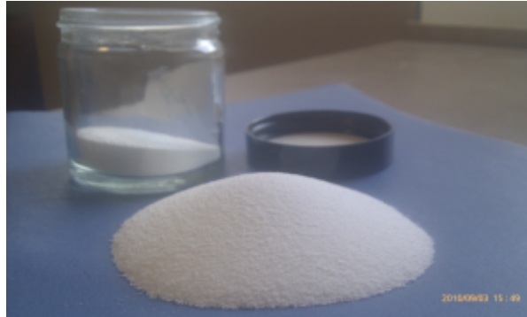
Figure 2.6 Microencapsulated PCM. BASF micronal powder (Oyeleke, 2010).
