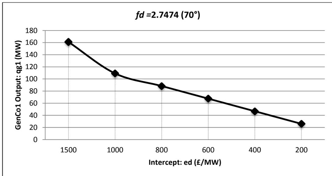
Figure 4.12: Impact of Inverse Demand Curve Intercept on GenCo1 Output ( $f_d=70^\circ$ )
