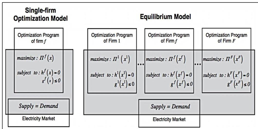
Figure 2.12: Differences between Optimization Model and Equilibrium Model [32]
