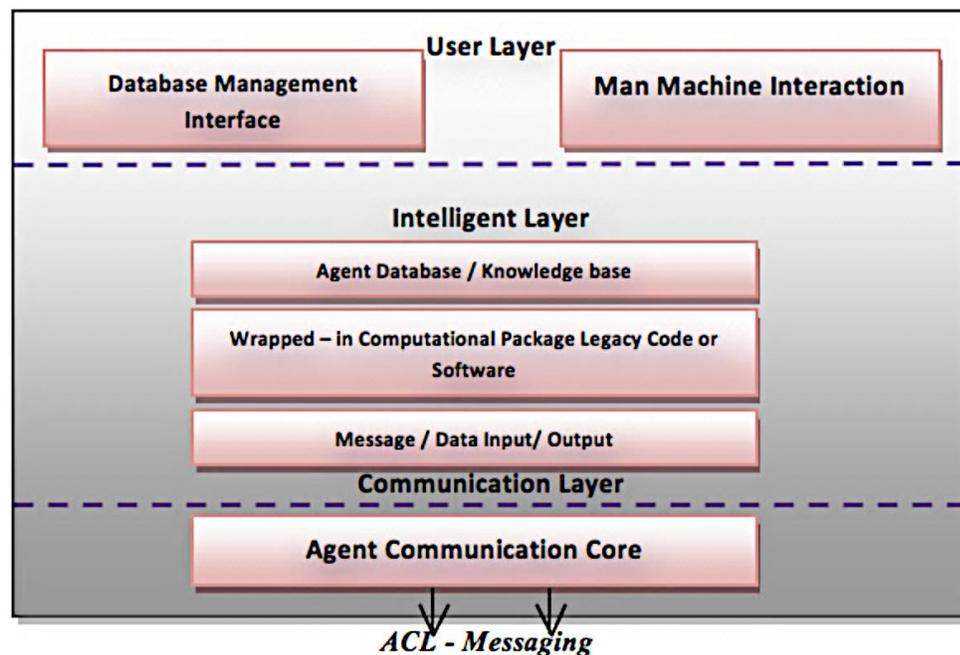
Figure 2.11: Layered Structure of an Agent
