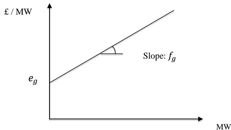
Figure 5.3: Initial Inverse Generation Curve
