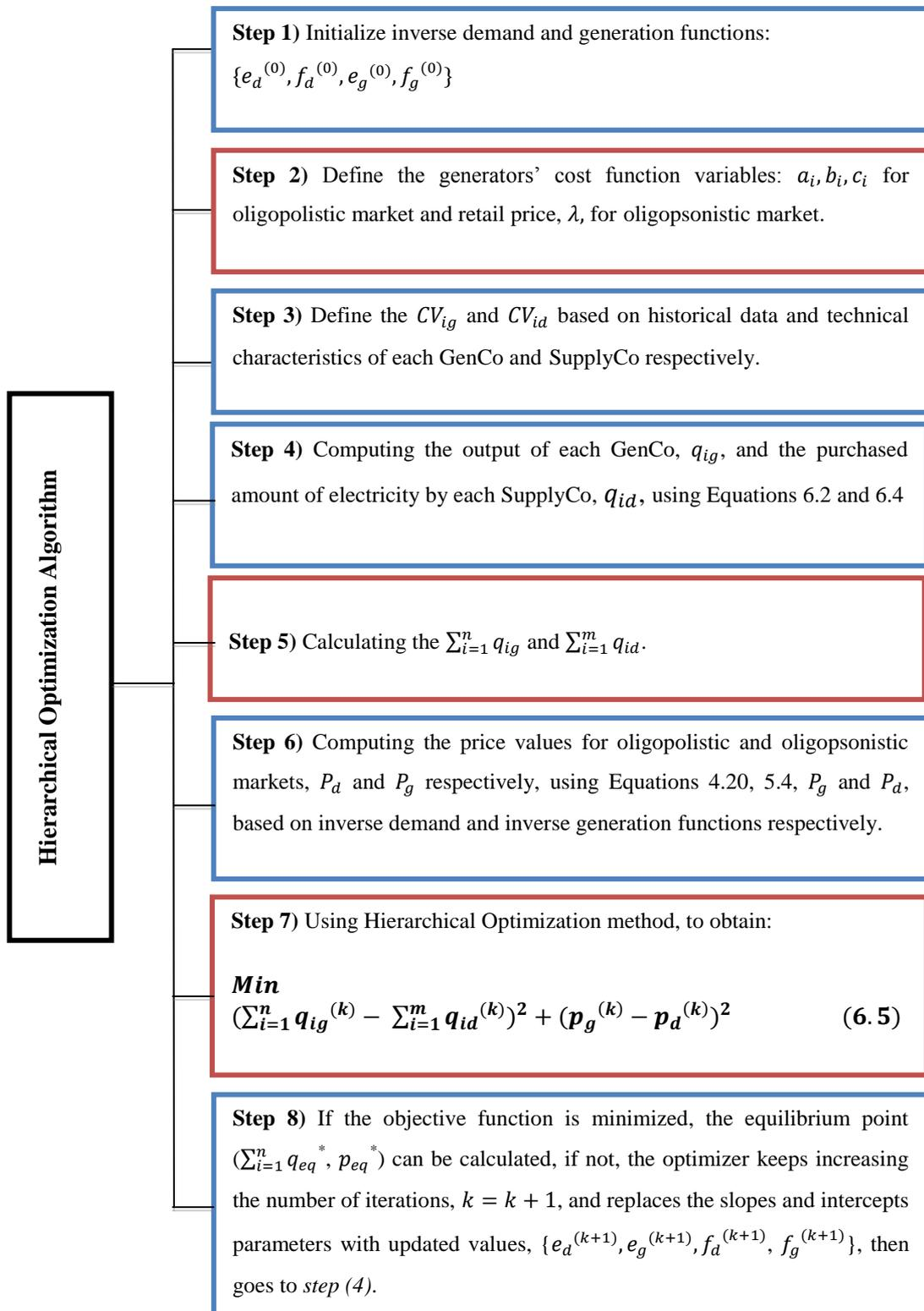
Figure 6.4: Hierarchical Optimization Algorithm
