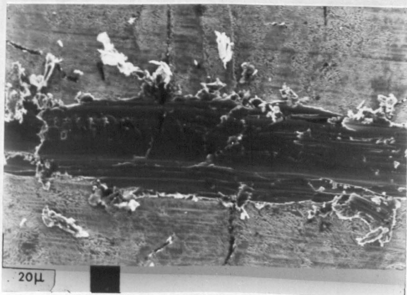
Fig. 60 Grey cast Iron fragmentation, diamond indenter at 60 attack angle.
