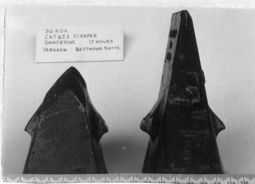
Fig. 16 New and worn digger teeth after less than 20 working hours.
