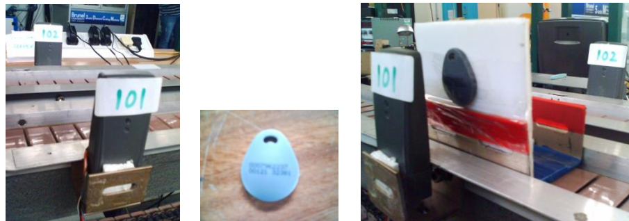
Figure 8-10 Proximity RFID reader and its associated passive tag
