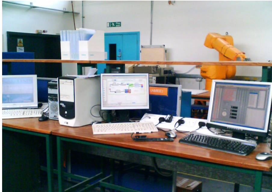
Figure 8-16 view of three PC machines for - from left to right - OPC server system, simulation system, and DAQ system
