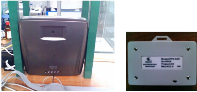
Figure 8-11 Range RFID reader and its associated active tag
