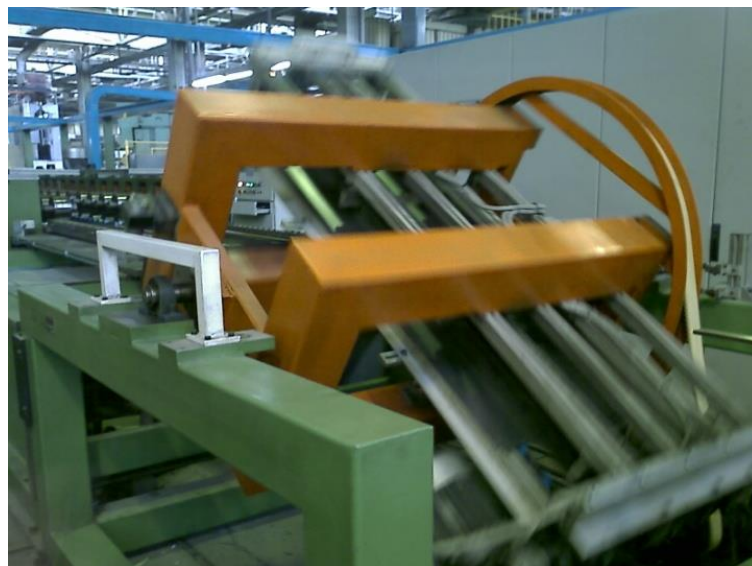
Figure 9-6 GR-3A or tilter machine
