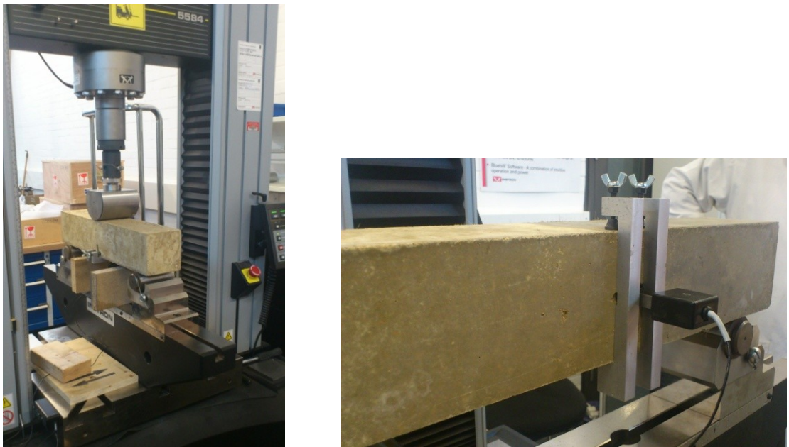
Figure 3.5—Fracture test setup with Instron hydraulic machine and a bend fixture
