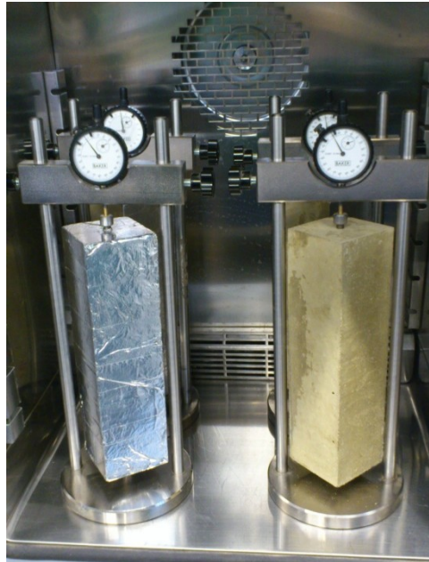
Figure 6.3—Concrete prisms for free shrinkage test placed in the environmental chamber
