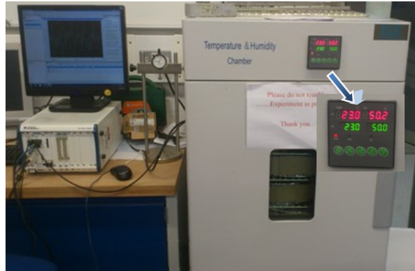
Figure 4.6—Ring specimens connected to the data logger and under testing in environmental chamber
