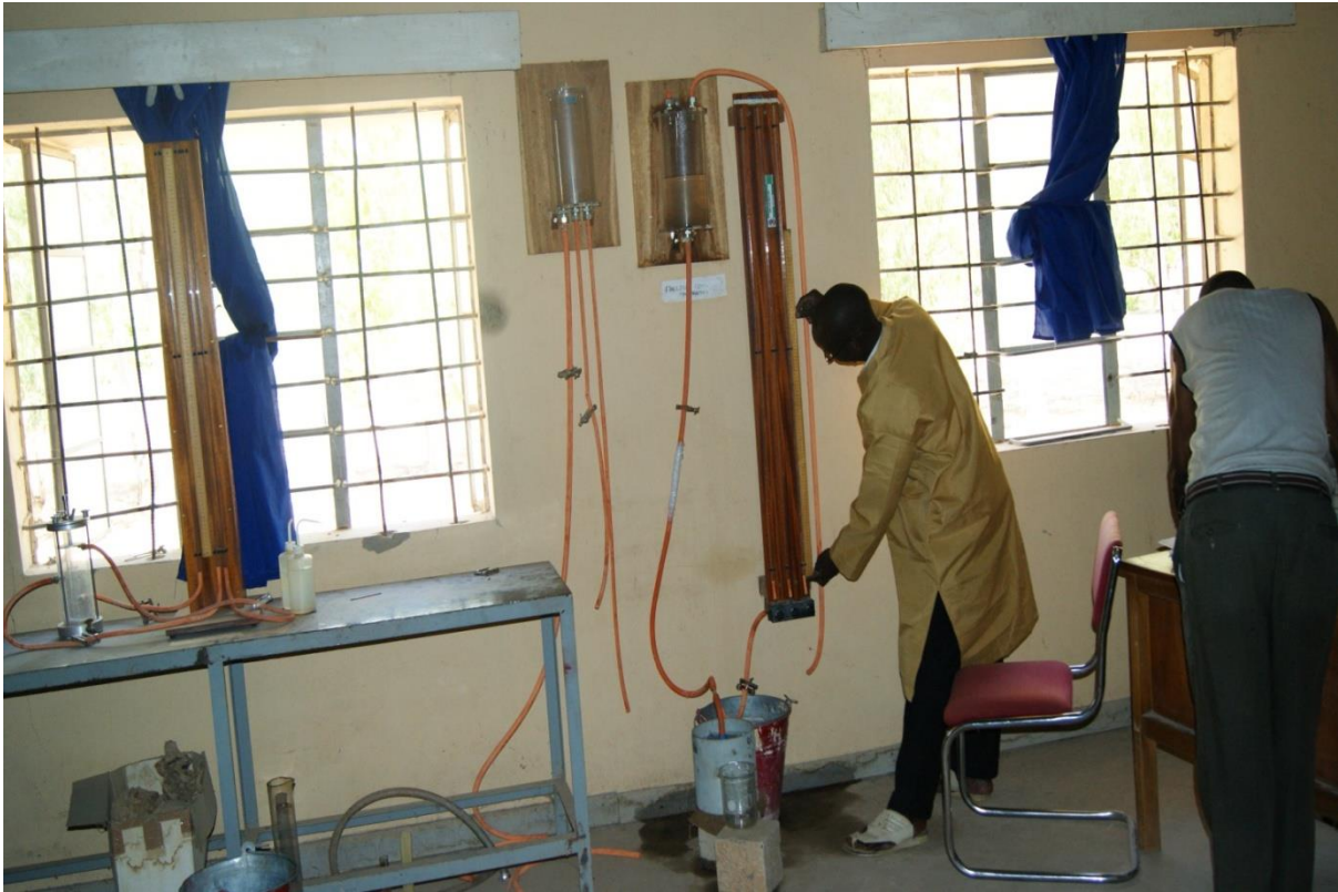
Figure 3.11: Taking reading for laboratory permeability test using falling head permeameter (The photograph taken by Garba on 20 th May 2011).
