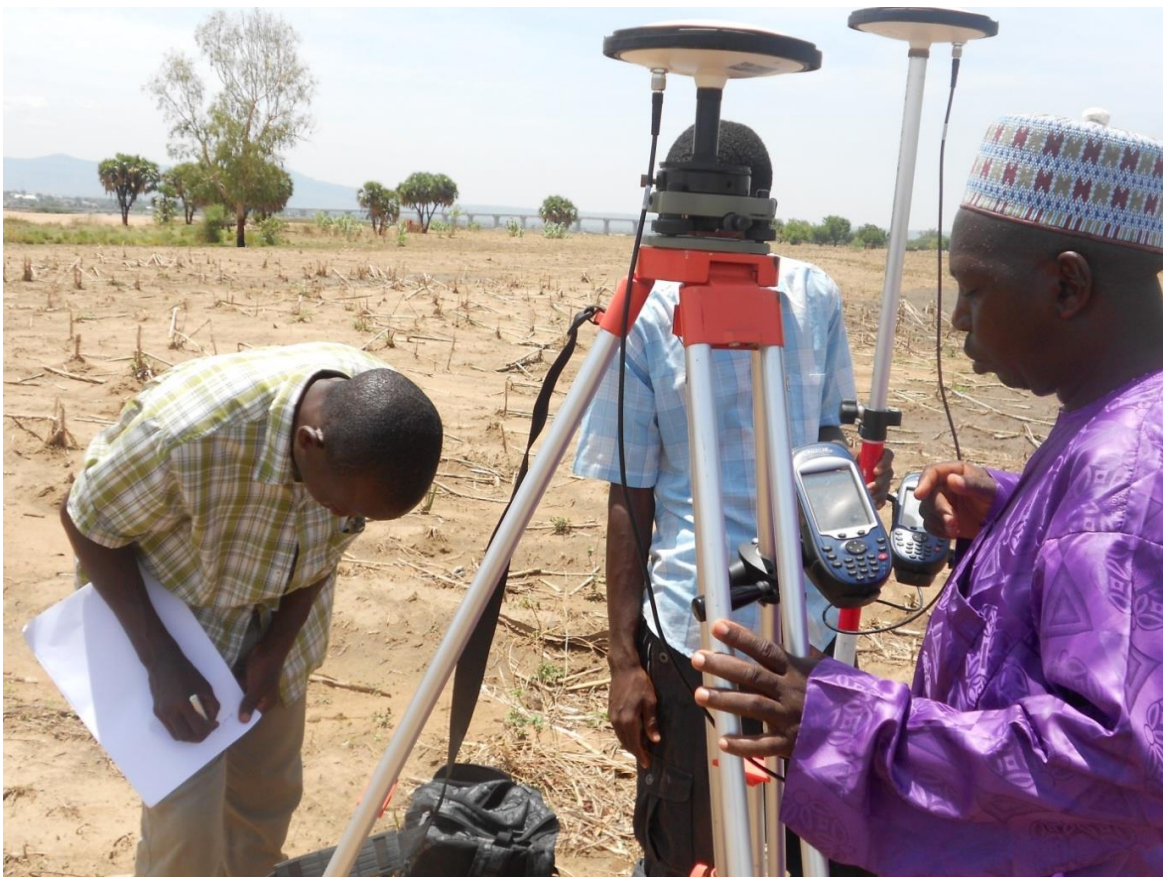
Figure 3.1: A ProMark3 Global Positioning System instrument for determining the height elevation across the floodplain at borehole location 1 transects 1 (see Figure 2.8) (the photograph taken by Mohammed Abana Girei on 13 th April 2012).
