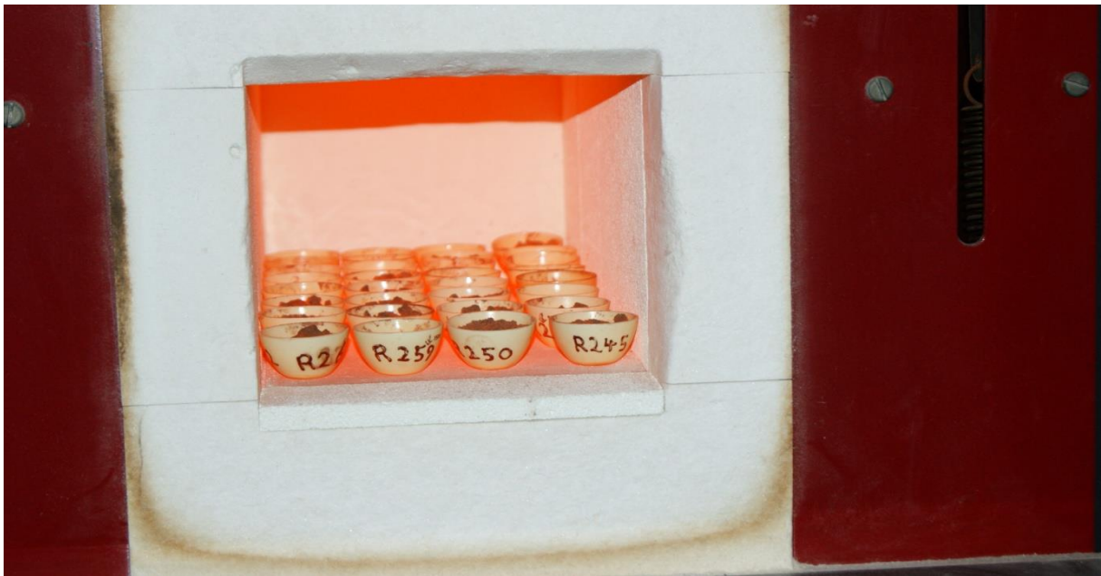
Figure 3.7: Crucibles with samples heated in a muffle furnace for the determination of loss on ignition for the sediment samples (The photograph taken by the author on 2 nd September 2011).
