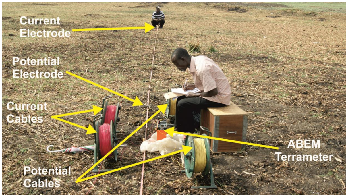
Figure 3.10: Taking resistivity sounding readings in the field with the ABEM Terrameter equipment at borehole location 8 transects 4 (see Figure 2.8) (The photograph taken by Mohammed Girei on 10 th April 2011).
