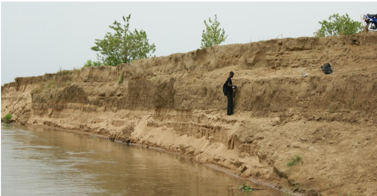
Figure 3.2: Sampling sediment using a plastic trowel along River Benue Valley Bank, Yola outcrops at sampling location G along transect 3 (see Figure 2.28) (The photograph taken by Mohammed Abana Girei on 19 th April 2011).
