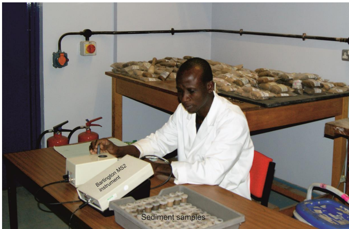
Figure 3.8: Taking reading for magnetic susceptibility in the laboratory with the Bartington MS2 instrument (The photograph taken by Nik Nik on 10 th August 2011).
