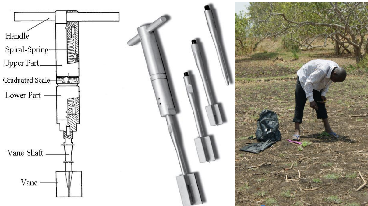
Figure 2.24: A Geonor H-60 Field Shear Vane Tester, 3 Vanes and pointer and determining shear strength on sediments (Geonor, 2005; Eijkelkamp, 2009).
