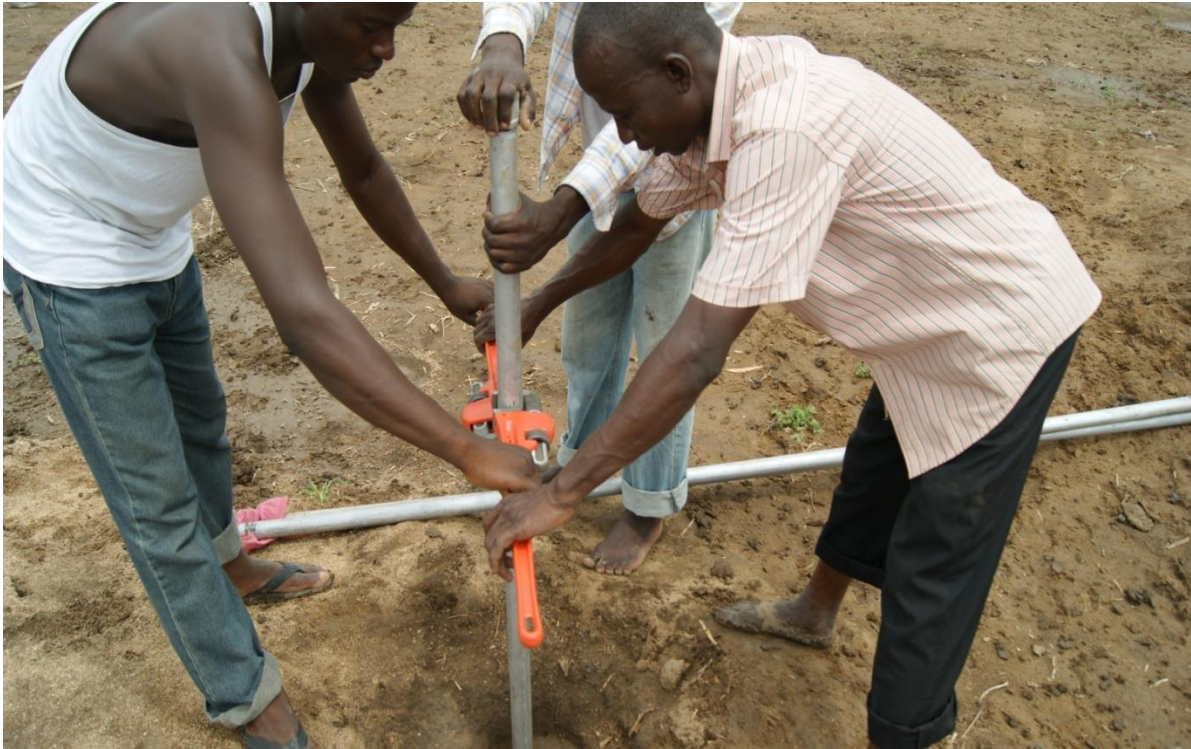
Figure 3.3: Borehole drilling using hand augering method for sediment sampling in the floodplain at borehole location 4 transect 2 (see Figure 2.8) (The photograph taken by Mohammed Abana Girei on 4 th May 2011).
