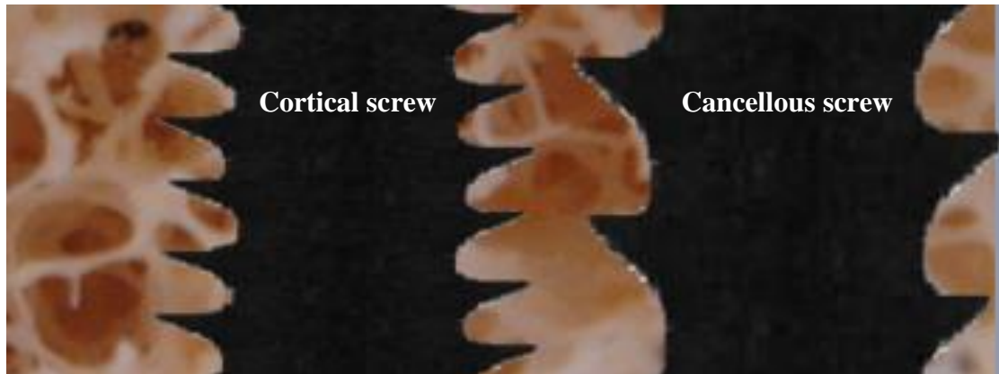
Figure 2.13: Which one would have the best pull-out force? Smaller or bigger threads pitch (Philip Procter, Stryker Osteosynthesis)
