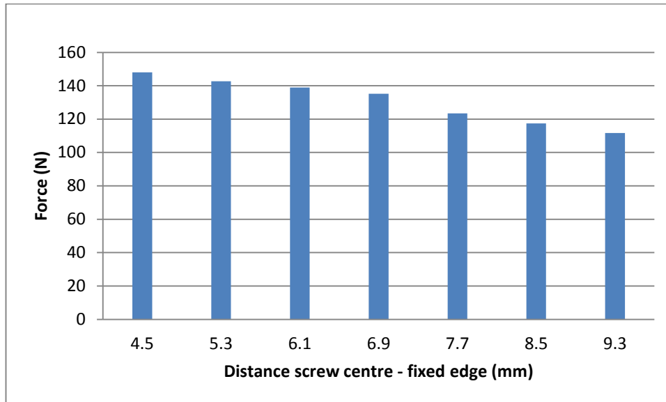
Figure 3.6: Force reaction at 0.3mm screw vertical displacement by distance to fixed edge
