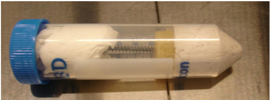
Figure 5.5: Bone sample with screw inserted positioned along the tube axis with tissues
