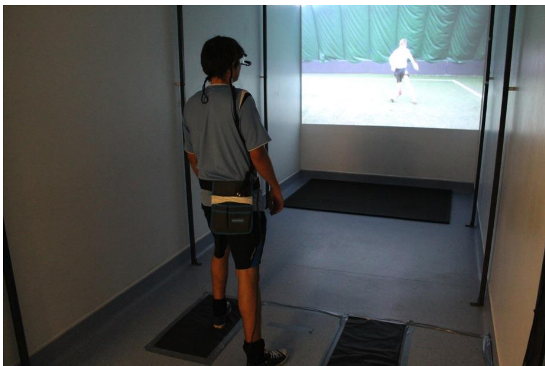
Figure 5.2. The experimental setup, with eye-tracking, and the perceptual-cognitive soccer representative task simulation.
