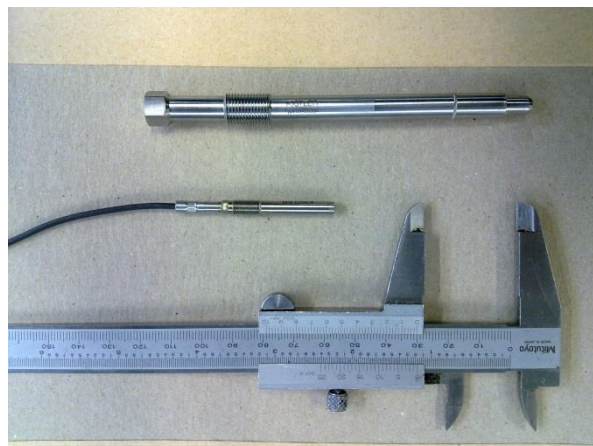
Figure A.5: Kistler pressure transducer and glow plug adapter
