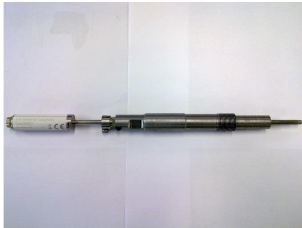
Figure A.7: Kistler 2629C1 TDC sensor with adapter.
