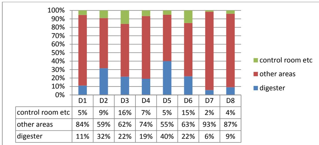
Figure 4.4. Area requirements for eight anaerobic digesters in Cyprus (D1-D6 are completely mixed, D7 and D8 are anaerobic lagoons)
