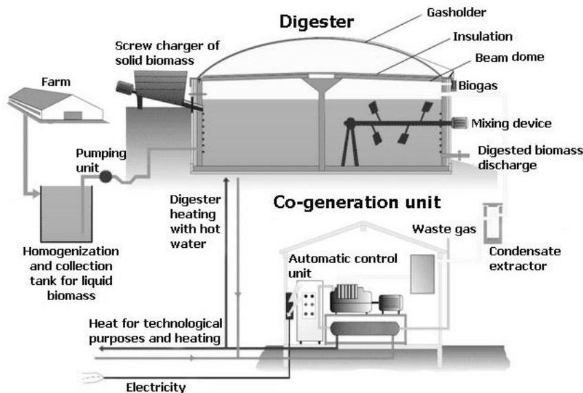
Figure 4.2. Stages of AD, with energy production from the biogas produced (Zorg Biogas, 2010)
