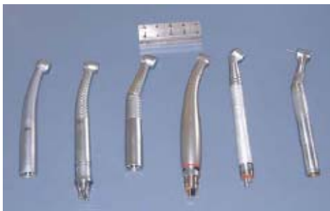
Figure 1 Drill handpieces tested together with the steel bar with holes in which the burr was placed during tests.
