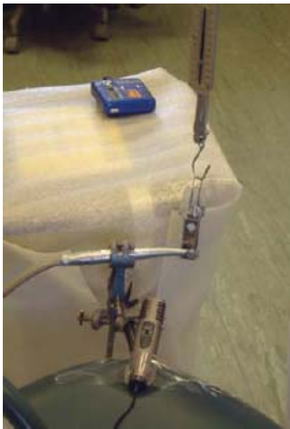
Figure 4: Handpiece under load
